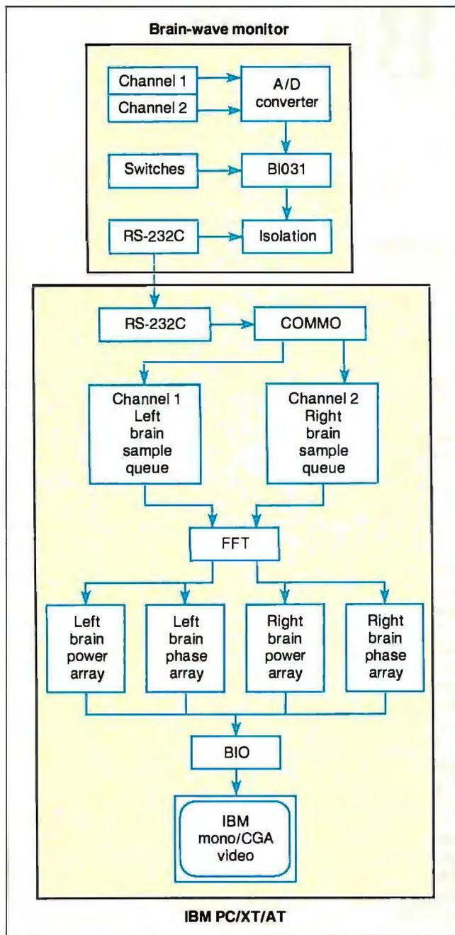
**Figure 1:** A block diagram of the complete HAL system, showing major components of the brain-wave monitor and the host machine.
