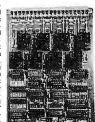
The BCC40R can be directly controlled from BASIC or it can function completely in the background under an application program using high speed interrupt-driven ROM C firmware. This firmware sets aside a table in memory which reflects the status and setpoints of the relays. Interaction among programs within a multiboard BCC40x system merely consists of reading or setting these memory table values.
