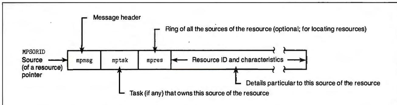
Figure 6: Internal representation of a source (of a resource) data type.
