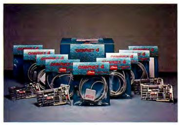
The Omninet/4 Networking Kit includes four transporter cards, four workstation kits, three trunk cable kits, one termination kit, one software kit and one installation guide.
