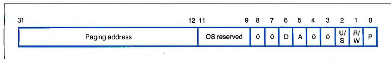
**Figure A:** Page-directory entry and page-table entry layout. PDEs and PTEs are almost identical, but a PDE points to a page table, while a PTE points to a page.
