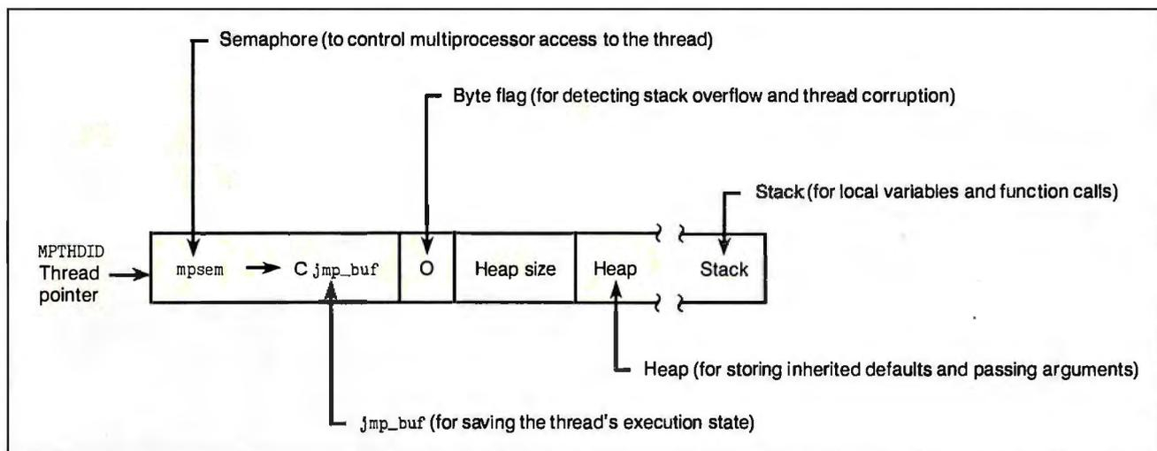
**Figure 2:** Internal representation of the thread data type.
