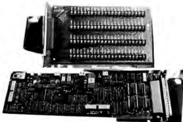
**IBM PC\* DATA ACQUISITION AND CONTROL ADAPTER & DISTRIBUTION PANEL** provides the capability to control and monitor processes within a sensor base system.
