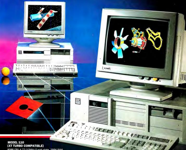
8088 CPU,4.77/10MHz 0 wait state, 256K RAM upgradable to 640K, 360K floppy and floppy controller, 101 enhanced keyboard, 150W power supply and FCC approved.
