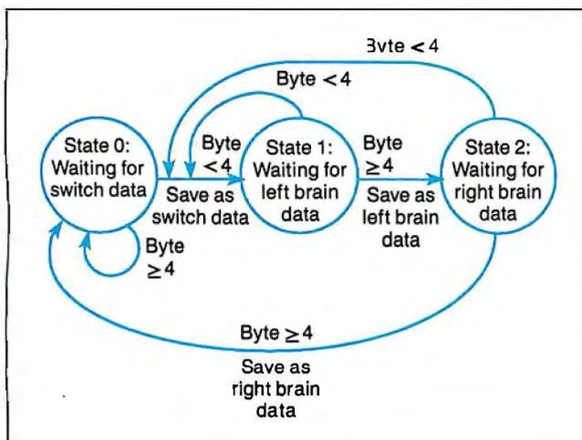
Figure 3: The host computer's receiver routine executes a finite-state machine, shown here graphically. Each circular node of the graph represents a state, and transitions from state to state occur when the system receives a byte.
