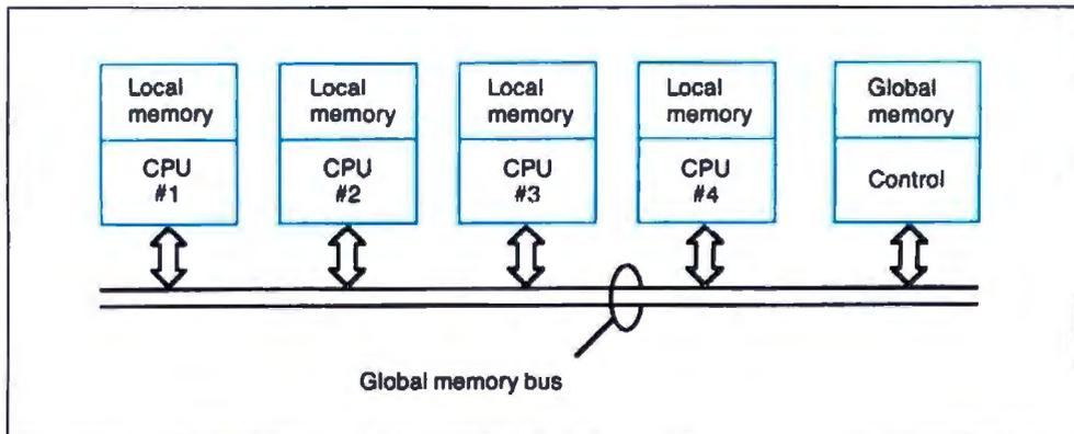
**Figure 13:** A four-way direct-connected multiprocessor system.
