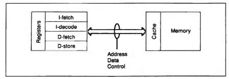
Figure 8: In a final attempt to improve throughput, pipelining is added to the CPU.
