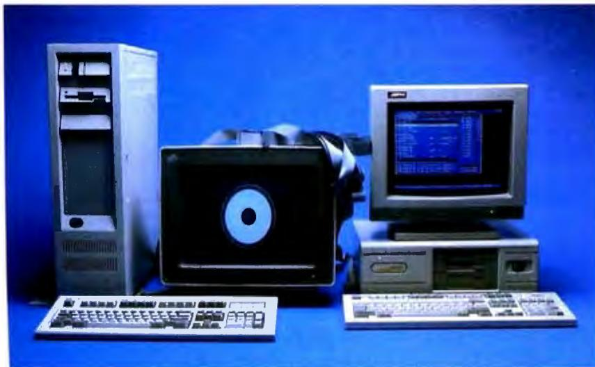
**Photo 3:** Remote debugging with Turbo Debugger. The machine on the left is executing the BYTE low-level graphics benchmark program, controlled via a serial connection with the machine on the right running the debugger.
