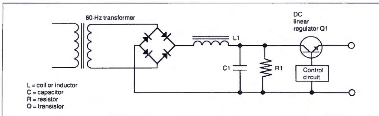
**Figure 1:** Linear power supplies, used in small computers up until a few years ago, featured a large 60-Hz power transformer connected across the input. Such power supplies were sensitive to variations in voltage and made power supplies bulky.
