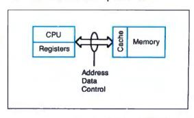
Figure 6: The modified system from figure 3 is further modified by adding a cache between the CPU and memory.
