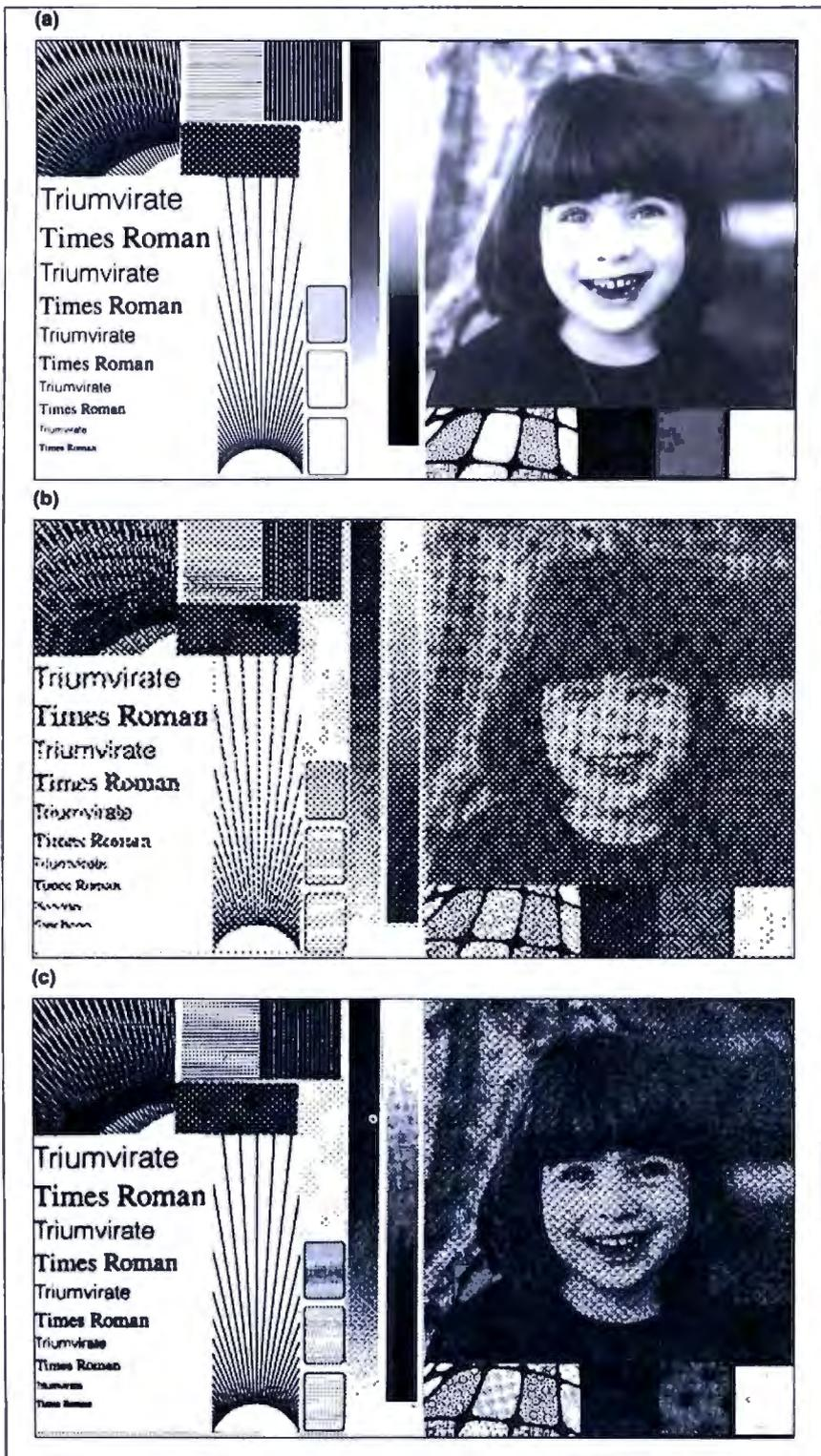
**Figure 1:** (a) *BYTE's* test pattern for scanner quality. (b) *The test pattern scanned at 150 dpi. The Microtek scanner was adjusted for halftone scanning to accommodate the halftone image. When the scanner was adjusted for line art, the lines and patterns looked considerably better, but the halftone's quality suffered.* (c) *The test pattern scanned at 300 dpi, halftone setting. Notice the improvement in the lines and patterns as well as in the halftone image. All images are actual size.*
