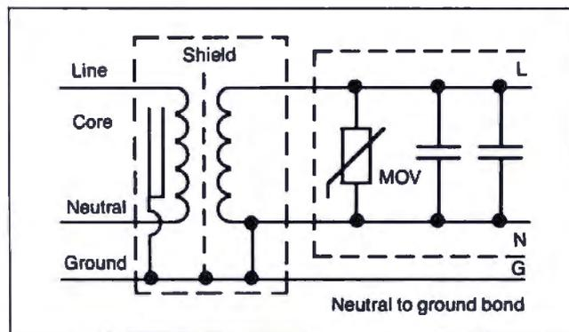
**Figure 7:** A power-line conditioner contains an isolation transformer with secondary surge suppression and the neutral and ground bonded.
