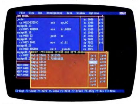
Photo 2: Turbo Debugger's numeric coprocessor window lets you dive into your system's floating-point unit (in this case, an 80387). Notice that you can enter numbers directly into the coprocessor's registers.
