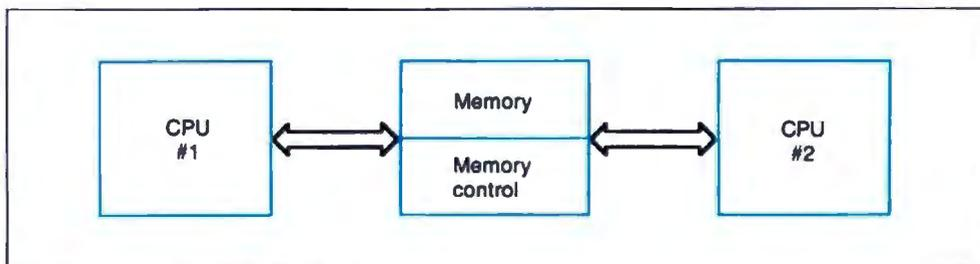
**Figure 11:** Both CPUs of the system described in figure 10 execute ADD instructions. ▼
