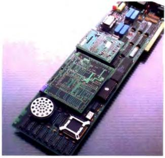
Connection Coprocessor multitasking board from Intel.
