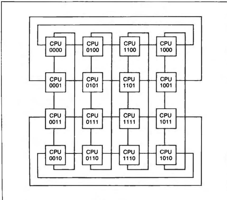
Figure 16: The processors from figure 15 are each assigned an ID number to simplify message passing.
