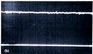
Photo 2: These photos show noise in an electrical circuit, (a) before and (b) after insertion of a power-line conditioner. In both photos, the top trace is normal-mode noise and the bottom trace is common-mode noise.
