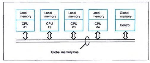
Figure 13: A four-way direct-connected multiprocessor system.
