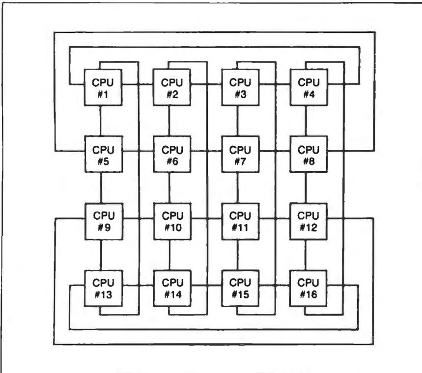
Figure 15: A 16-processor system. Each processor can communicate with its four closest neighbors.
