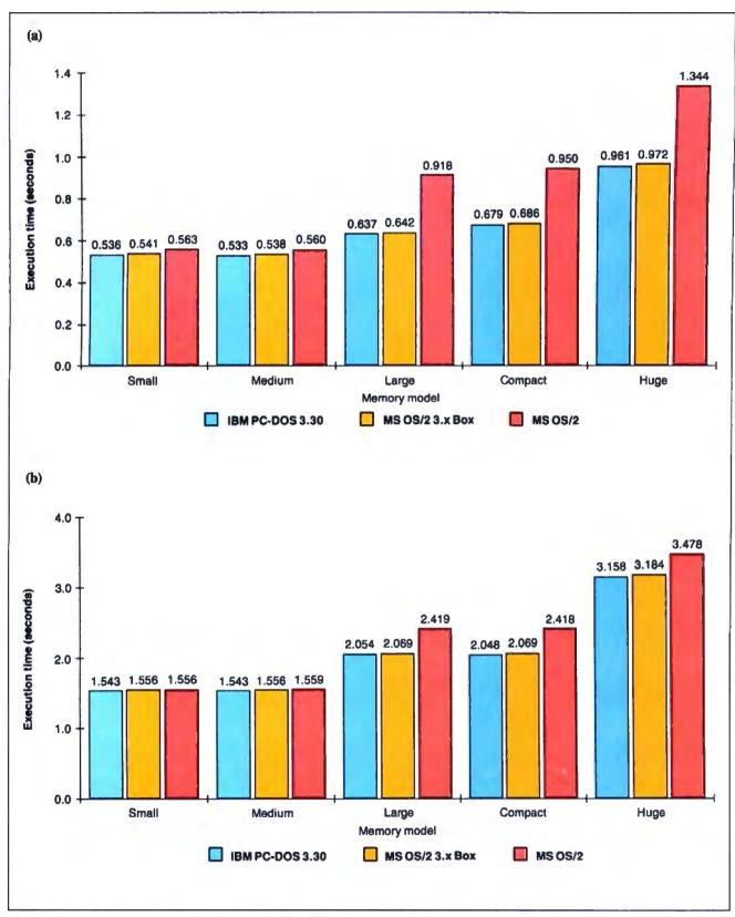
Figure 1: According to my tests with small memory models, the Sieve of Eratosthenes took somewhat longer to run in the compatibility box and in OS/2 protected mode than in DOS. Using larger memory models, however, OS/2 took as much as 44 percent longer on a 16-MHz Trillian Power Systems 386 (a), and 18 percent longer on an 8-MHz IBM PC AT (b).
