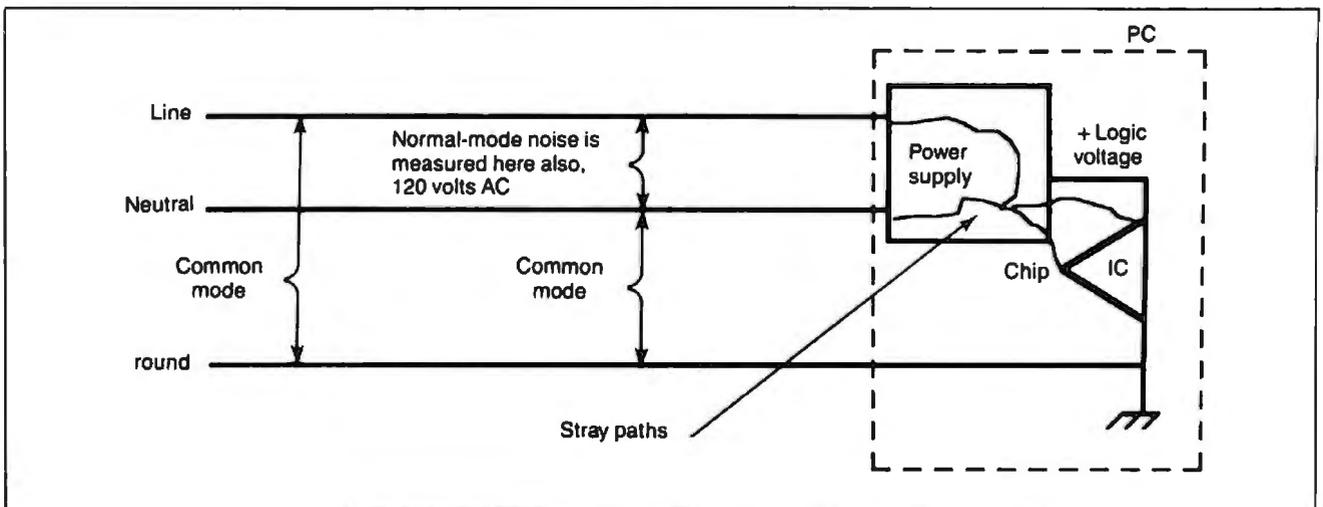
**Figure 3:** Normal-mode noise appears as voltage between the line and neutral wires in a circuit. Common-mode noise appears between the neutral and ground wires. If common-mode noise can find a stray path (and it will, especially through a switching power supply), it will appear across the chip from one of its pins and the logic ground pin. Normal-mode noise appears across the power supply just like utility power.
