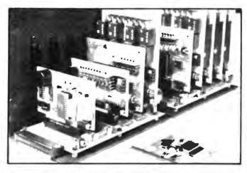
An A-BUS system with two Motherboards
