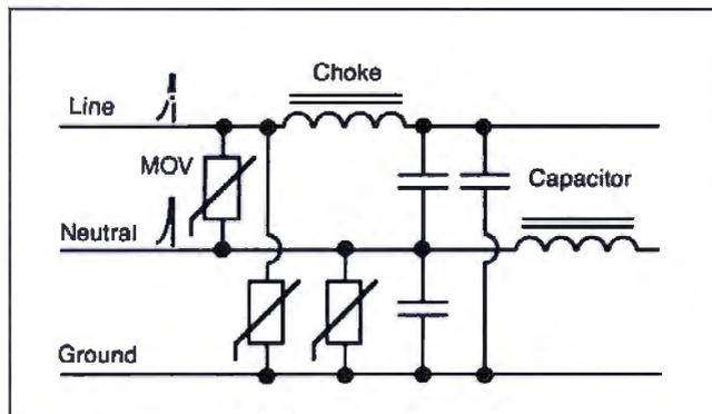
**Figure 6:** Typical circuit of a surge suppressor. Most simple surge strips have only a MOV (metal oxide varistor) and capacitors from line to neutral.
