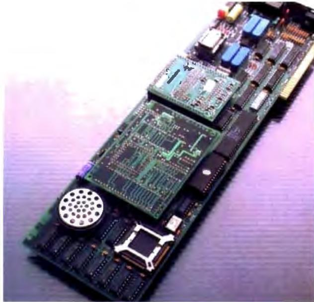
Connection Coprocessor multitasking board from Intel.
