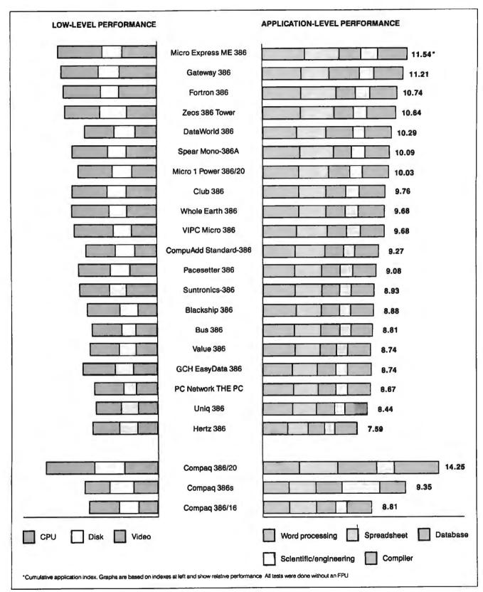
Figure 1: The Micro Express ME 386 and the Gateway 386, with 20-MHz 80386s, finished tops. Of systems with 16-MHz 80386s, the Zeos 386 Tower and the DataWorld 386 are on top. Fourteen systems finished higher on the benchmarks than a 16-MHz Compaq Deskpro. Compared to the Compaq 386s, all had a higher CPU index, and half had a higher application index.
