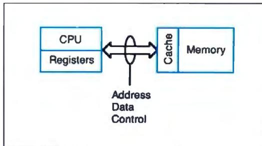
**Figure 6:** The modified system from figure 3 is further modified by adding a cache between the CPU and memory.
