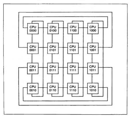
Figure 16: The processors from figure 15 are each assigned an 1D number to simplify message passing.
