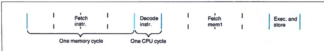
**Figure 5:** *Doubling the CPU clock speed for the instruction shown in figure 4 yields this sequence. Since the CPU is running twice as fast, memory access now requires four cycles.*
