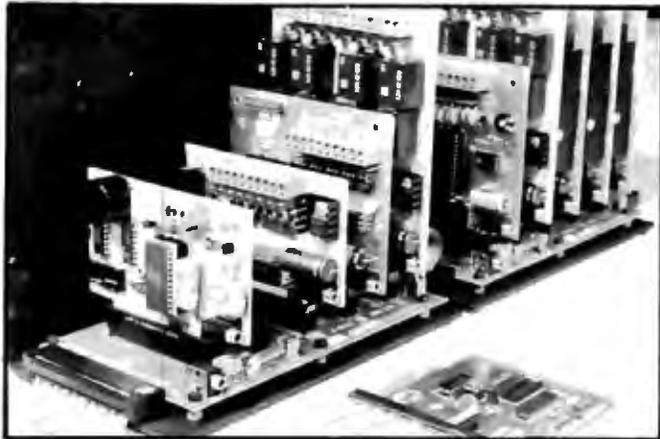
An A-BUS system with two Motherboards
