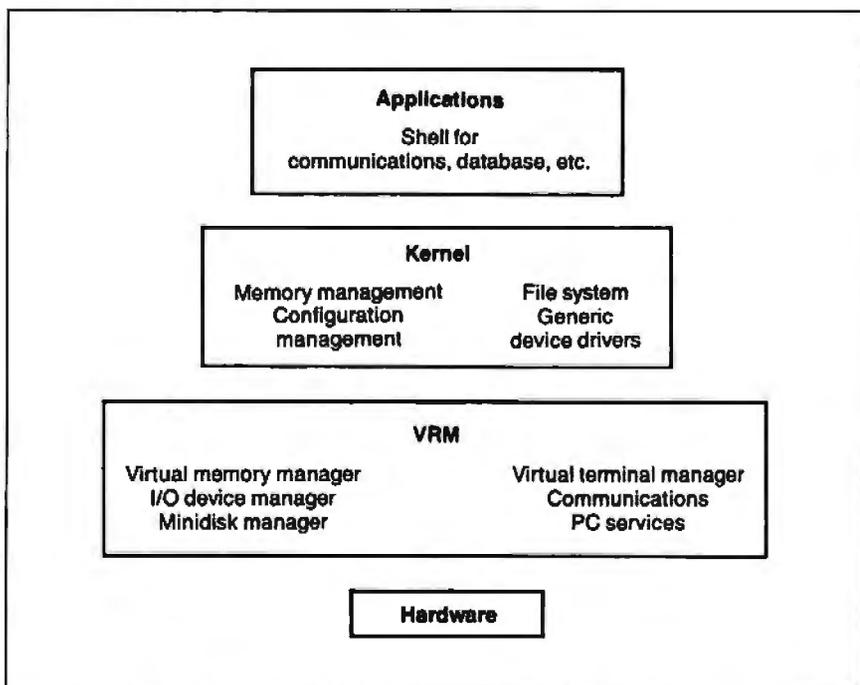
**Figure 1:** AIX's Virtual Resource Manager (VRM) hides the complexities of the hardware from the operating system software.
