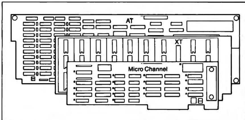
Figure 1: The MCA card is smaller in area than either the XT or AT cards.
