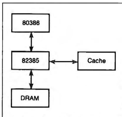
*The Intel 82385 cache controller lets the 80386 run out of a small high-speed cache whenever possible; it accesses slower DRAM only when the memory the 80386 needs is not in the cache.*
