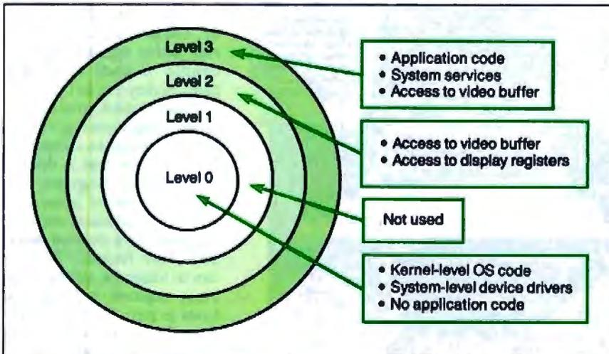
**Figure 1:** The 80286 protected-mode architecture allows OS/2 to partition its running environment into privilege levels, which specify the access to system services and hardware registers. A similar drawing of real-mode DOS programming would show only one circle.
