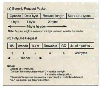
Figure 3: X Protocol request packets contain a 4-byte header and as many additional bytes as needed to communicate the request. The PolyLine request contains the information to draw a series of lines with a given line style and thickness within the graphics context.
