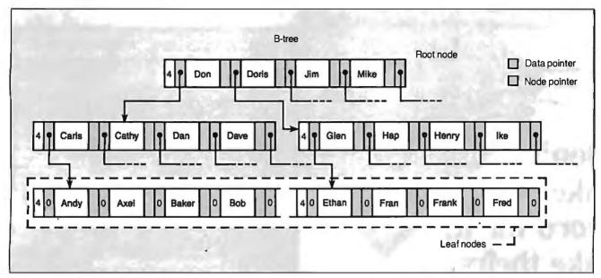
Figure 3: A B-tree of order 4. Now, each node holds multiple keys. (Note the dashed-line key pointers leading to nodes not shown.)
