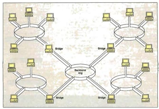
Figure 9: A backbone ring consists of a series of bridges in a ring, each connecting a peripheral ring to the backbone.
