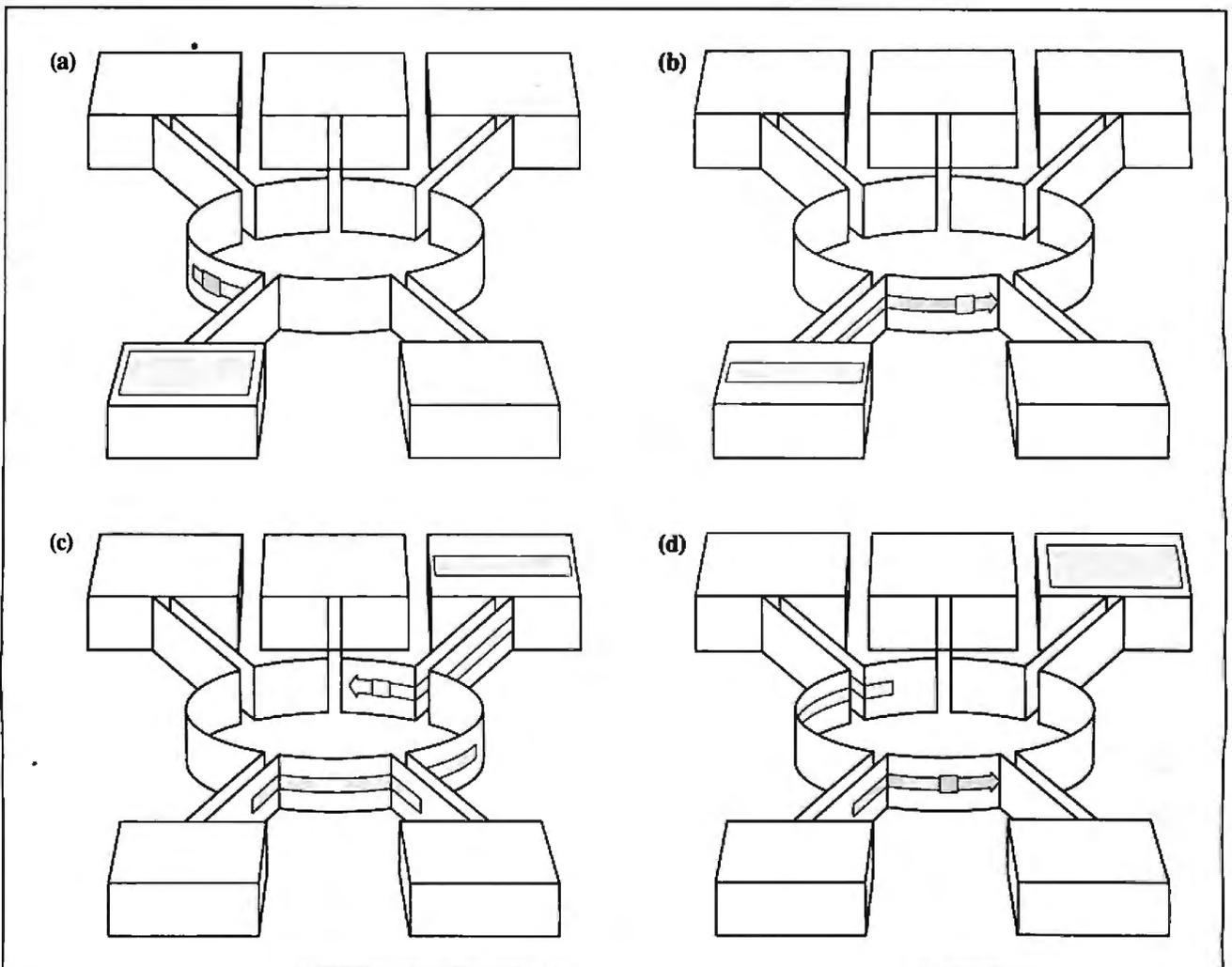
**Figure 1:** A functional overview of the Token Ring. (a) The sending station waits for a token; (b) the sending station makes the token a frame by adding addresses and data; (c) the receiving station copies data and sets the "copied bit"; and (d) the sending station removes the data and generates a new token. (Figure courtesy of IBM Corp.)
