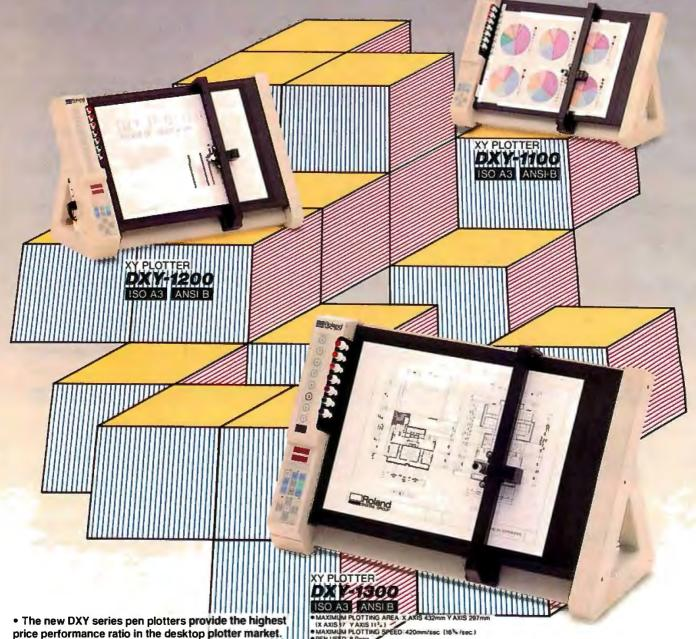
Revolutionary new micro-stepper motors deliver a maximum plotting speed of over 16 ips (420mm/sec) while maintaining superior resolution of 0.0004"/step (0.0125mm/step). With new vertical and horizontal pen arm supports, excellent plot quality is assured.
