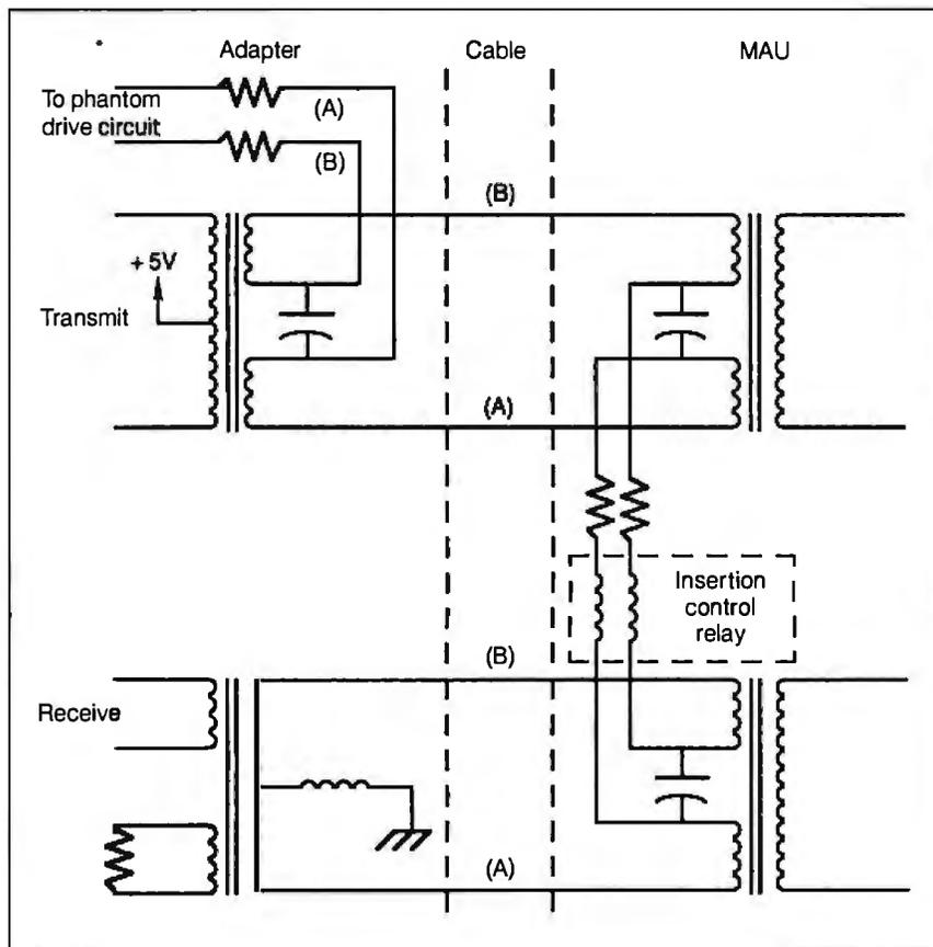
**Figure 4:** The "phantom circuit" is essential to ring maintenance. If a node is on a damaged section of the ring or if requested by the local-area-network management program, a node removes itself from the ring by removing its voltage from the circuit (deactivating the phantom circuit). The presence of too much or too little current in the phantom circuit indicates a wiring problem. (Figure courtesy of Texas Instruments.)
