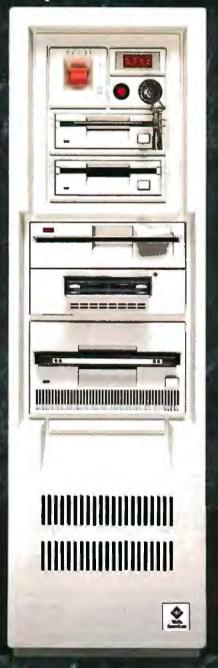
The CompuStar is also easily expanded. That's because there are seven CompuStar disk/tape compartments — six accessible from the front and an additional full-height bay inside. All this in a sleek, compact tower design that actually leaves more room on your desktop than any of the so-called "desktop" models.
