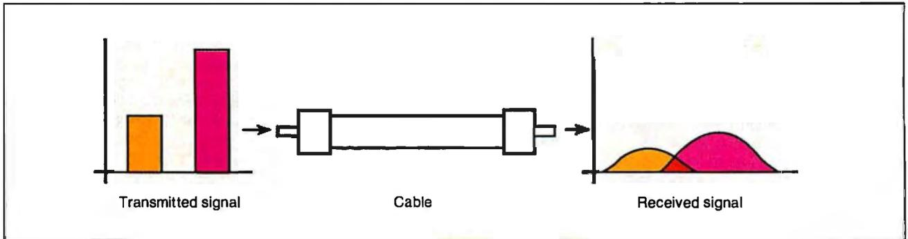
**Figure 3:** The change in signal levels over metallic cable. Beginning as a square wave, the typical digital signal will weaken and round off as it travels down the cable. As adjacent square waves do the same, the different pulses run into one another.
