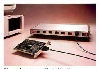
Fiberstar, the plastic optical-fiber LAN from Netronix.
