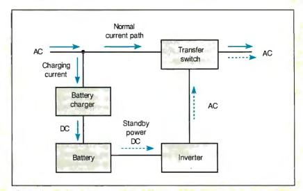
Figure A: The block diagram of a standby power system.
