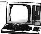
Hard to believe... but we found a stash of brand new fully factory assembled Zenith/Heath Model H/89s. These computers feature 64K/byte of memory, the Zilog Z-80 CPU and operate under CP/M. The unit incorporates a 12 inch green screen, three serial ports, and one 5 1/4" disk drive. Zenith's original price was \$1895. We have still 97 units available for sale, while supplies last we are offering the H/89 at only \$179. CP/M operating system available \$24.95
