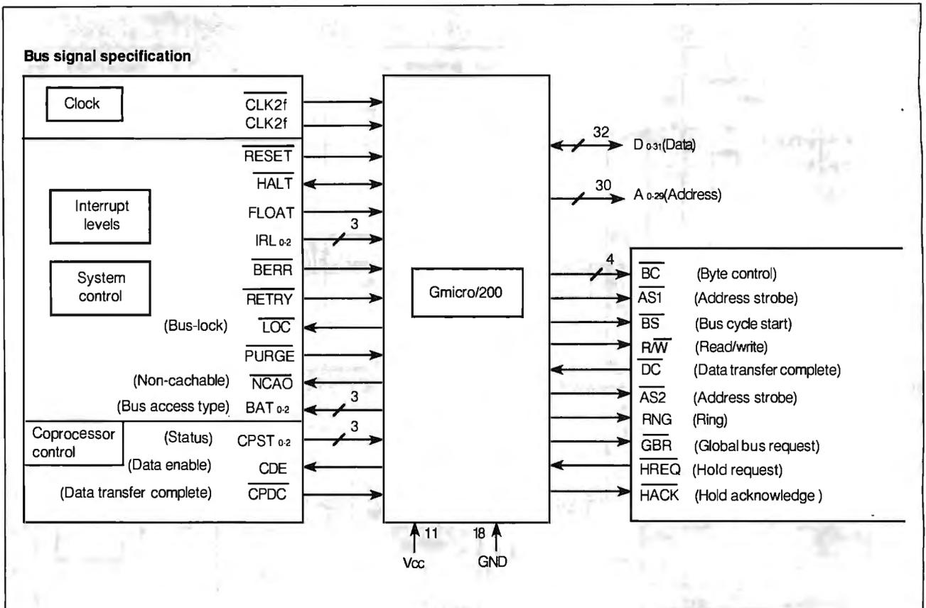
**Figure 6:** The bus signal specification for the Gmicro/200. The instruction set permits an elegant way of handling interrupts including error-handling and virtual memory.
