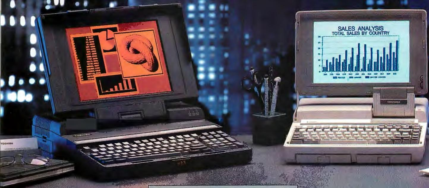
*T5200: 20MHz 386 processor, 2 internal IBM®-compatible expansion slots, VGA gas plasma display with VGA monitor port, 40MB or 100MB hard disk, 2MB RAM standard expandable to 8MB, 1.44MB 3½" diskette drive.*
