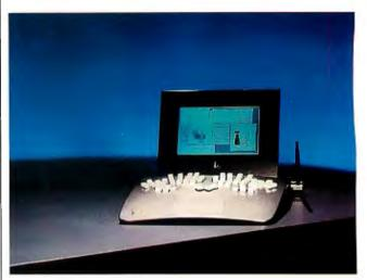
**Photo 1:** The BTRON standard PC includes a flat-panel display, an ergonomic keyboard, and a stylus pointing device. Everything from the CPU instruction set to the user interface was designed as a unit.
