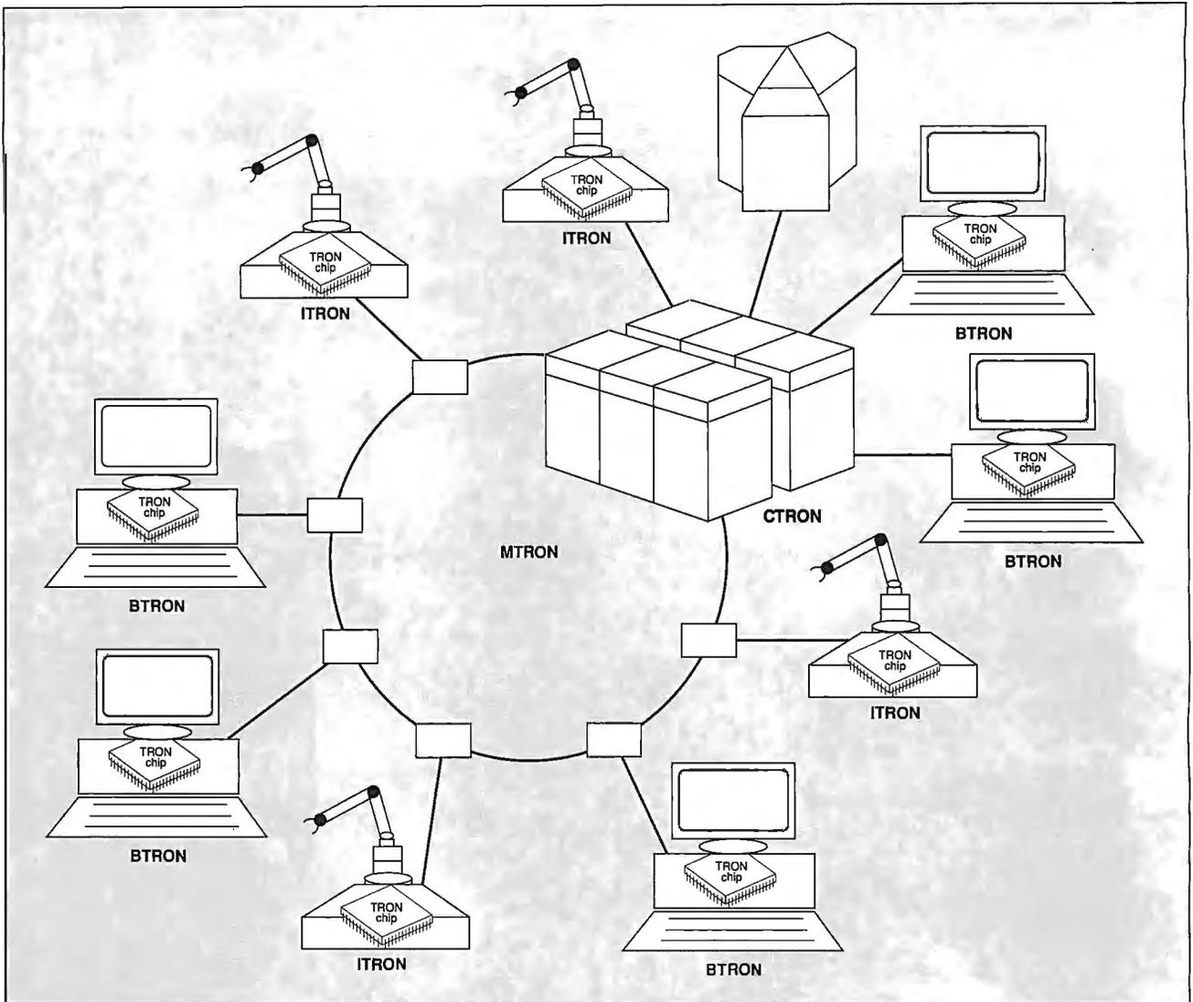
**Figure 1:** In the TRON world, BTRON workstations can communicate with ITRON industrial computers and share data with a mainframe through a CTRON file server. The network linking these and other "intelligent objects" together is MTRON.
