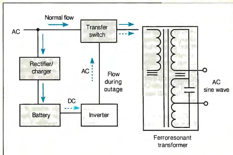
Figure C: The block diagram of a ferroresonant UPS.
