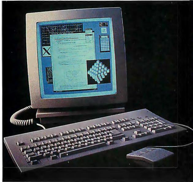
*The X Window-based NCD16 computer has an Ethernet link.*
