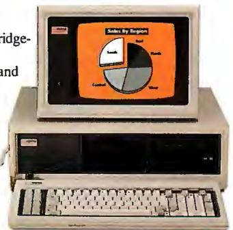
IBM® PS/2™ Model 30 286 with Bridge-File™ 5.25. Now compatible with DOS 4.0 and OS/2™. Give ALL your 3.5" systems easy access to 5.25" disks. Dual capacity 360 Kb/1.2 Mb access to all files.
