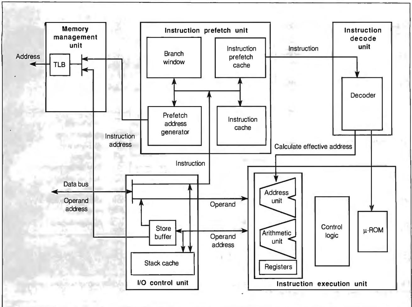
**Figure 5:** The Gmicro/200, the first generation of TRON CPUs, provides 32-bit addressing that is upwardly compatible with future 48-bit and 64-bit addressing modes. The internal structure of the Gmicro/200 provides for a very orthogonal instruction set. With the symmetry of operands, you can combine operands in any order.
