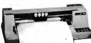
The Hitachi 672/XD is a four color 11 by 17 (B size) plotter with superior accuracy and repeatability (.3mm). The 672 accepts HPGL 7475 commands and is both Centronics parallel and RS232C compatible.
