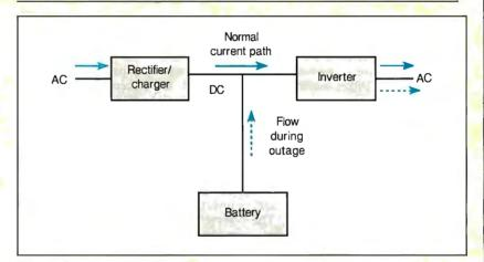
Figure B: The block diagram of a true on-line UPS.
