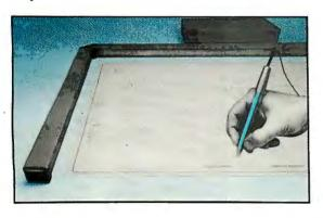
All our digitizers come complete with RS-232 output format, power supply, two-way communications, a stylus, optional one button and four button cursors, a five function menu, and are IBM-PC compatible. So no matter what your size requirements are, we've got you covered; (at low cost too!).
