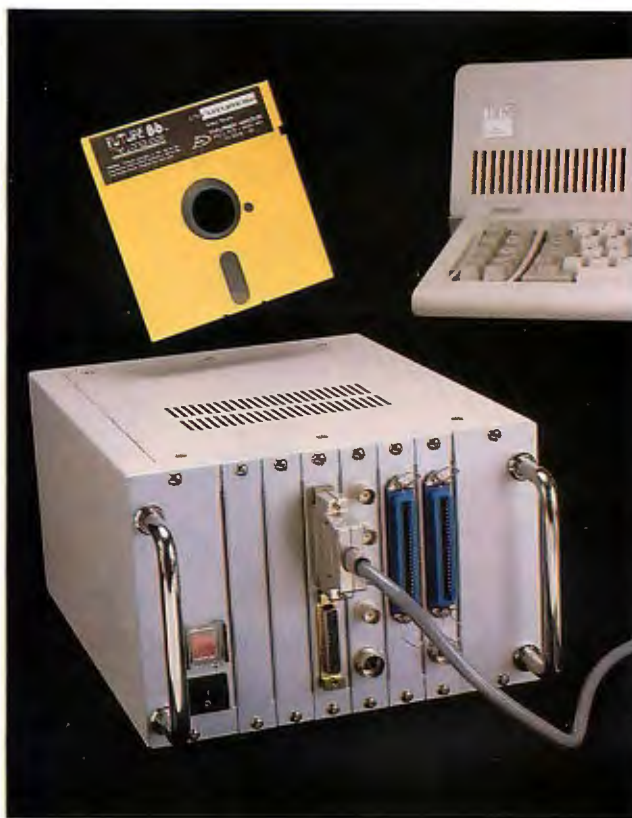
The UDM controls RS-232C and IEEE-488 I/O.
