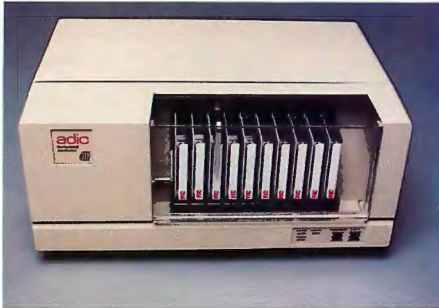
Data cartridge backup on the LANbacker 8000.
