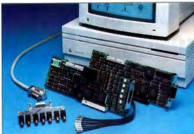
The NB-A2000 Mac II board monitors channels at up to 1 MHz.
