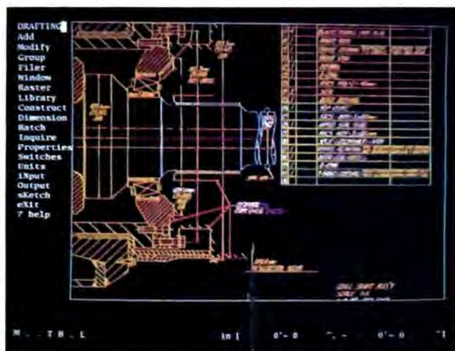
CAD Overlay lets you import scanned images to VersaCAD. The yellow lines are the scanned raster image, and the other colors are VersaCAD entities drawn over the scanned image.
