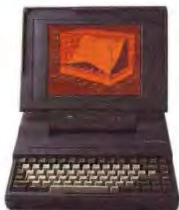
T3100e: 12MHz 80286, internal IBM slot, 20MB hard disk, gas plasma display, 1MB RAM expands to 5MB, 1.44MB 3½" diskette drive.
