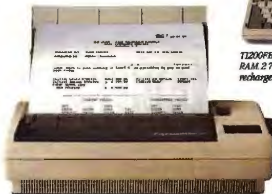
ExpressWriter 301: 4 lbs, letter-quality 24-dot print head, 60 cps, Toshiba/Qume and Epson LQ emulations, 5 resident fonts.
