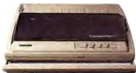
ExpressWriter 3U: 24-pin dot matrix, 180 cps draft/60 cps letter quality, 3 resident emulations (Toshiba/Qume, Epson LQ, IBM Proprinter), 16K buffer, 5 resident fonts plus card slots, 11 lbs.
