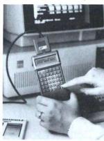
of either two or four lines of LCD display, several different keyboard designs, and from 32K to 96K of internal RAM memory. All Organiser units can use our removable and interchangeable memory modules, allowing the Organiser II to be configured to meet your unique data and program memory requirements.
