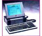
Optional paper white VGA LCD display with back-lit super twist technology.
