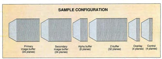
Figure 3: A frame buffer can have many bit planes and require a vast amount of memory. This configuration has a total of 96 bit planes. Assuming a screen resolution of 1280 by 1024 pixels, this represents 125,829,120 bits, or nearly 16 million bytes.
