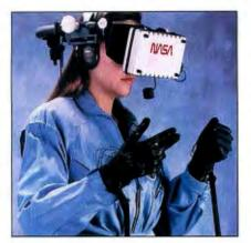
**Photo 1:** VIEW is a wide-angle, headmounted, stereoscopic display system controlled by the operator's voice, position, and gestures.
