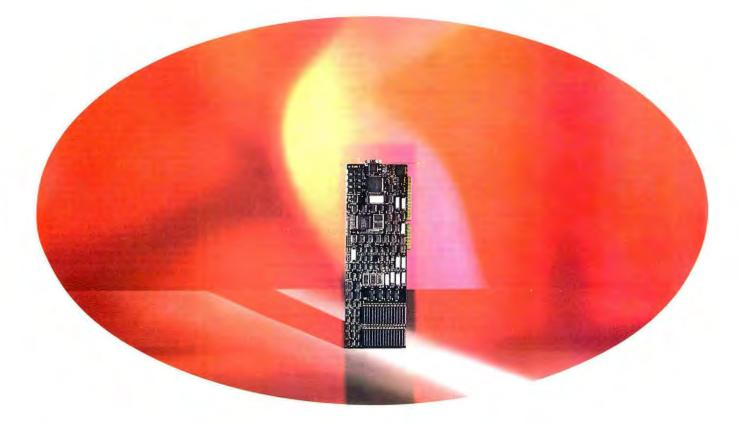
The MultiSync Graphics Engine Board. Uses 50MHz TMS \$4010 graphics processor to accelerate software applications as much as 900%.
