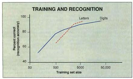
Figure 3: The figure plots accuracy rate versus the size of a training set for a backpropagation neural network. You need large training sets to achieve high accuracy rates.
