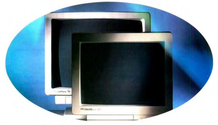
The 16" MulliSync 4D and 20" 5D monitors. Our largest high-resolution color monitors. Digitally controlled, the 4D supports VGA through 1024 x 768, the 5D, up to 1280 x 1024.
