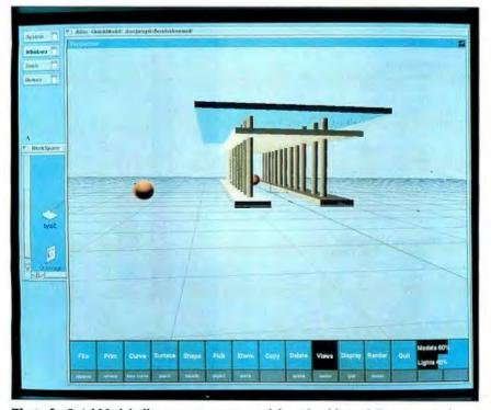
**Photo 2:** QuickModel allows you to create models with additive 3-D geometric forms in orthographic views. You can then view them in perspective and export your views to Wavefront's Personal Visualizer, a full rendering program.
