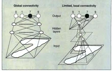
Figure 1: Back-propagation techniques enable a neural network that starts out with randomly valued connections to learn to correctly recognize input patterns. Network architectures with limited connectivity represent one way to make these recognition systems compact enough to fit on small machines.
