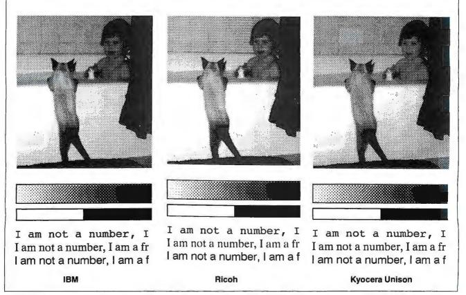
Figure 2: A sample printout from each printer engine covered in this product focus. The engines varied little in print quality, although the Ricoh engine's output lacked the sharpness of the other five samples.
