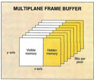
**Figure 2:** A graphical display with a single plane allows only monochrome images. Increasing the screen depth allows more colors, double-buffering for animation, z-buffering for 3-D rendering, alpha buffering for transparency, or antialiasing. The system shown here has 8 bits per pixel, which provides 2<sup>s</sup> options (256 color choices), and a portion of nondisplayable (hidden) screen memory, which can be used for fast generation of bit-mapped text, texture mapping, and pattern tiling.
