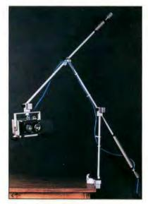
**Photo B:** The CCSV, a stereoscopic viewer fixed on a counterbalanced kinematic linkage, lets you easily enter and leave the virtual world.
