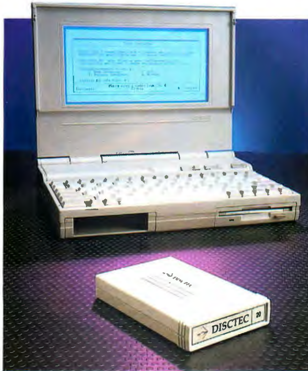
Disk Technologies' RHD 20 is a 20-MB removable hard disk drive that's fast and uses little power.
