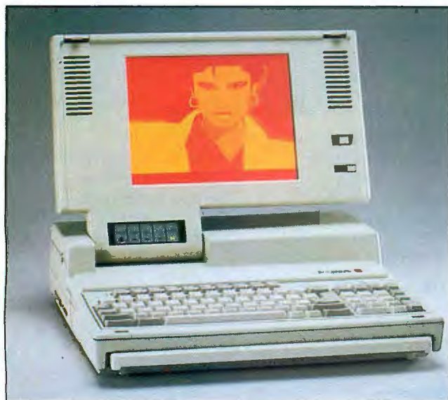
Fora's LP-386SX laptop features VGA graphics, floppy and hard disk drives, and a half-length expansion slot.
