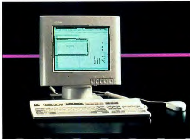
The Unisys PW 2 LAN workstation fits on the back of its accompanying monitor, out of your way.
