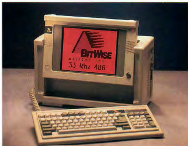
The Bitwise 486 Super Portable features VGA graphics, enough RAM for Unix, and more hard disk storage than some file servers.
