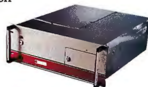
Mission Critical Rack-mount 2001: 10 option slots, 3 drive bays and a 95-130 VAC, 47-440 Hz power supply.
