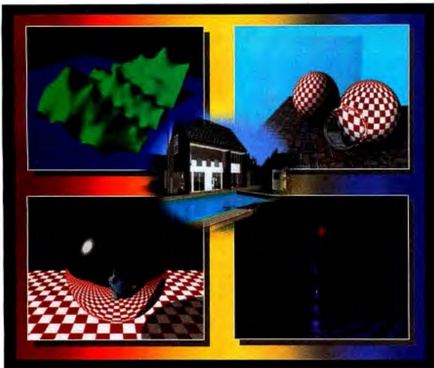
Photo 1: I created this composite 512- by 482-pixel by 24-bit image using a standard VGA monitor and Hercules Art Dept. bundled with the HGS card. Each image began as a wire-frame AutoCAD model; Big-D by Graphics Software was then used to ray-trace and render the AutoCAD DXF files. I rescaled the resulting TARGA files to 320 by 200 pixels and placed them over a 24-bit color background gradation. Finally, I vignettted the center image using the Art Dept.'s elliptical edge-fade command. (Original images and Big-D images courtesy of Butch Balingit/Digitech & Graphics Software, Inc.; file-to-slide conversion courtesy of Image Center)
