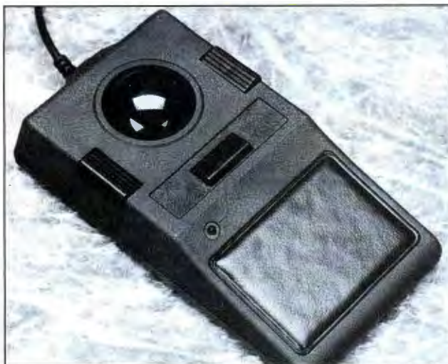
The Mouse-Trak Model M5-IND's electronics have a conformal coating to protect it when used in high-moisture areas.
