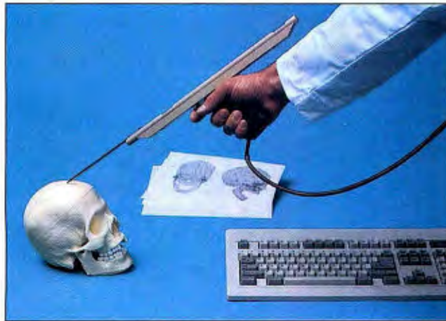
With the Series 300 digitizing system, you can capture 3-D coordinates of real-world objects.
