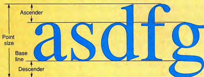
Figure 1: A font's point size is measured from ascender to descender. Traditional leading specifies the space between one line's descender and the next line's ascender. However, these DTP packages measure leading from ascender to ascender. All the packages allow you to shift the text baseline for custom subscripts and other effects.
