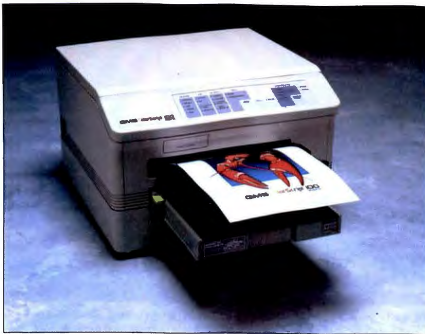
Photo 2: Some thermal wax printers, such as the QMS ColorScript 100, are PostScript compatible.
