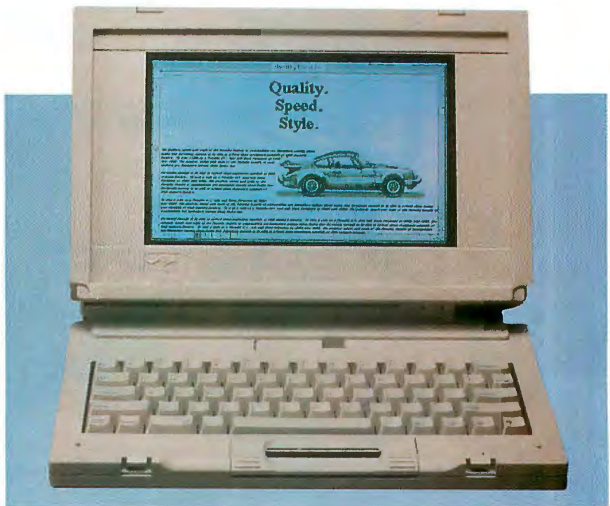
Photo 4: The Outbound Systems Macintosh-compatible laptop sacrificed the Mac Portable's cutting-edge display and trackball in favor of a normal LCD and the first use of the Isopoint pointer. Outbound's Isopoint is 4½ inches long and 1 inch high, and it resolves 101.6 pulses per inch of travel. Its low power usage keeps overall power consumption to a minimum.
