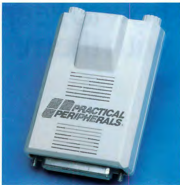
The credit-card-size, 2400-bps Practical Peripherals Pocket Modem accepts pulse or Touch-Tone dialing.
