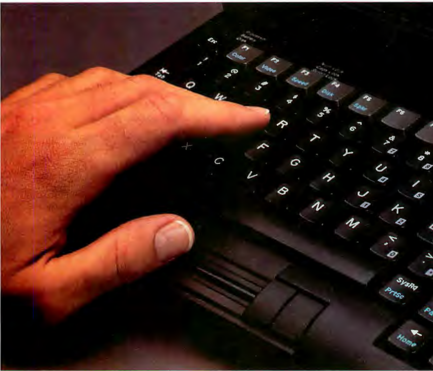
Photo 5: Grid Systems was the first company to deliver a laptop designed specifically to run Windows: The Gridcase 1550SX has a 386SX CPU and an Isopoint. Grid's Isopoint is a later iteration than the one on the Outbound, smaller in dimensions and higher in resolution. It emulates a Microsoft Mouse.
