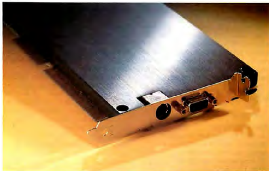
Vista's V-ATE add-in card for AT diagnostics. The distinctive metal shield and rugged bus connectors are designed for repeated installations and removal.
