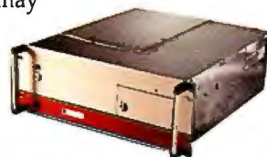
Mission Critical Rack-mount 2001: 10 option slots and 3 drive bays.
