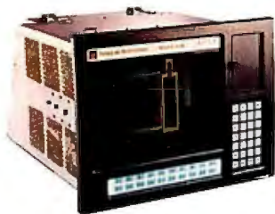
Mission Critical Workstation 1448: 9 option slots and 2 drive bays.
