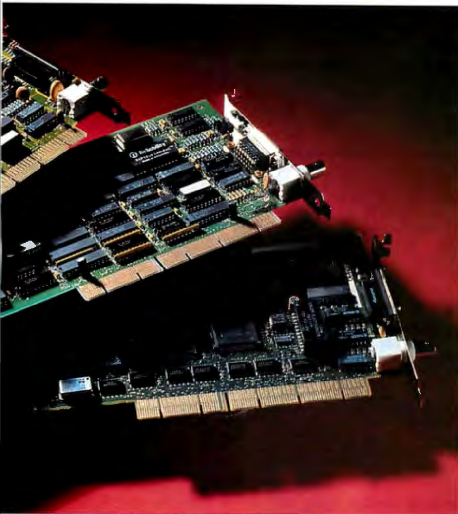
The Mylex LNE390 (left) offers the most flexibility. You can configure it for DMA, I/O-mapped, or memory-mapped operation. The Racal-InterLan ES3210 (center) communicates via shared memory. Novell/Anthem's bus-mastering NE3200 (right) is the only adapter with an on-board coprocessor.
