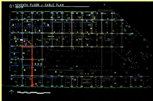
One option of Isicad's COMMAND cable management system lets you highlight an individual cable path in relation to the rest of the network. (Courtesy of Isicad)
