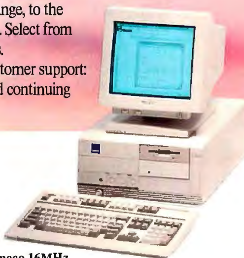
Jameco 16MHz 80386SX Computer Kit • 2MB RAM (expandable to 8MB) • 200 Watt power supply • 101-key keyboard • Multi I/O Card • Toshiba 1.44MB, 3.5" floppy drive • DR DOS 5.0 and QAPLUS diagnostic software $1199.95/JE3816 monitor extra
