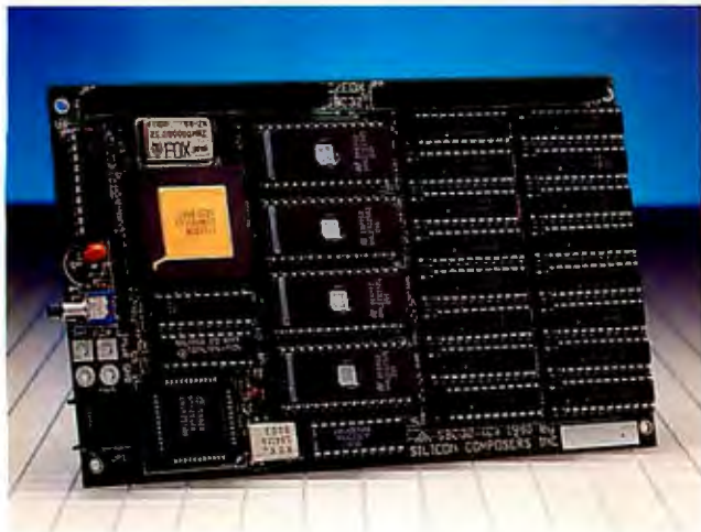
The SC/FOX SBC32 computer uses the SC32 Stack Chip microprocessor, which executes the Forth language in silicon.
