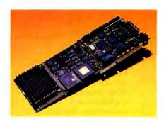
Photo 1: The Opus PM 500 is a complete SPARC system on a PC-compatible card.
