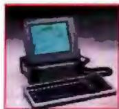
expansion slot. The matching VGA LCD display module (available in August) turns Moby Brick into a portable, go anywhere solution. The LCD features a 64 gray scale controller and the latest Sharp thin film, super twist, backlit LCD technology.
