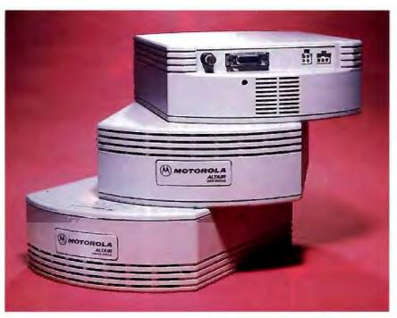
The Altair system. Shown here are the Control Module (CM) and two User Modules (UM). The grillwork hides a special six-sector microwave antenna. The back panel has connections for power, thin and thick Ethernet, and, on the CM, a special RS-232 cable for UM security registration. Installation can be as simple as placing the unit on your desk and connecting the Ethernet cable.
