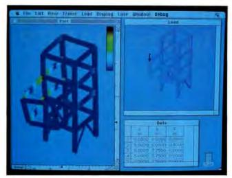
Multiframe shows a load being applied to a structure in the right window, while showing in the left window an exaggerated deflection shape resulting from the load. The colored bar provides a minimum and maximum scale for the bend.
