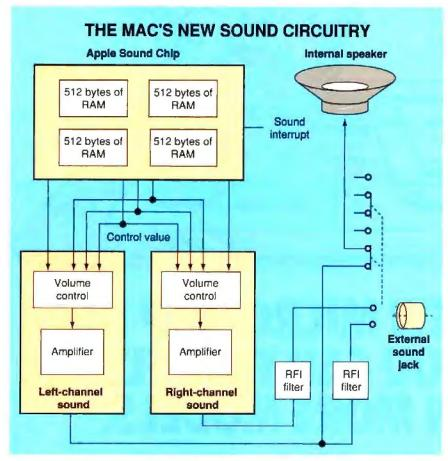
Figure 2: The introduction of the Mac II brought a new sound circuitry using the Apple Sound Chip, which supports stereo sound. Since the ASC implements much of the classic design's software in silicon, it provides complex sound generation using little CPU overhead.
