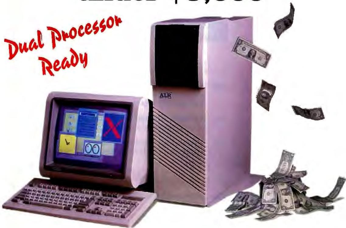
Speaking of adding processors, the ALR POWERPRO is also the only affordably priced server/host system to give you an upgrade path to SYSTEMPRO™ compatible dual processing. Just plug in our POWERPRO 33-MHz i486 MP1 and MP2 modules, and the POWERPRO will instantly become a true symmetrical dual processing system. The POWERPRO can truly
