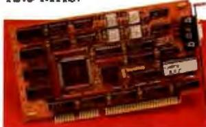
The card's Ultra VGA driver increases the usual 16 or 256 colors on a monitor to 742,813, with near-photographic quality, according to the company. It has a 60-Hz refresh rate and 512 KB of video RAM. Software drivers include Super VGA for Windows 3.0 and Ultra VGA for Windows 3.0 and Autodesk applications.
