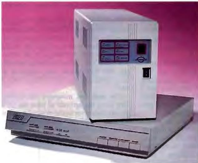
*The Para Systems (top) and Zentao UPSes monitor power conditions and alert network workstations if a power failure occurs.*
