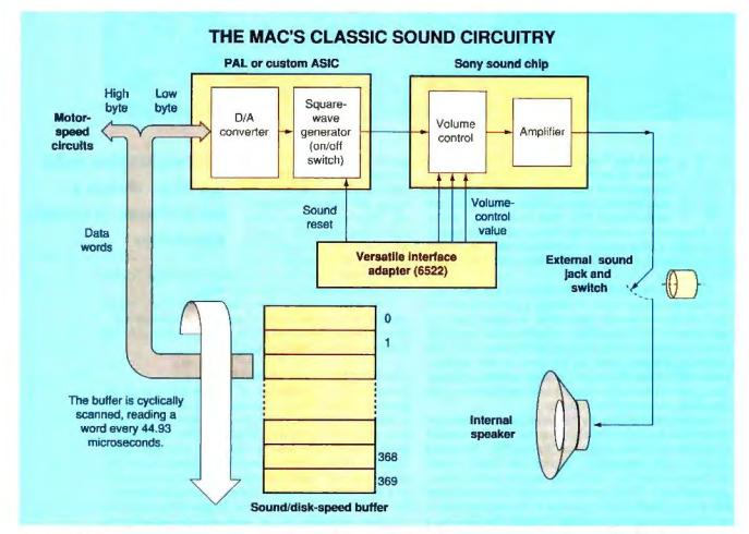
Figure 1: This block diagram shows the "classic" sound design in the Mac Plus, SE, and Classic. The sound buffer data is interleaved with the Sony disk speed buffer. The Sound cdev sets the digital volume value.
