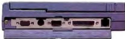
**LEFTSIDE CONNECTORS:** Behind a hinged side panel, SlimLite has ports for external VGA monitor and keyboard plus a 9-pin serial port, parallel port and phone jack plug.
