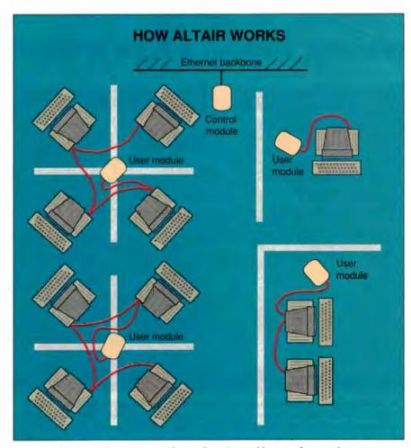
A typical Altair topology isn't totally wireless: You cable up to four workstations to each User Module, which then makes a line-of-sight connection to the Control Module. You cable the Control Module to your file server, host, or network backbone. Motorola suggests mounting the modules high to avoid obstructions.
