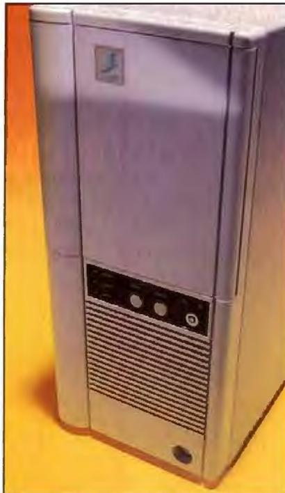
**T**he FlexComServer 100 is a plug-and-play alternative to installing processor cards on your LAN. It consists of a 16-MHz 286 system bundled with Cubix processor cards, a network card, a floppy disk drive, and all the software you need to get a dial-in system up and running. Evergreen Systems also bundles a copy of DMA's pcAnywhere IV/LAN remote-control software. I tested the FlexComServer 100 (\$2195) with two Cubix CP-2286 dual-286 processor
