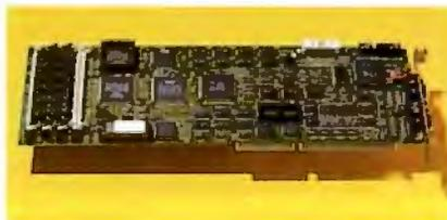
**T**he QL 3001, although similar in philosophy to Alloy's PC-Slave/286 card, features considerably more powerful hardware: a 20-MHz 386SX processor, VGA, and 1 MB of memory (with SIMM sockets for up to 16 MB). Each card, which includes support software, sells for \$1845. (Cubix also sells a 286-based card for \$1040 and a 16-MHz 386SX card for \$1395.)
