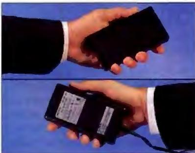
TOP: Rechargeable Ni-Cad battery weighs 1.05 lbs.
