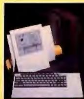
Synapse, the manufacturing division of Technology Design (Bellevue, WA), has introduced a PC compatible called **Emily, Julie, and Max**. Emily, the keyboard, looks like a spiral notebook, with a wide, sloping front. Julie is the 10-inch, VGA-compatible, backlit LCD. It plugs into Max, the CPU, which looks like five books standing on end. A 25-MHz 386-based model sells for \$7995 with a 100-MB hard disk drive, a 3½-inch floppy disk drive, 4 MB of memory, and five 32-bit slots. ■
