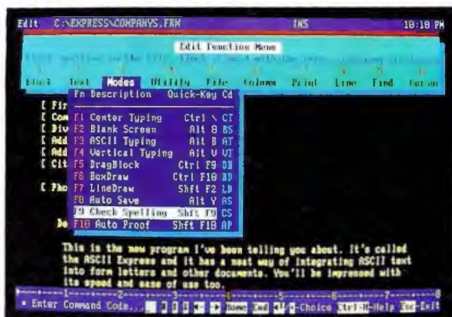
In this example of ASCII Express's drop-down menu box in the editor, the cursor is positioned on the Check Spelling feature.
