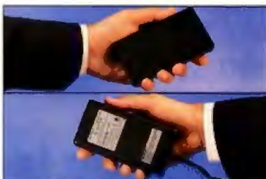
TOP: Rechargeable Ni-Cad battery weighs 1.05 lbs. BOTTOM: Compact "AC Pack" weighs well under a pound.
