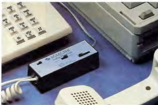
Laptop Phone Link works without software or external power.
