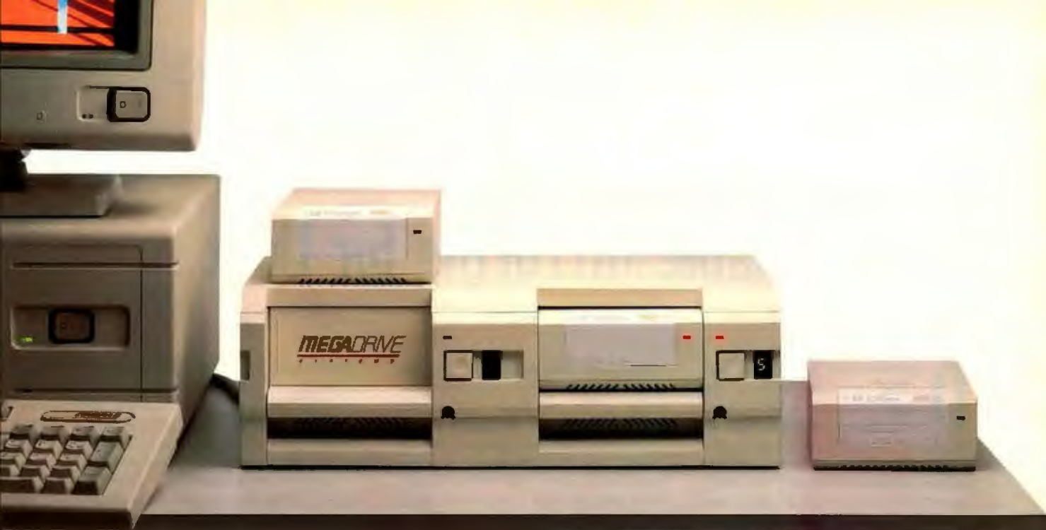
Millennium two-slot horizontal docking bay and three removable hard drive modules
