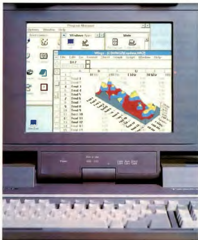
Photo 2: The Toshiba T3200SXC's display is simply gorgeous. The backlit LCD, based on active-matrix technology, responds quickly enough to keep up with a mouse cursor.
