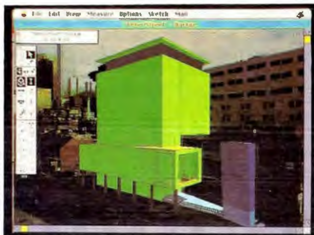
Alias Upfront lets you place buildings and other objects into a scanned photograph. When you click on three vertices of an object in the scanned image, the program matches the building to the perspective in the photograph.
