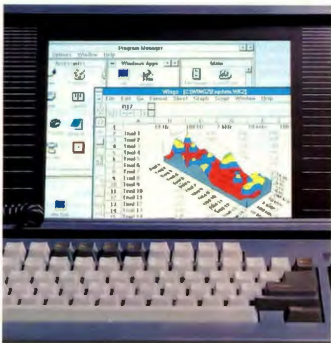
Photo 1: The Dolch C-P.A.C. 486-33E handles 256-color VGA modes. It uses a sophisticated LCD controller to coax other colors out of Sharp's active-matrix color LCD panel.
