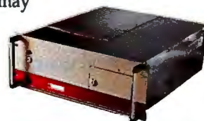
Mission Critical Rack-mount 2001. 10 option slots and 3 drive bays.
