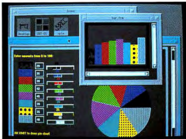
Jam for Interbase can display multiple data objects, including arrays and geographical data in Motif (shown here) or in character mode. An intelligent emulator lets Jam applications on PCs connect to the servers running Interbase.
