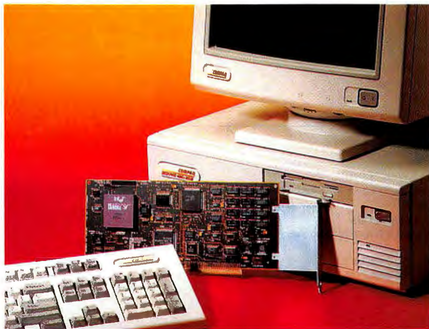
The Compaq Deskpro 486s/16M, with its upgradable processor card. On the card is the new 16-MHz version of the Intel 486SX chip.
