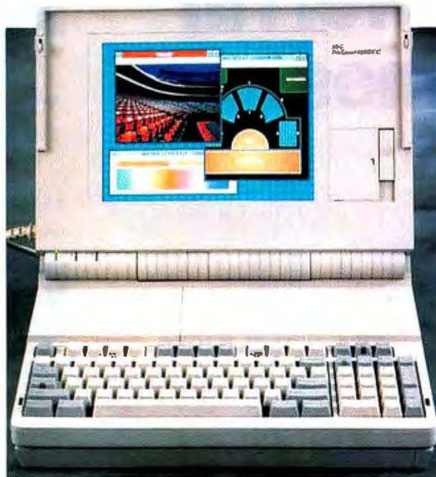
The ProSpeed 486SX/C works in Windows 3.0 and supports 256 colors and Super VGA.
