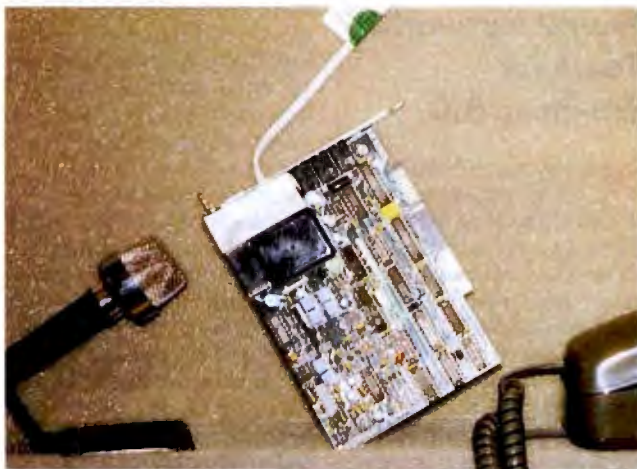
The StarTalker interactive voice-response card can record and play back speech and other sounds to and from your computer's hard disk, via a microphone or a telephone.
