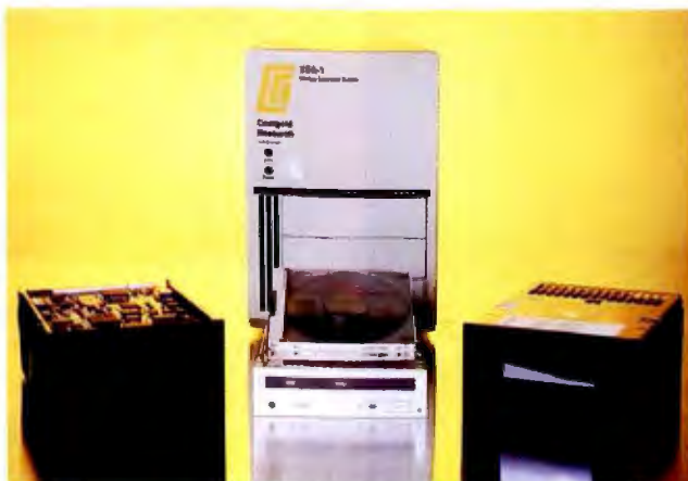
One XSA-1 Storage Expansion System can accommodate up to 4 gigabytes of disk storage or a mixture of hard disk drives, tape drives, magneto-optical devices, cartridge tapes, and CD-ROM drives.
