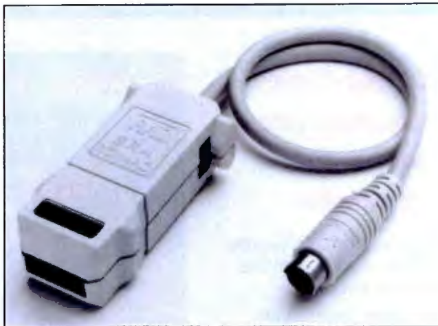
The SRM-3D/Mac and SRM-3A/Mac short-range miniature modems for the Mac allow full-duplex, asynchronous transmission over four-wire telephone lines at data transfer rates of up to 19,200 bps.
