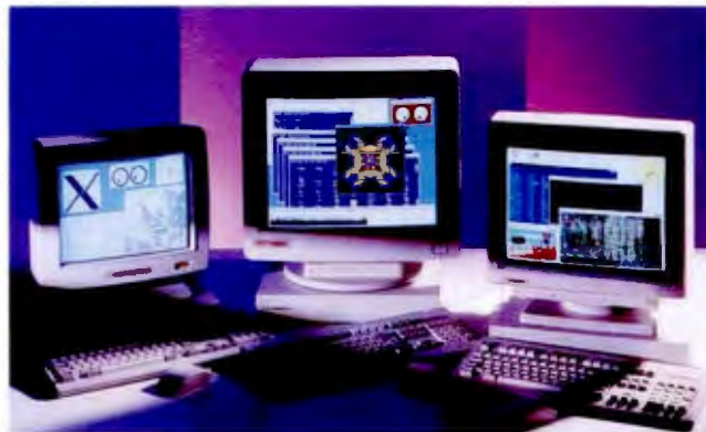
The 4500 series of X Window System terminals run at 50 MHz and include 1 MB of RAM, 16 colors, and over 480 fonts.
