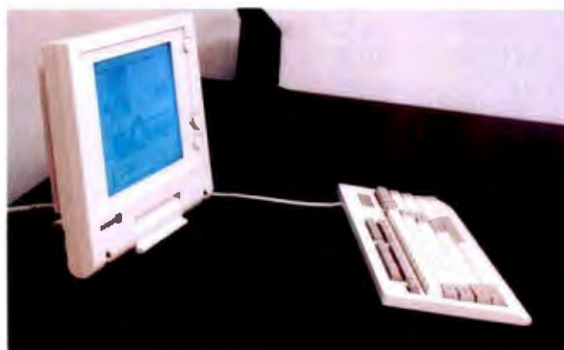
The Sygnos-S28 stand-alone LCD monitor is compatible with CGA, EGA, VGA, and MGA standards.
