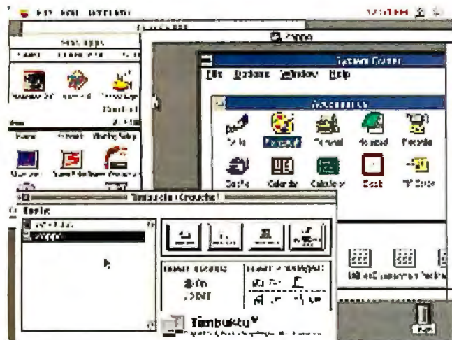
Screen 1: The Mac version of Timbuktu being used to control Windows. You can operate Mac software and then click on the background window to regain control of the PC when required. The white pointer belongs to the remote PC; the black pointer is the Mac's.
