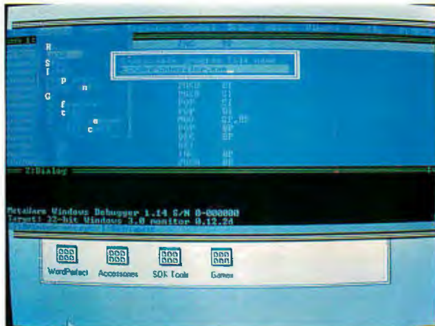
According to MetaWare, you can use its debugger to debug 32-bit applications on your development machine without using an extra terminal or computer.
