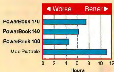
Figure 2: Battery test results show that the new PowerBooks aren't as long-lived as the old Mac Portable. However, the greatly reduced weight and better screen compensate for the shorter battery life.
