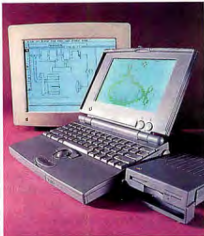
Photo 2: The PowerBook 100, with an Envisio memory/video expansion board. Envisio's Notebook Display Adapter is driving a second screen on the AppleColor 13-inch monitor in the background while providing an extra 2 MB of RAM.
