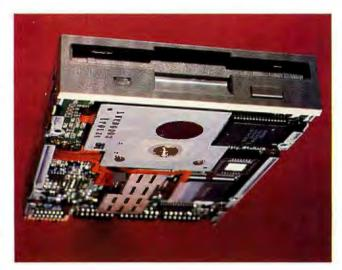
track pitch. Floptical uses closed-loop servo-positioned heads that read rings that are preprinted on special disks. The result is that Insite can cram 1245 tracks per inch onto the medium, compared with 45 to 135 tpi for floppy disks. The linear density is higher, too, at nearly 24,000 bits per inch (versus 17,000 bpi for high-density drives).
