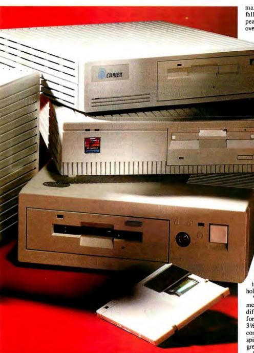
than a floppy drive and far more convenient than a tape, a 3½-inch MO drive is useful for storing archival copies of files and for primary storage of large files that need to be loaded only once; it could even
