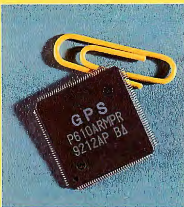
Photo A: The remarkable size of the ARM 610 is only apparent when compared directly with a universally recognizable object. GPS (GEC Plessey Semiconductors) recently became the second source for the ARM processor range.
