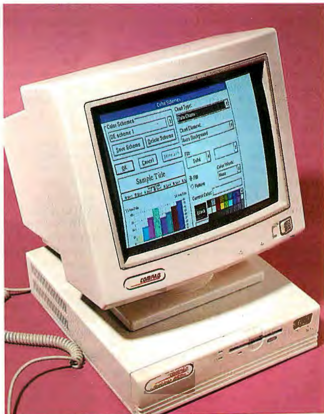
The Compaq ProLinea 3/25s is one of two 25-MHz 386SX models intended for users with limited budgets and experience.
