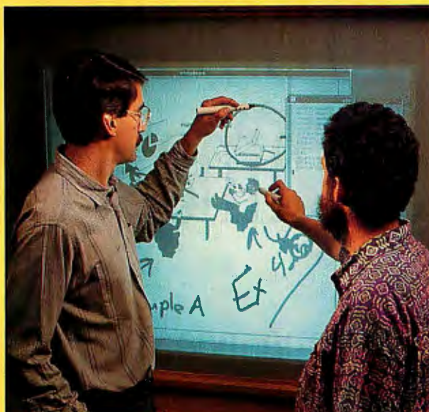
Photo A: This Xerox PARC computerized whiteboard uses a projected LCD and a stylus technology that were developed for this application. Several of these systems are connected to the Xerox network.
