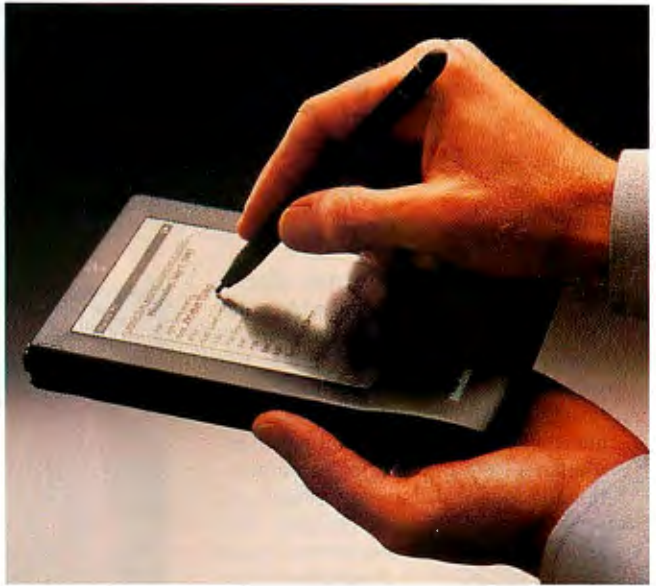
Photo 1: The Newton is the first in a series of what Apple refers to as PDAs. This pen-input hand-held system combines a fast RISC processor with an innovative new operating system and software. Apple expects to sell the Newton for less than $1000 when the system becomes commercially available in January 1993.
