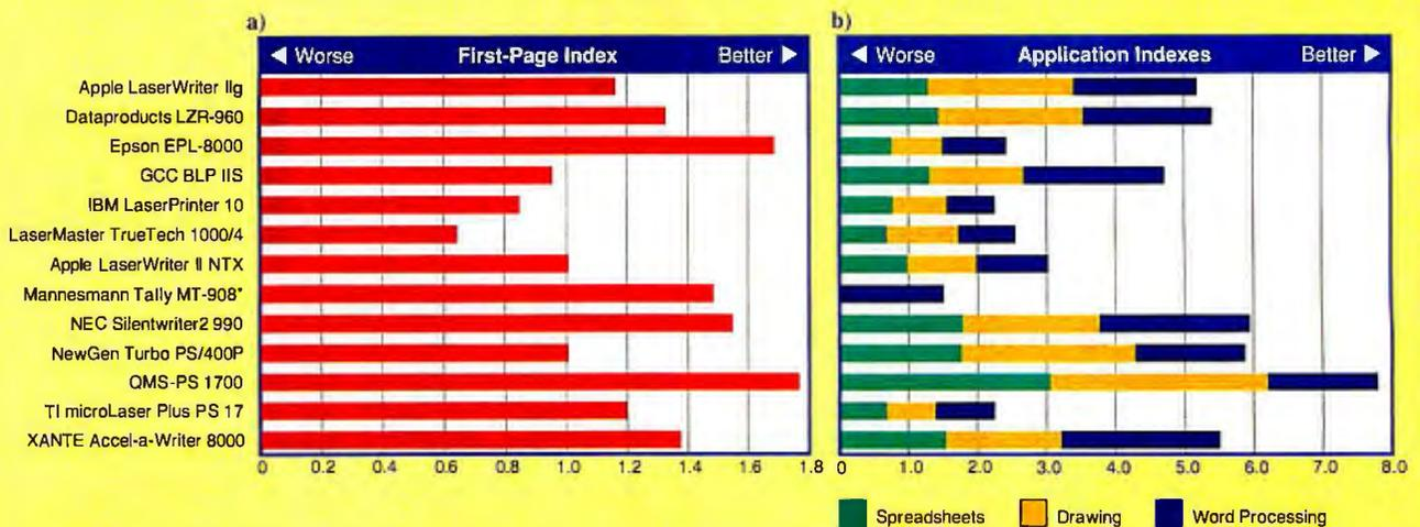
(a) The first-page index tracks each printer's performance on a single page of text, comparing completion time against that of the Apple LaserWriter II NTX. We started timing when the print command was entered and stopped timing when the page fell into the output tray. This test evaluates how efficiently a printer can handle memos and simple business correspondence.
