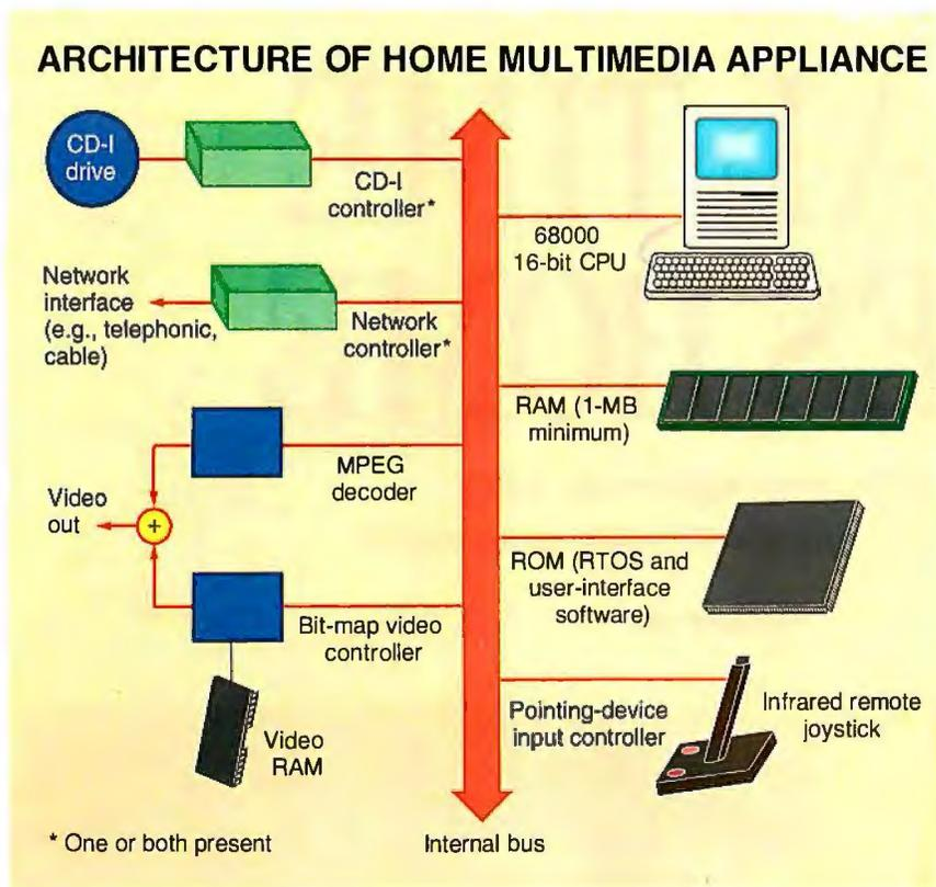
**Figure 1:** The architecture of a home multimedia appliance has most of the same components as a low-end PC, with digital video and audio decoders added. The CPU and RTOS manage the flow of data from the optical disk or network interface to the decoders and run the GUI.
