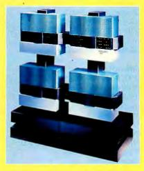
The GigaCube's modules can be stacked to build walls with up to 16,084 processors.
