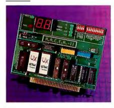
Racer II shows the current test operation on a seven-segment numeric display to alleviate binary decoding.
