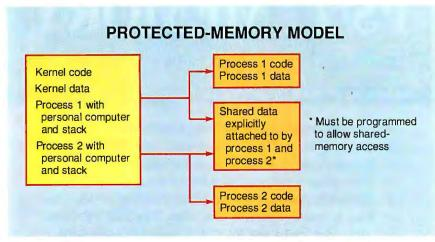
**Figure 1:** The protected-memory model reserves protected data and code areas for each process. Provisions for sharing data between processes must be specially programmed.
