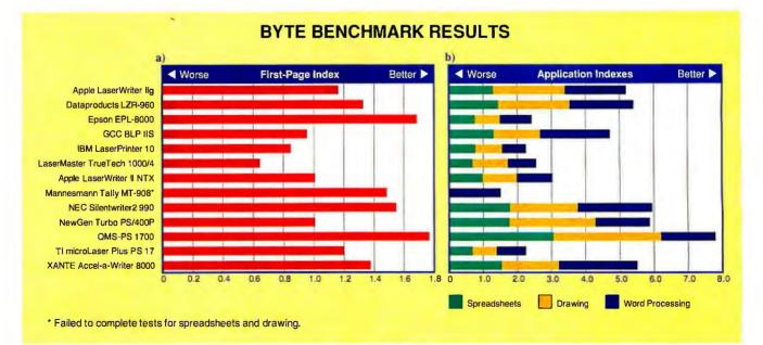
(a) The first-page index tracks each printer's performance on a single page of text, comparing completion time against that of the Apple LaserWriter II NTX. We started timing when the print command was entered and stopped timing when the page fell into the output tray. This test evaluates how efficiently a printer can handle memos and simple business correspondence.
