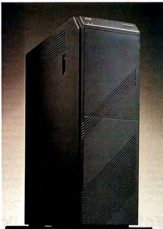
*The Series 6000i Model 640 Unix multiuser system provides more than 2 GB of disk space.*
