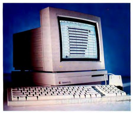
The Mac LC II packs a 68030 CPU, 4 MB of RAM, and 32-Bit QuickDraw capability into a compact box.
