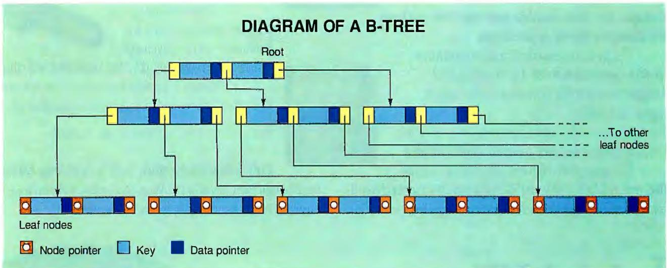
The search for a particular key always begins at the root. If the key is not found, the search concludes in a leaf node where the key would be if it were in the tree. If the search is in preparation for an insert operation, the location where the search ends is where the insert begins.
