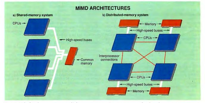
Figure 2: (a) In shared-memory systems, multiple processors communicate over a common bus through a common memory store. (b) In distributed-memory systems, each processor has its own memory store and communicates via high-speed links.
