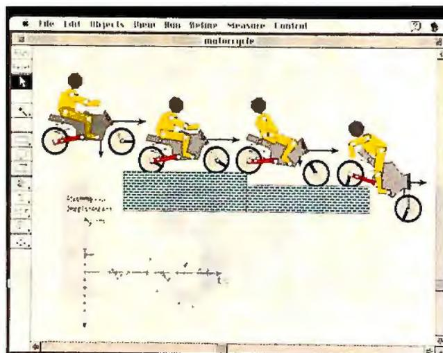
*This screen from Interactive Physics II shows the effect that the mass of the rider's body and the motorcycle, friction, gravity, and speed create as the biker drives down a step. If handlebars had been added to the cycle, the rider could have compensated for the extreme bending of back, knees, and elbows.*
