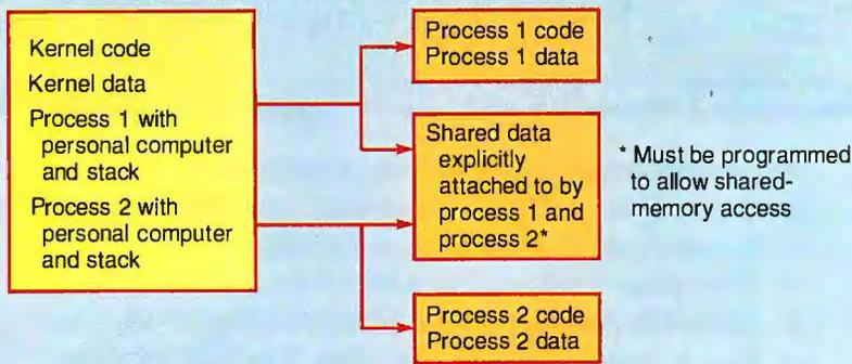
**Figure 1:** The protected-memory model reserves protected data and code areas for each process. Provisions for sharing data between processes must be specially programmed.
