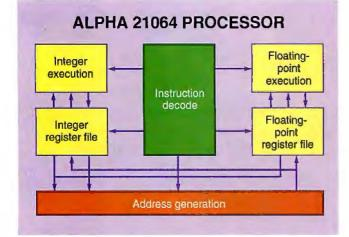
**Figure 2:** Avoiding bottlenecks is the goal of the Alpha core architecture, shown here with distributed floating-point and integer register files and execution logic.
