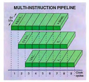
**Figure 3:** Multi-instruction pipelining requires paying special attention to instruction interaction. In this example of a fourway machine, the instructions E and J cannot execute until the result of A has been computed. However, special bypass logic—a standard architectural attribute—sends both E and J the results of A at the same time the results are entered into the A register, so they don't have to wait an extra cycle.
