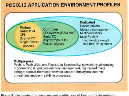
**Figure 2:** The application environment profile core of Posix.13 is the minimal profile. Successively larger and more robust application environment profiles build on this core.
