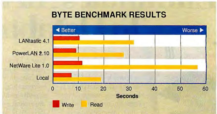
LANtastic 4.1 comes close to toppling PowerLAN 2.10, the fastest peer LAN we've tested. The newest LANtastic also easily outguns Novell's NetWare Lite. Local tests (timed directly on the host machine) are included for comparison.
