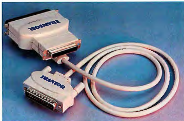
The MiniSCSI Plus connects CD-ROM and SCSI devices to laptops.
