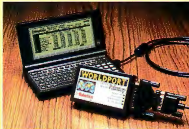
USRobotics's WorldPort Palmtop Fax/Data Modem provides fax operation to hand-held PCs without the need for a separate software package.
