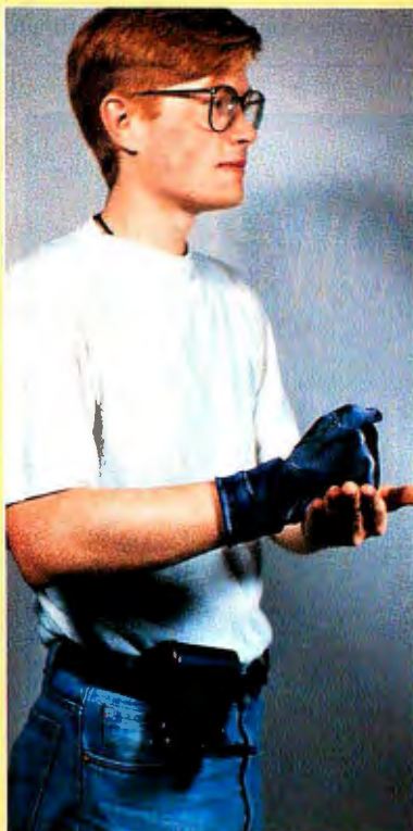
Photo B: To help hearing-impaired people communicate with those who don't use American Sign Language, students at Carnegie Mellon developed this prototype translator. The design uses gloves with sensors to send hand- and arm-movement information to a personal computer. Software converts the signals into English words, which are synthesized and output over a loudspeaker. (Courtesy of Carnegie Mellon University)
