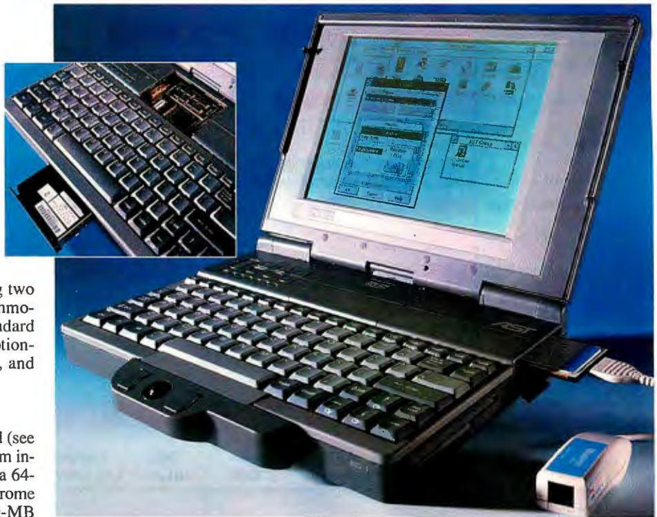
AST's new PowerExec notebook features PCMCIA support, a clip-on trackball, an upgradable screen, and (inset) a removable hard drive and an upgradable CPU.
