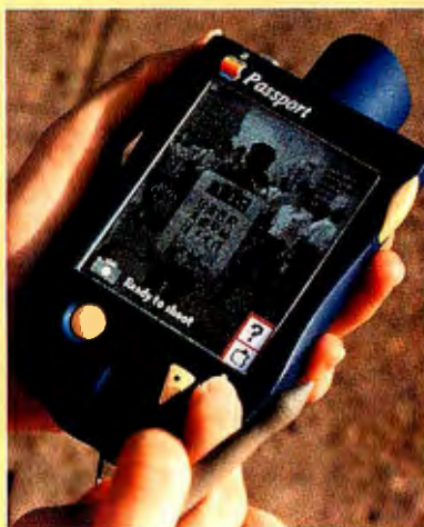
Photo A: The Passport combines digital photography and character-recognition technologies with bilingual dictionaries on chips. Using this hand-held device, you can capture an image of something you'd like translated and see the translation of the words or symbols. (Courtesy of Carnegie Mellon University)
