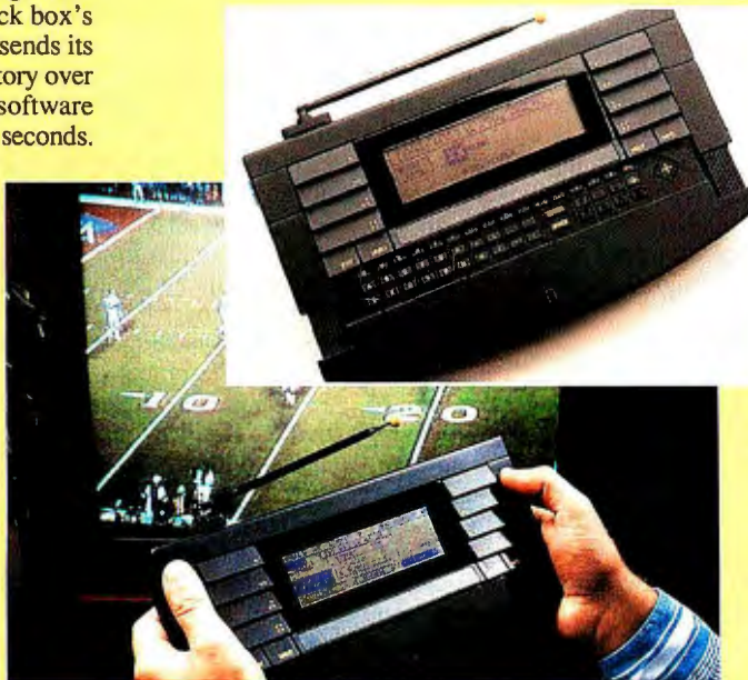
Unlike with other ITV services, Interactive Network's display appears on the hand-held control unit and not on your TV. The unit has an 8-row by 40-column LCD and a miniature keyboard. (Photo courtesy of Interactive Network)
