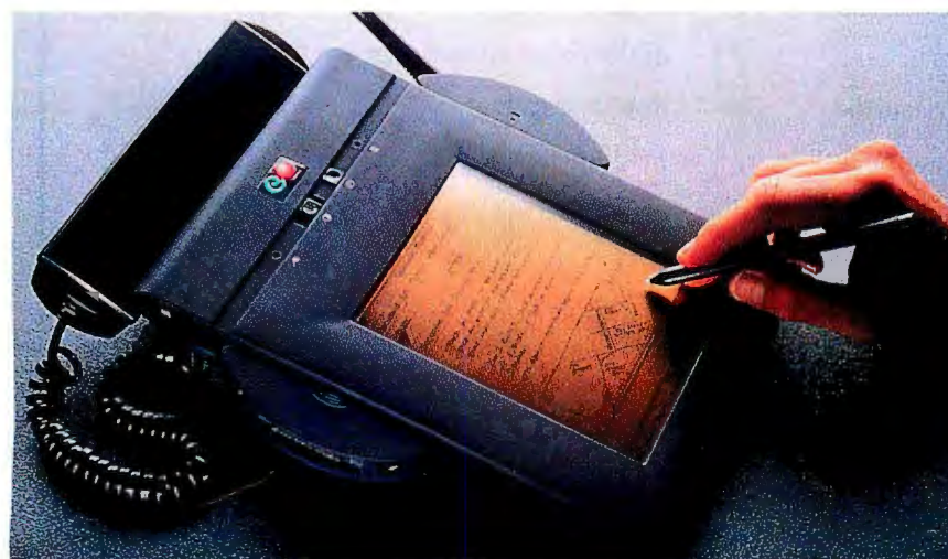
Photo 1: The EO 440's screen is a standard 640- by 480-pixel VGA display with 110-dot-per-inch resolution. Shown is the optional CellPhone module, which lets the internal modem work over the cellular telephone system.
