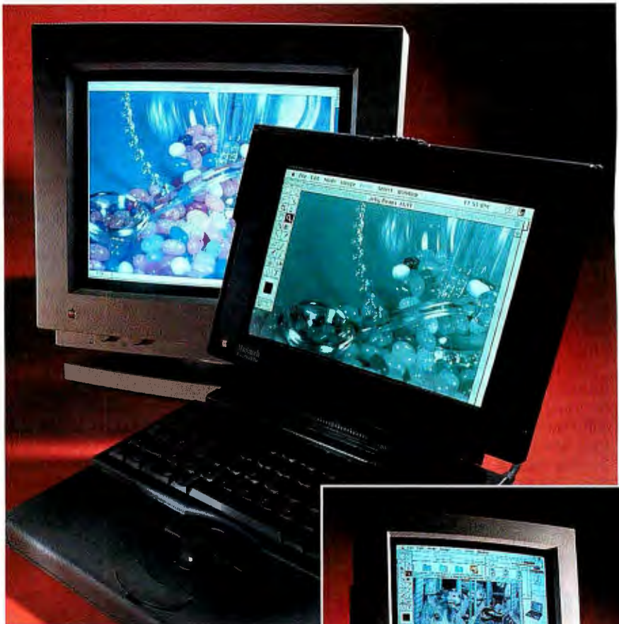
Photo 1: The PowerBook 180, shown here with an external color monitor, bundles more performance than a Mac IIci into a 9.3- by 11.25- by 2.25-inch package.
