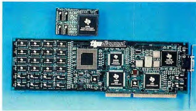
The Diamond 32-bit graphics accelerator board lets you do rendering in true color.
