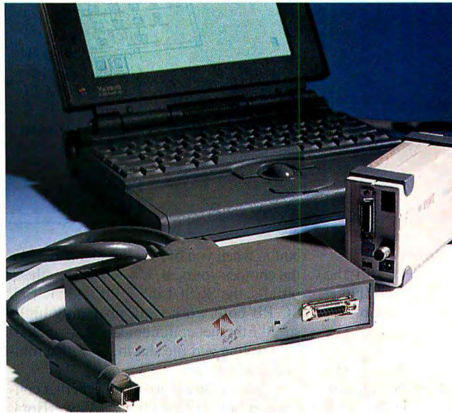
Photo 1: Two ways for PowerBooks to tap into Ethernet: Asanté's EN/SC PB (left) and Dayna Communications' DaynaPort SCSI/Link-3 PB (right).
