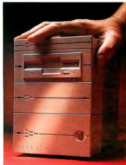
Sized to take up minimal desk space, the SmartStack modular storage system can run up to seven SCSI peripherals.
