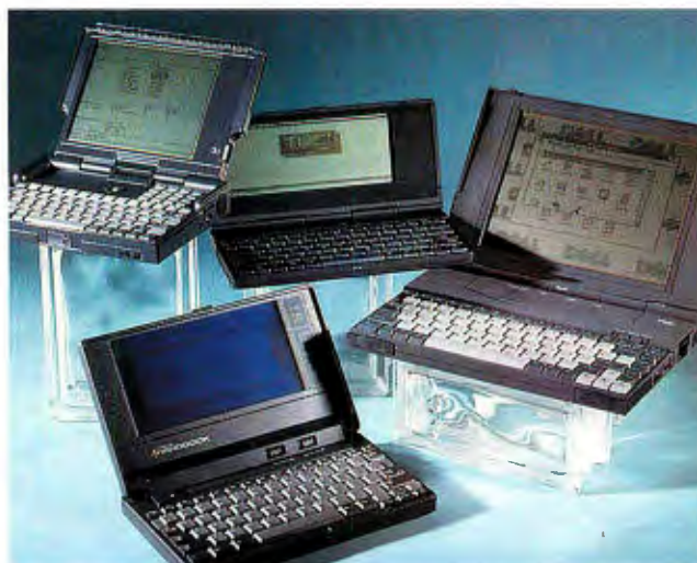
Photo 1: Subnotebooks come in ultraportable sizes but still run standard MS-DOS software. The price you pay for compactness is a cramped keyboard or a tiny screen.
