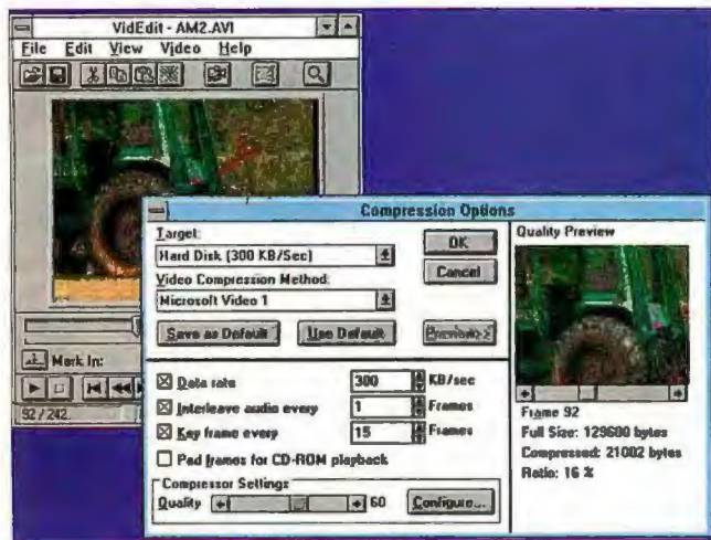
Screen 2: VidEdit, Video for Windows' editor and processor. The dialog box shows the video compression interface, which provides instant feedback through the quality preview window. (Video clip courtesy of Firstlight Productions)
