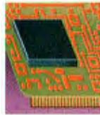
**DAUGHTERCARD:** This board plugs into a special connector on the motherboard and links the Pentium to a secondary cache at CPU speed over a 64-bit bus.
