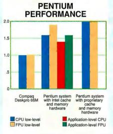
Figure A: Pentium systems can provide nearly twice the performance of a Compaq Deskpro 66M with a 66-MHz 486DX2. One Pentium system, which had its own CPU support circuitry, did better than the other systems we tested.
