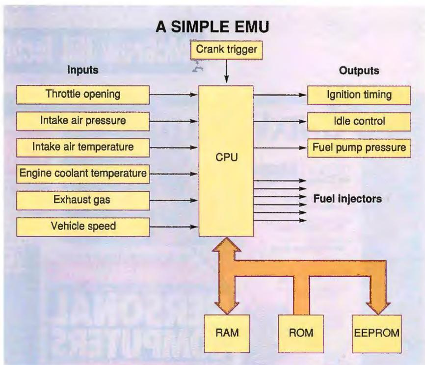
**Figure 1:** A typical EMU processes multiple inputs using engine "maps" in RAM, ROM, or EEPROM to control engine fuel injectors and ignition and idle controls. The turning crankshaft serves as the CPU clock.
