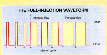
Figure A: Fuel injectors work by pulse-width modulation of fuel flow. Computers such as Ford's EEC-IV can easily generate such waveforms to control the fuel-injection process.
