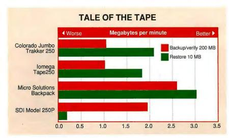
The graph indicates the kind of performance you can expect when backing up and restoring a typical mix of data. The Micro Solutions Backpack was the fastest drive. The SDI Model 250P may have posted better restore times, but its software insisted on scanning an entire tape even after recovering the requested files.
