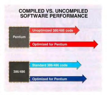
Figure 2: Based on Intel's estimates, Pentium-optimized applications will run about 30 percent faster than unoptimized programs on Pentium systems and 5 percent to 10 percent faster on 386/486 systems.
