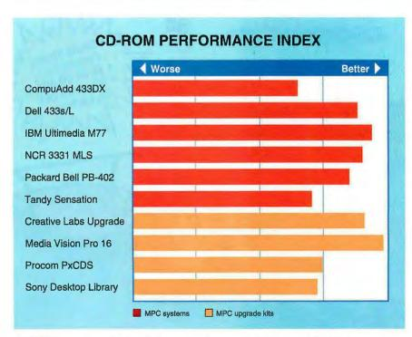
CD-ROM drive speeds are a key factor in the overall performance of an MPC system. Media Vision's Pro 16 Multimedia System MPC upgrade kit consistently proved to have the fastest overall CD-ROM drive with the NEC-84J. All MPC upgrade kit tests were performed using an MIS 486/66 system. Performance ratings between MPC systems and upgrade kits should not be compared head-to-head.
