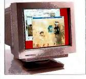
er Saver mode, where the power draw is cut to approximately 12 and 16 W, respectively. You can set the Power Saver mode to last anywhere from a few seconds to 60 minutes. When the monitor enters the second stage, the Power Down mode, power consumption drops to about 8.5 and 11.5 W, respectively. When in the Power Down mode, it takes about the same amount of time to wake the FlexScan as it does to cold-start the monitor.
