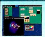
Iris Explorer's visual-programming interface is a simple way to take advantage of Silicon Graphics' rich data-visualization capabilities. You can rotate, walk through, and even fly through the virtual objects that represent your data. You can add color mapping, lighting, and surface characteristics to the data. Your data may not have any spacial characteristics of its own, but you can explore it as if it were an object in your hand.
