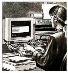
A PC for a blind user, equipped with an Oscar optical scanner and a braille printer, both by TeleSensory. The optical scanner converts text into ASCII code or into proprietary word processing format. Files saved on disk can then be translated into braille and sent to the printer. Visually impaired users can also enlarge the text on the screen by loading a TSR software magnification program.
