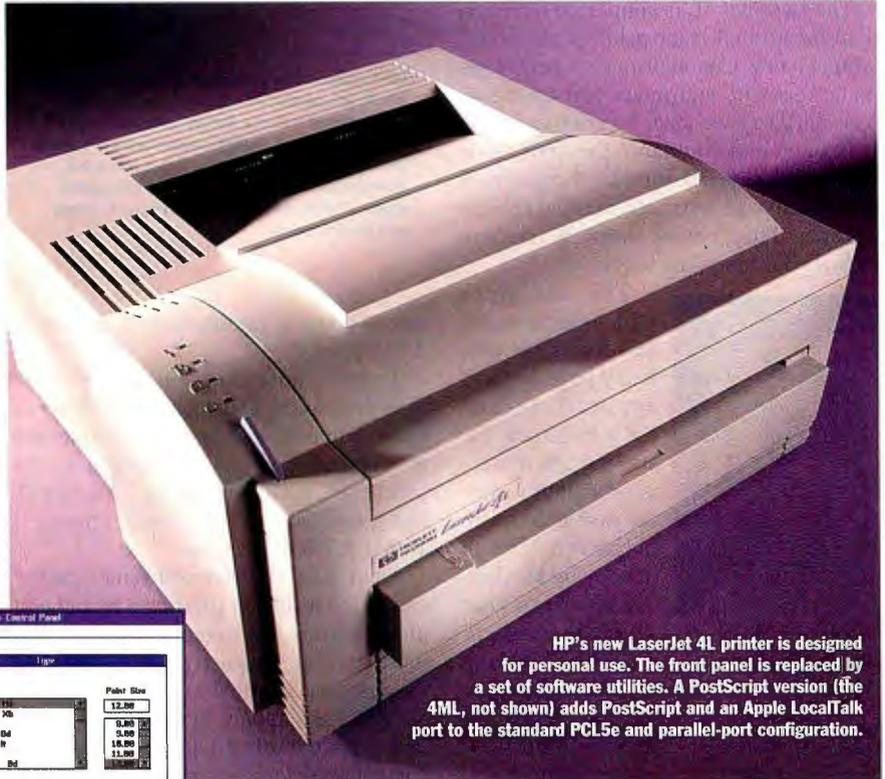
HP's new LaserJet 4L printer is designed for personal use. The front panel is replaced by a set of software utilities. A PostScript version (the 4ML, not shown) adds PostScript and an Apple LocalTalk port to the standard PCL5e and parallel-port configuration.
