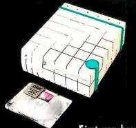
CAPACITY: 128 MB SIZE: 6.9" (H) x 2.7" (W) x 8.3" (D) WEIGHT: 4.11 LBS MOUNTING: VERTICAL OR HORIZONTAL
