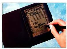
The Pen Pad weighs less than a pound and is solely penoperated, with no external (or emulated) keyboard option.
