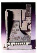
**ADJUSTABLE PAPER TRAYS are** common, but the mechanism on the 4L's single tray is unique. An adjustable ston on its single tray slides along a special track and locks in settings for 81/4- by 11-inch executive, and B5 sheets. The tray is sized for standard A4 paper, but it also prints envelopes, labels, and transparencies. To fit legal-size paper, the slide juts off the end of the tray, allowing the paper to stick out the back of the printer.
