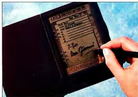
The Pen Pad weighs less than a pound and is solely pen-operated, with no external (or emulated) keyboard option.
