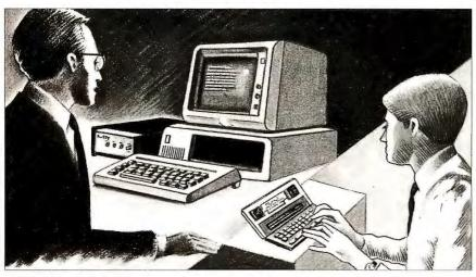
**This deaf user's PC** is connected to a telephone via an Ultratec Intele-Modem Baudot/ASCII modem. The user is sending and receiving messages to and from someone at a remote site who is using a telecommunications device for deaf people (right).
