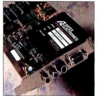
Antex SX-7 (\$995) from Antex Electronics (Gardena, CA) provides real-time direct-from-disk decoding of files recorded using Dolby AC-2 bit-rate reduction technique. The Windows 3.1-compatible board has playback sample rates up to 50 kHz.
