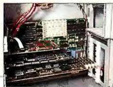
In addition to its pacesetter performance in our FoxPro and subsystem tests (see item above), the Thunderbox II can easily be expanded in the three areas vital to database and development performance: CPU, memory, and storage. The system contains a socket for upgrading to Pentium processors, disk cache that's expandable to 16 MB, and five available EISA slots.
