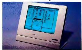
This 10" black on white monitor is easy-to-read, yet \$795 compact. Resolution is 640x480 for sharp, flicker-free image. Fast response, high refresh rate twisted nematic technology with backlighting provides a bright low radiation screen with a wide viewing angle. The adjustable monitor base is only 29x14 cm. It lets you mount the LCD monitor on vertical surfaces or fold for transport. Comes with 1.5 m cable and controller card. No external power required. IBM AT compatible.
