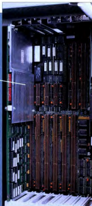
Acer took a unique approach to dissipating the heat generated by the Pentium in the AcerFrame 3000MP. A metal plate acts as a heat sink; it's thin enough to allow normal spacing of the expansion slots.
