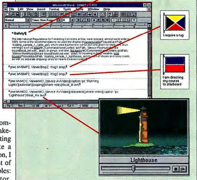
The Microsoft Word screen displays sample Viewer code. Clickable hot spots appear as underlined text in the resulting presentation. Multimedia links include sound, video, and embedded graphics. Notice the commands to place the flag bit maps and the MCI calls for playing sound and for displaying the lighthouse video.
