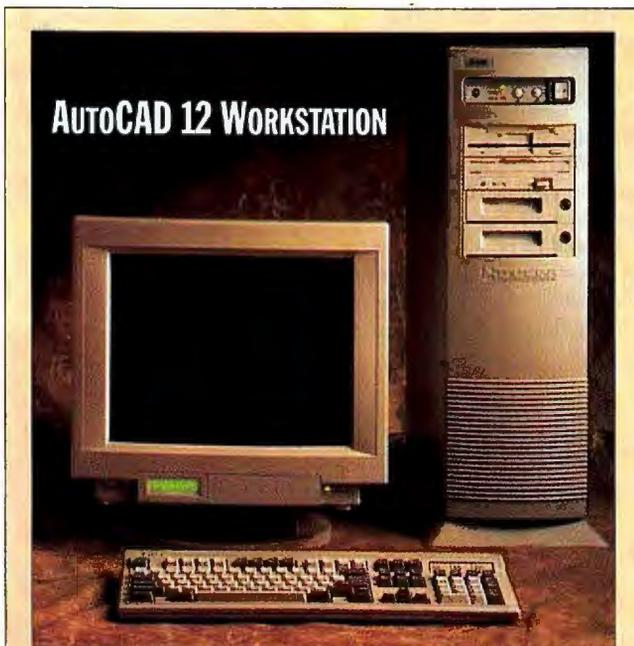
The new Tri-CAD 486 66-MHz VL-Station (from \$3595) targets the enhancements of AutoCAD release 12 for Windows. The workstation includes an IDE cache controller with 2 MB of RAM, a Weitek P9000-based VL-Bus accelerator with 2 MB of RAM, and support for noninterlaced resolutions of up to 1280 by 1024 pixels with 24 colors. The standard configuration includes 8 MB of RAM, a 340-MB hard drive, a 17-inch monitor, a 12- by 12-inch digitizer, and a cordless 16-button cursor.
