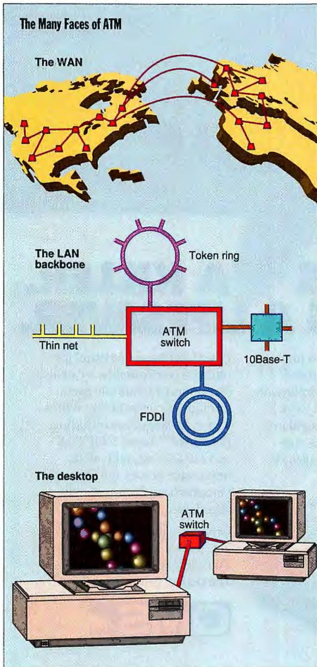
**What separates ATM from other networking technologies is its ability to scale from the desktop to the WAN to cable TV to voice networks. Its enormous throughput makes it a strong technology for implementing WANs, and its fast switching makes it ideal as a backbone for interconnecting LANs. It will even show up on some desktops, but only supporting the most data-intensive—and price-insensitive—applications.**
