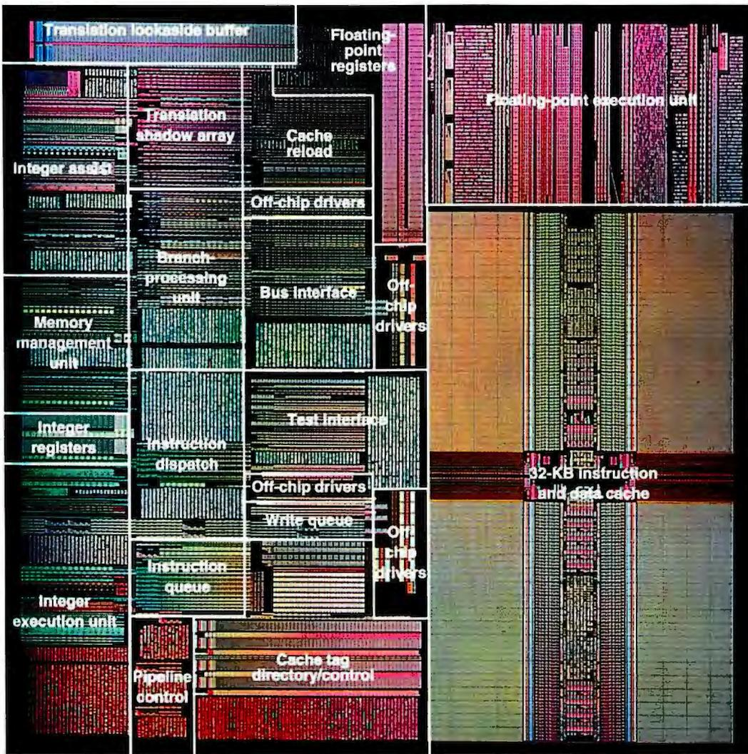
One way the PowerPC 601 conserves die area is to cluster its off-chip connection points in the interior of the die. This eliminates lines needed to move the connections to the periphery of the chip.
