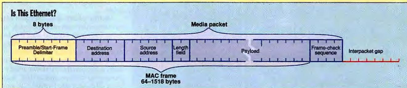
The Ethernet frame defines how Ethernet organizes the data in a packet. Hewlett-Packard and AT&T say that the frame defines Ethernet; Grand Junction Networks and its supporters say that the frame is necessary but not sufficient by itself.
