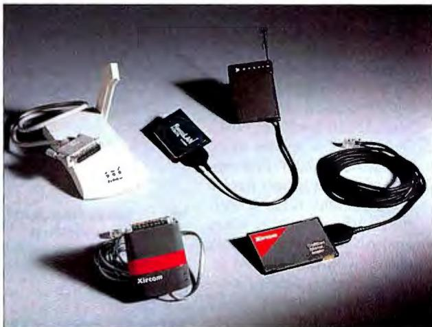
Xircom's PCMCIA and parallel port network adapters (shown at bottom) provide relatively painless network connections, provided you have an available cable nearby. Alps Electric's (top left) and Proxim's (top right) solutions are slower but solve the "last 500 feet" problem.
