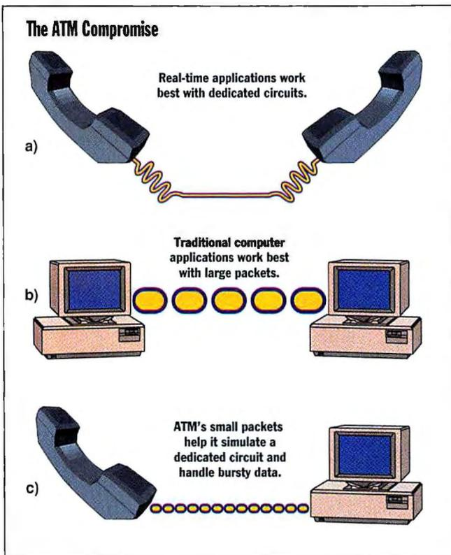
**ATM is not an ideal choice** for real-time applications like voice and video (a), or for data communications applications like file transfers (b). It is, however, the best technology on the horizon for combining both functions. Because of its fast, hardware-based switching, it can emulate the dedicated circuits usually required for real-time applications. And because it is packet-based, it can handle the bursty traffic characteristic of traditional data communications applications (c).
