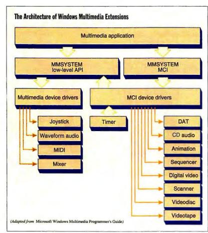
**Under Windows,** applications talk to MMSYSTEM, which invokes either a low-level multimedia device driver or an MCI driver, such as the sequencer. MCI drivers may either control the hardware directly or call on a multimedia device driver to control the hardware.
