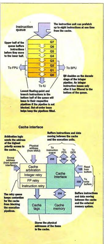
unit can fetch up to eight instructions from the cache during any one tick of the 601's master clock, meaning that the queue can go from empty to full in one clock cycle, assuming a cache hit.
