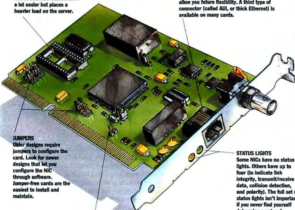
and-play: Intel's Ether Express Flash C, for example, comes with a program that automatically configures the card, finds a NetWare server, and downloads drivers from the server. At the other end of the spectrum were cards like the CNet CN650E+, which came with a one-page manual and no drivers or diagnostics.
