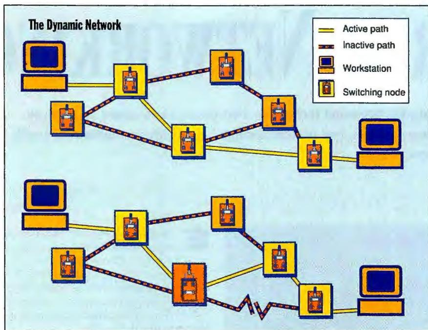
Like other switching technologies, such as X.25 and voice telephony, ATM networks consist of switches located at communications nodes. If a communications link fails, the network can dynamically reroute traffic to bypass the fault and maintain communications.
