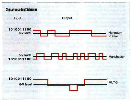
The way a signaling scheme represents strings of bits determines the electrical characteristics of a network. Although complex signaling schemes (e.g., MLT-3) have greater processing overhead, they can reduce electrical noise by decreasing the voltage changes necessary to transmit a signal.
