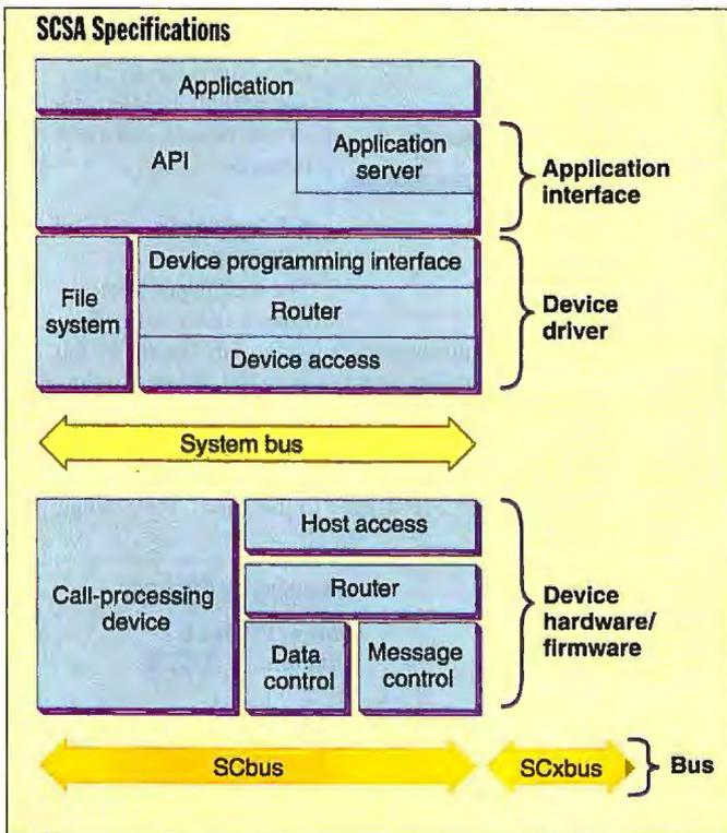
Dialogic's SCSA takes a layered approach to integrating telephony with computer applications. At the top of the stack are applications that access a standard API set. Applications—and applications developers—are freed from dealing with the complexities of device drivers, call-processing hardware, or interfaces to telephone lines.
