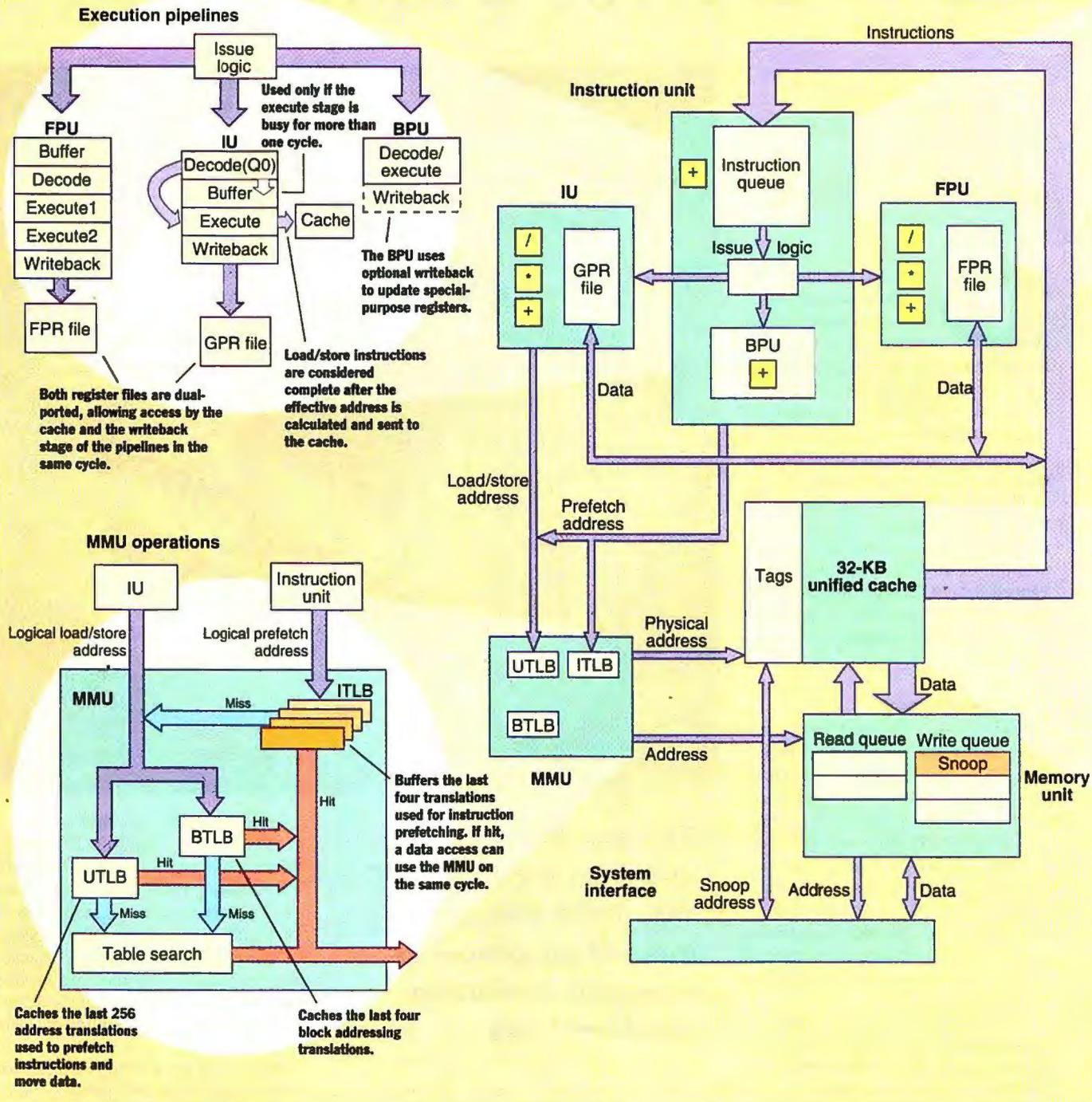
To achieve optimal performance, the MPC601 must keep its three execution units busy. This task falls primarily to the instruction unit, which fetches instructions from the internal cache and issues them to the individual execution pipelines.
