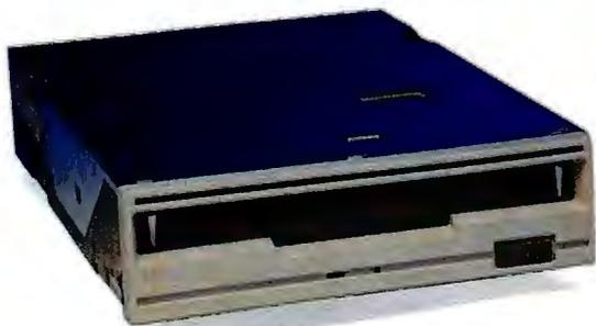
You've been waiting for a powerful optical storage drive that slides easily into any standard half-height computer bay. And Pioneer engineers did it. Presenting the **world's first** 5¼" half-height multifunction (rewritable/WORM) drive. *The DE-UH7101.*
