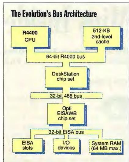
**The Evolution's motherboard** is home for three buses. A 64-bit-wide R4000 bus connects the CPU to a secondary cache; a 486 bus serves as the interface between the R4000 and PC peripherals; and an EISA bus provides expansion. A DeskStation Technology custom chip set links the R4000 to secondary cache and to the 486 bus, while an Opti chip set links the 486 bus to EISA. System memory hangs off the EISA bus.
