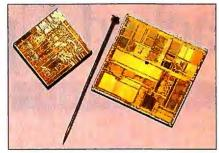
The MPC601 (left) is a much smaller chip than the Pentium due to several factors: It uses a 0.65-micron, four-layer metal CMOS process to pack 2.8 million transistors onto a die only 11 mm square. Intel's 0.8micron three-layer metal BiCMOS technology limits the Pentium's 3.1 million transistors to a die that's 16.6 by 17.6 mm in size. The MPC601's smaller die helps reduce the cost of its manufacture.
