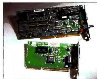
NICs built from one or two chips (bottom) allow for smaller physical designs with no performance change.
