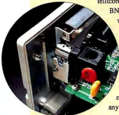
Compaq Deskpro 4/66i to insert the card for testing. Although this was the worst case, we found similar problems with other cards—BNC connectors were too high or too low. If your system is tightly packed, you may not be able to connect the BNC T-adapter at all.
