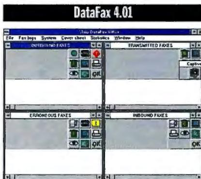
**T**rio Information Systems' DataFax is composed of five modules. Winserve, the main module, controls the modem and manages the fax traffic. Faxes are either sent in the background or, if Winserve is not running, stored in an outbound queue.
