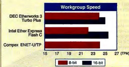
Eight-bit NICs are faster at 8-bit operations than dual 8- and 16-bit cards.
