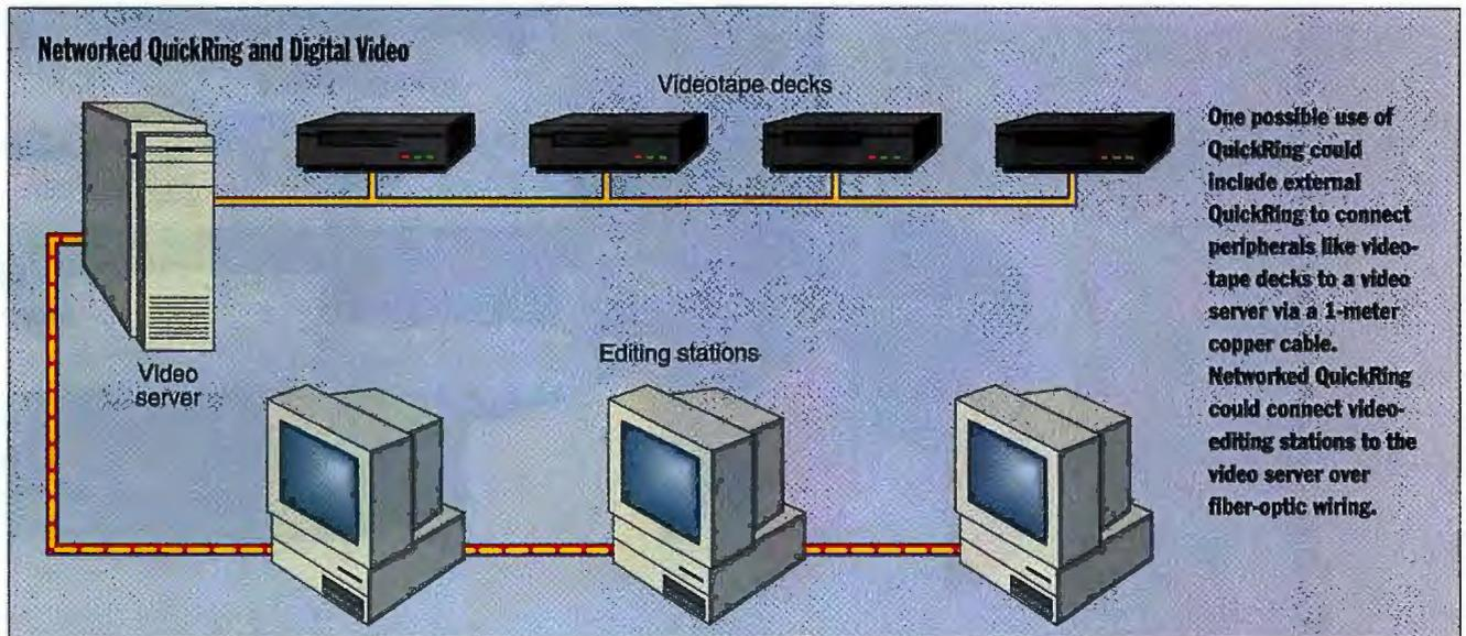
One possible use of QuickRing could include external QuickRing to connect peripherals like videotape decks to a video server via a 1-meter copper cable. Networked QuickRing could connect video-editing stations to the video server over fiber-optic wiring.
