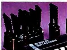
**But if you insist on using jumpers,** then those on the Complex ENET-U/TP are the easiest to use. Unlike standard jumpers, those on the ENET-U/TP have attached flags. You may need pliers to pull out and reinsert standard jumpers when they are (as is usually the case) very close together. The extensions on the ENET-U/TP's jumpers made them easy to grab and reinsert. Although it's not something you do too often, when it comes to manual setup, every little bit helps.
