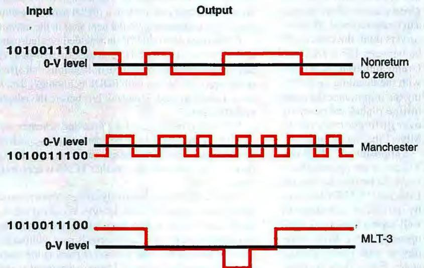
The way a signaling scheme represents strings of bits determines the electrical characteristics of a network. Although complex signaling schemes (e.g., MLT-3) have greater processing overhead, they can reduce electrical noise by decreasing the voltage changes necessary to transmit a signal.
