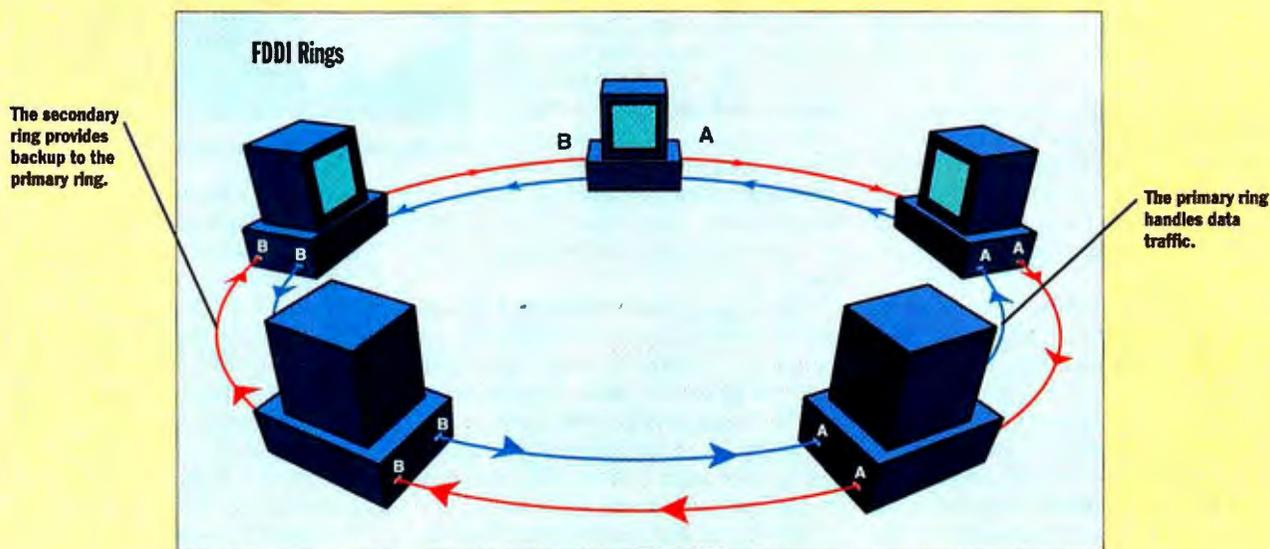
Each station on an FDDI network requires connections to both fiber-optic rings, with the primary ring handling data transmission and the secondary one providing fault tolerance and system management.
