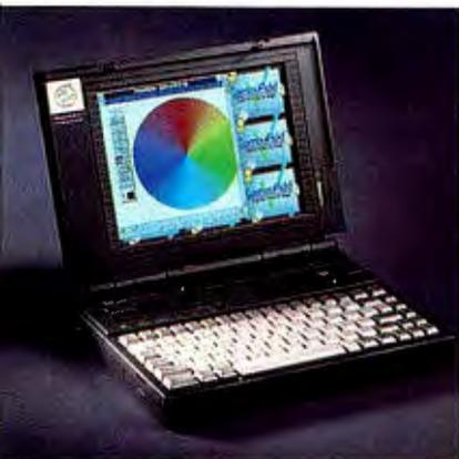
pound notebook includes a 200-MB hard drive, an internal fax modem, 4 MB of RAM, 512 KB of video memory, a PCMCIA slot, and a built-in trackball.
