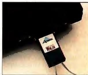
many as 250 PCs up to 600 feet away via the adapter's two RJ-11 jacks. Included are a 25-foot phone cable and a driver disk.
