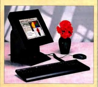
A 64,000-color active-matrix thin-film-transistor flat-panel display is standard with the APF4000 Series (from \$5995) of 66-MHz 486DX2 desktop computer systems. Included are VESA Local Bus video, a 170-MB hard drive, a 1.44-MB floppy drive, and a PCMCIA Type II slot. Consuming less than 50 W, the APF4000 has no cooling fan, which means quiet operation. The diminutive system measures 9 by 10 inches and weighs 14 pounds. Ethernet and Token Ring interfaces are available.
