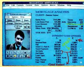
A Cadillac among desktop video and document conferencing systems, NCR's TeleMedia Connection is a hardware and software package that supports collaborative document mark-up and real-time video-in-a-window. It uses H.261-standard compression and requires dual ISDN channels for quarter-screen video throughput of 15 fps.
