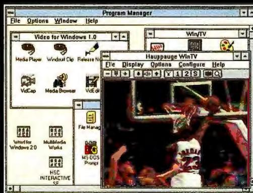
Resize or reposition your Win/TV window anywhere on the screen. The "always-in-front" mode allows the video image to always be viewable.
