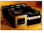
that fits more controller electronics onto the board by wrapping the flexible printed circuit board around the drive mechanics. (This same technology is often found in notebook computers.)
