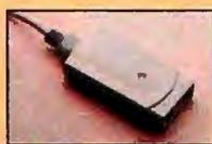
The Apple PlainTalk microphone is designed to focus on an area 18 to 30 inches in front of it to help eliminate background noise.
