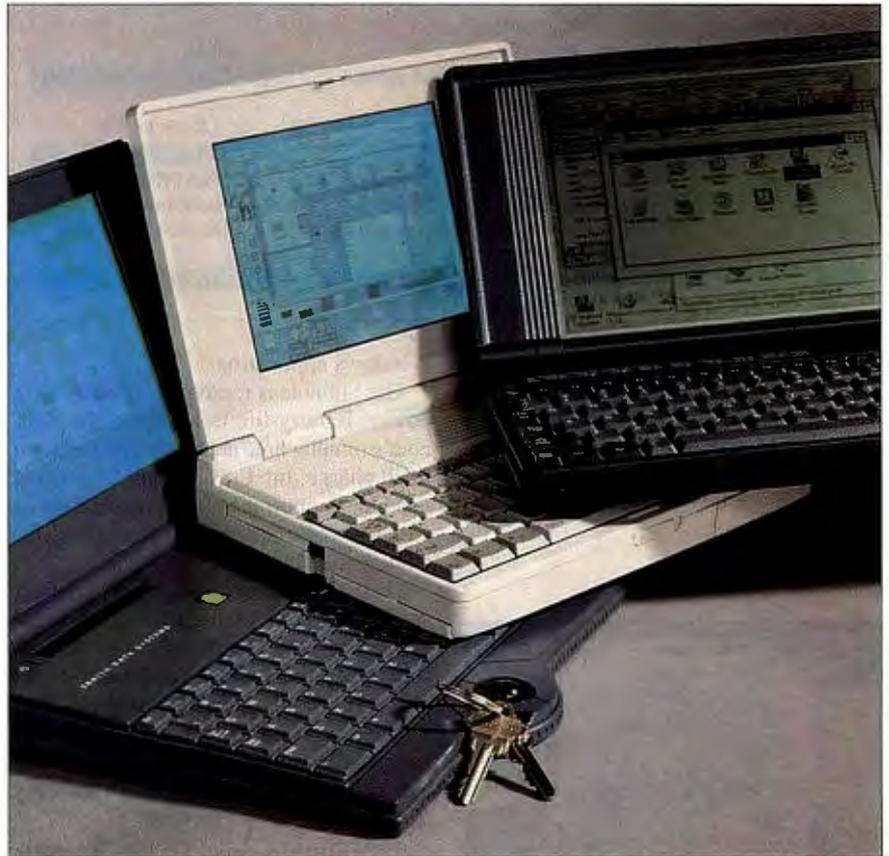
**New subnotebooks** from ZDS, CompUSA, and HP (left to right). HP easily captures the title of "most portable," weighing in at just under 3 pounds and with a profile smaller than that of most three-ring binders. However, CompUSA's Subnote packs quite a bit more processing power, and both the Subnote and ZDS's Z-Lite make fewer compromises for portability.
