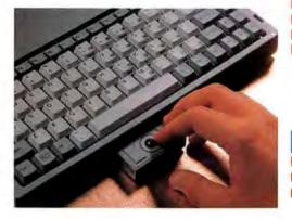
The integrated track ball slides out from a compartment by the space bar on the keyboard. You simply pull it out and go to work. Finished? Just slide the track ball back into the ColorBook.
