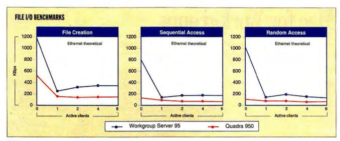
File I/O benchmarks for the Workgroup Server 95 and the Quadra 950. The Workgroup Server had a 500-MB hard drive and 16 MB of RAM to the Quadra's 230-MB hard drive and 12 MB of RAM. The figure shows aggregate network throughput while creating files and during sequential and random access. The Workgroup Server maintains a high network throughput at up to six highly active clients, although, of course, still well below theoretical Ethernet bandwidth.
