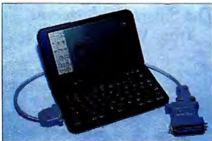
RS-232 converter cable and a self-power serial-to-parallel converter. The Serial Kit has the serial cable converter and a null modem adapter.
