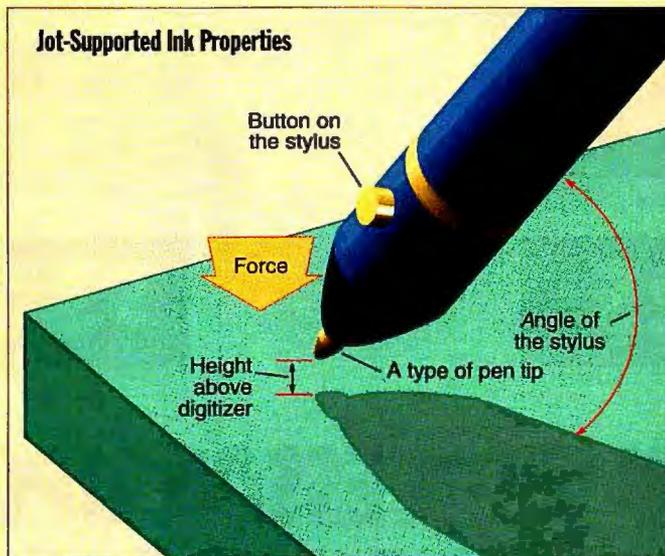
**Jot captures a surprising number of ink properties**, in addition to the coordinates of the path the pen takes, and stores them in an application-specific record. Besides the properties shown in the figure, Jot supports multiple strokes of ink combined into single objects, bounds, scale, offset, numbered groupings of strokes, color and opacity, and timing information.
