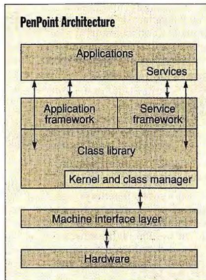
PenPoint, like Newton Intelligence, is object-oriented, but it maintains ties to a file-based structure.
