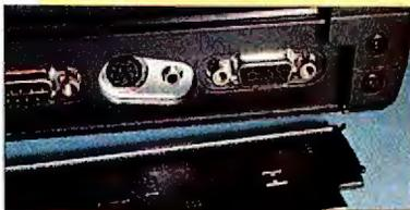
**Snap! Flimsy hinge pins** on the Compaq Contura's port-cover plate break off with the slightest provocation. Thicker pins proved sturdier, but the best solution was the Toshiba Satellite's, with sliding doors covering its ports. Note that this problem is not restricted to Compaq; other vendors, including Twinhead and Texas Instruments, are equally guilty.
