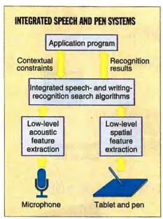
Speech and writing recognition in computers of the future will be integrated above the lowlevel feature extraction stage, enabling both input signals to be jointly decoded into a single recognition result that is consistent with the current context set by the application program.
