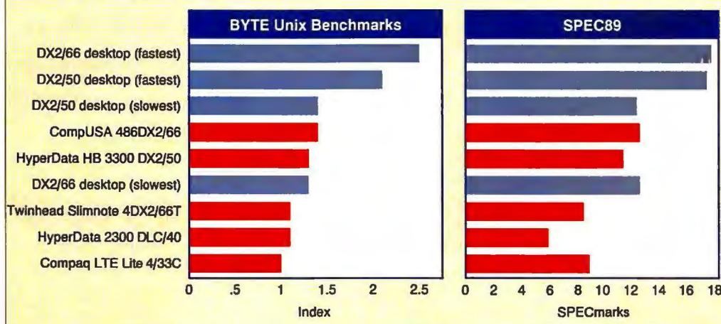
Although adequate for some Unix applications, 486-based notebooks lag in Unix performance compared to desktop 486-based systems.
