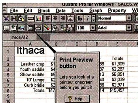
When you point at a control in one of the SpeedBars and click on the right mouse button while holding down the Control key, QP5W rewards you with an Object Help box. If the information in the box doesn't satisfy you, you can click on the box's help button for more details.
