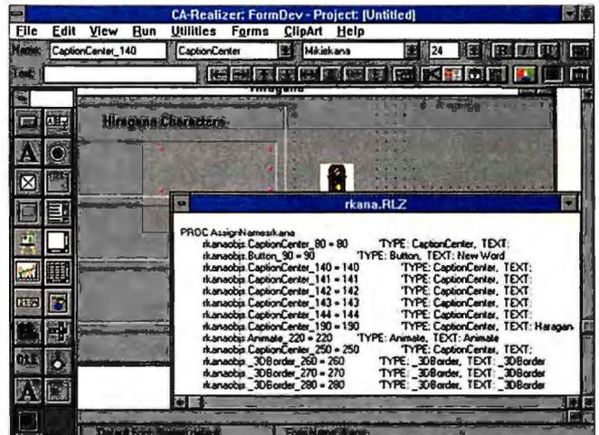
CA-Realizer 2.0's application screen and the underlying code generated by FormDev. This code is called from the main project program to display the screen at run time. The form code is a procedure function written in Realizer BASIC.
