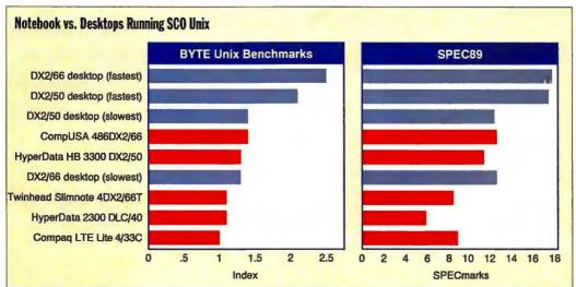
Although adequate for some Unix applications, 486-based notebooks lag in Unix performance compared to desktop 486-based systems.
