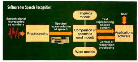
Speech-recognition software first converts the speech into its frequency components. It then uses stored models of expected word order to make a good guess as to what was said. The applications software can then display the text or take an action consistent with what was said.
