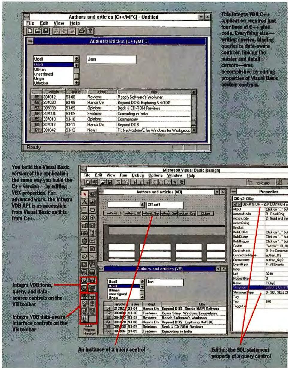
This Integra VDB C++ application required just four lines of C++ glue code. Everything else—writing queries, binding queries to data-aware controls, linking the master and detail cursors—was accomplished by editing properties of Visual Basic custom controls.
