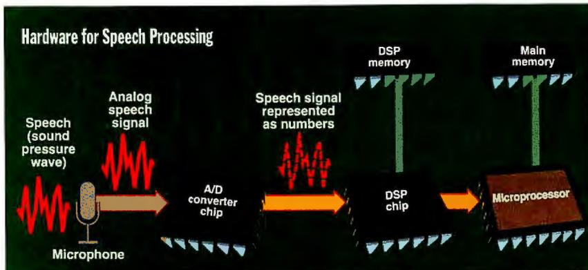
The speech-recognition hardware must convert the analog speech into digital form. Once in digital form, the speech is data that a DSP, a microprocessor, or both can process.
