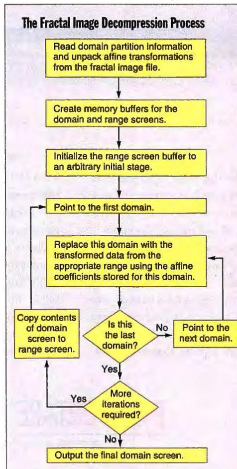
The algorithm to decompress an image stored as fractal-transform data.
