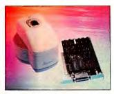
Startek's fingerprint identification system connects to a PC through the AT-bus card. The red LED fingerprint reader is at the top left.
