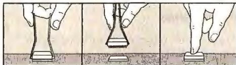
*Talk about immediate gratification. Just use the chip removal tool provided to pull out your 386DX chip (16, 20, and 25 MHz versions only at the moment), and plug our Cyrix Upgrade Microprocessor into the empty socket. Then get ready for screaming 486 power.*
