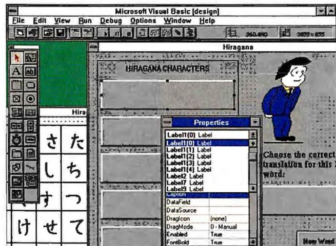
The development of the hiragana screen using Visual Basic 3.0. The five label objects, used to display the Japanese words, are set up in a control array for easier program handling. VB will ask if you want an array when you copy and paste multiple objects or give two similar objects the same name.
