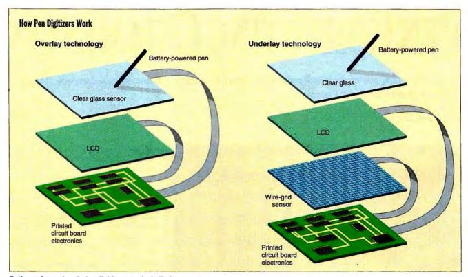
Both overlay and underlay digitizers work similarly. First, the pen interrupts a sensor field, sending an analog signal of the x, y coordinates to the system. The system translates the signal from analog to digital and lights the appropriate pixel.
