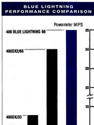
All processors were tested on the same IBM motherboard.
