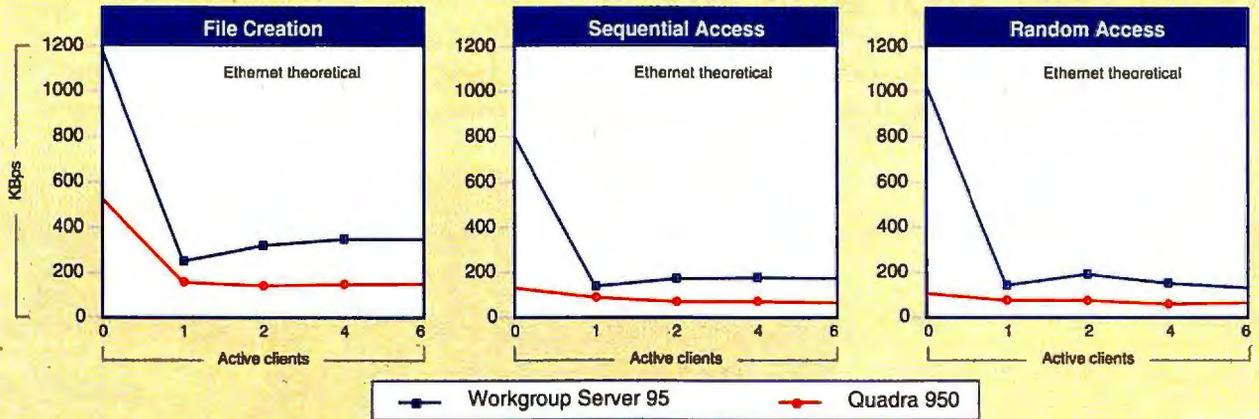
File I/O benchmarks for the Workgroup Server 95 and the Quadra 950. The Workgroup Server had a 500-MB hard drive and 16 MB of RAM to the Quadra's 230-MB hard drive and 12 MB of RAM. The figure shows aggregate network throughput while creating files and during sequential and random access. The Workgroup Server maintains a high network throughput at up to six highly active clients, although, of course, still well below theoretical Ethernet bandwidth.
