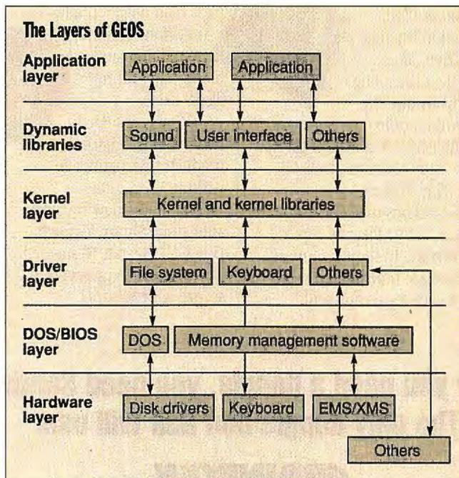
The GEOS operating system is based on the familiar DOS architecture, but it does make use of some high-level objects for the sake of reducing code requirements for programmers.
