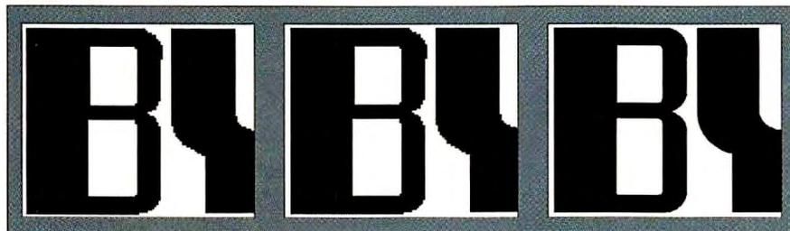
**Common Ground (left) and Acrobat Exchange (middle)** create electronic documents by servicing print calls from the application. Using this method, both technologies process the low-resolution preview image of an embedded EPS graphic. Acrobat Distiller converts EPS files directly, resulting in much higher-quality output (right).
