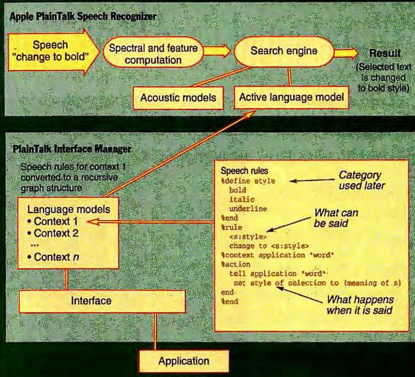
Apple's PlainTalk speech-recognition software allows continuous speech for command and data entry. An applications developer can use data structures called "speech rules" to define what speech the systems will understand in specific contexts (e.g., within a specific application). The resulting action is also specified within the rule.
