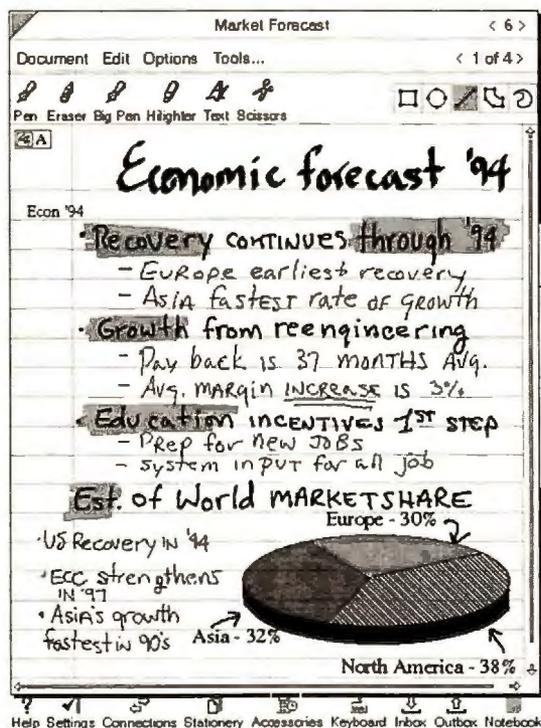
Ink Development's Notetaker captures, indexes, and manipulates digital ink. It can highlight or boldface handwritten text. You decide when to recognize handwritten text.
