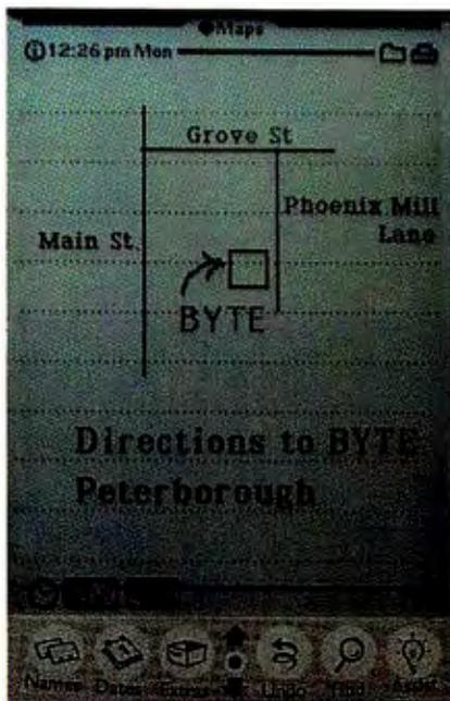
The MessagePad features a row of "hard icons" at the bottom of the screen that provide access to frequently used functions.
