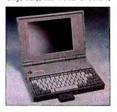
an 80- or 170-MB hard drive, an integrated trackball, and a PCM-CIA Type III slot.
