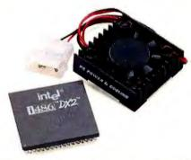
It's a fact. 486 chips run hot, often exceeding 185°F! Now, you can cool your 486 to a safe 85°-95°F with our popular CPU-Cool. It prevents random system errors and other heat-related problems. Consists of a mini-fan embedded in a sculptured heat sink that easily mounts on the CPU. Powered by a spare drive connector. Effective, inexpensive insurance!
