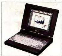
communication modules that support LANs and WANs (widearea networks), including wireless cellular data. With an AudioDrive multimedia chip, the Inex Technologies (Santa Clara, CA) notebooks provide the means for audio presentations, vocal script, and voice E-mail. The units support up to 20 MB of main memory and up to 200 MB of storage on the removable hard drives. The LCD screen is also upgradable.
