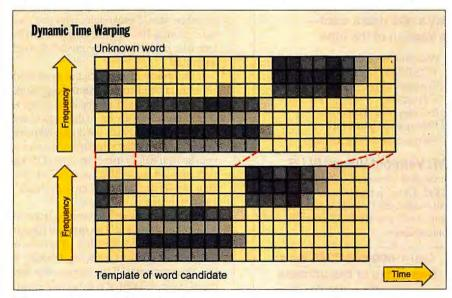
When an unknown word is spoken, it is compared to stored templates (i.e., frequency time pictures) of each word to get the best match. Dynamic time warping allows a match to be made so that the best-matching parts of each word align, making the match less sensitive to the speed of speaking.
