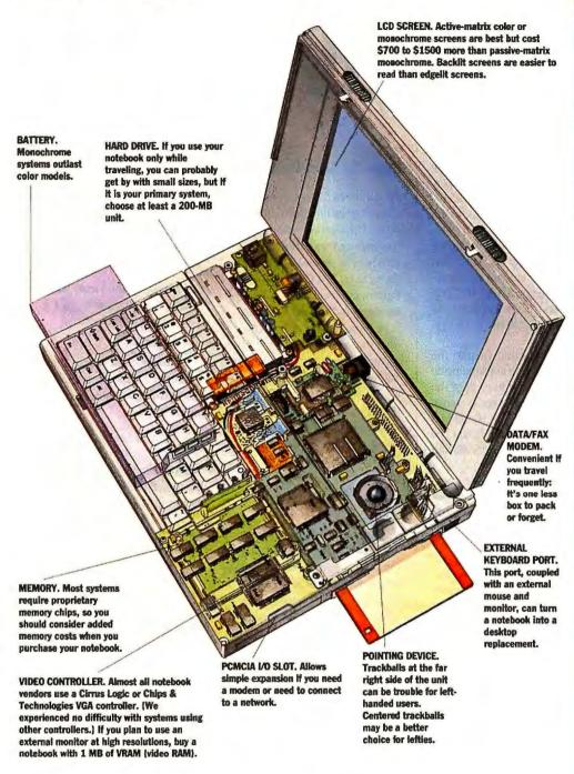
**EXTERNAL VIDEO CONNECTOR. Most** notebook LCD screens handle a resolution of only 640 by 480 pixels. Make sure your notebook's VGA controller can handle up to 1024 by 768 pixels on the external port if you want to use an external monitor.
