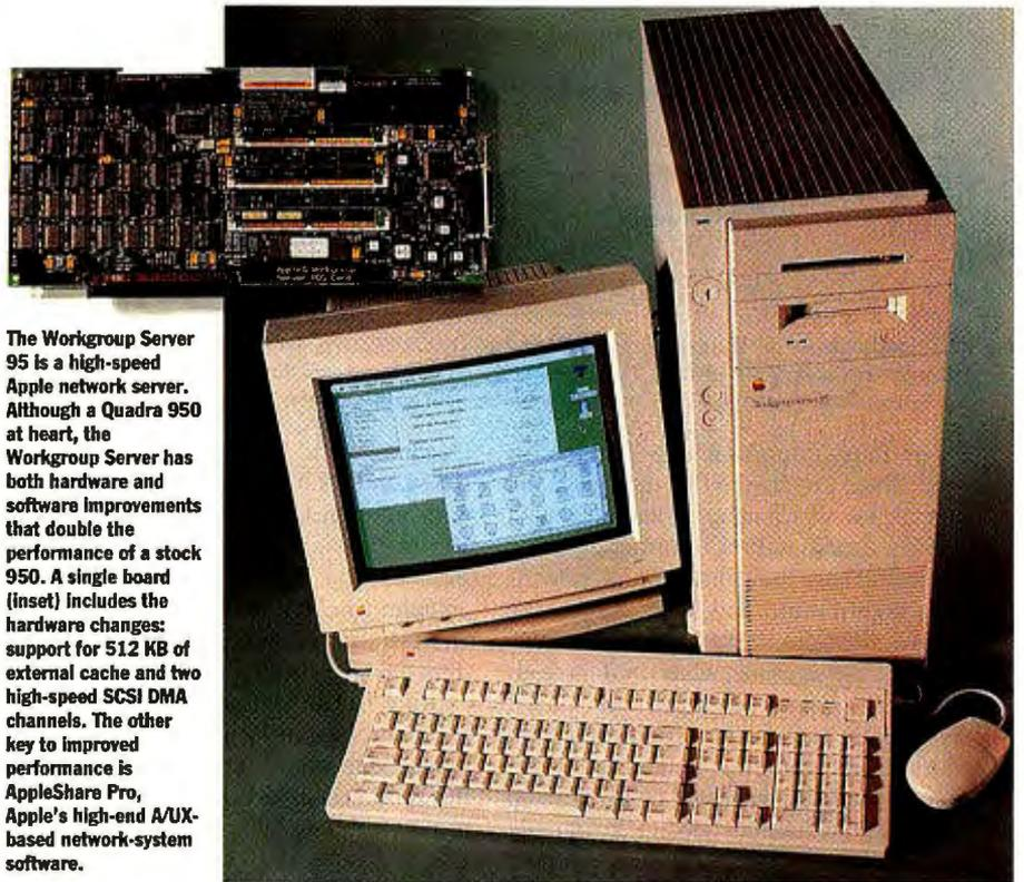
The Workgroup Server 95 is a high-speed Apple network server. Although a Quadra 950 at heart, the Workgroup Server has both hardware and software improvements that double the performance of a stock 950. A single board (inset) includes the hardware changes: support for 512 KB of external cache and two high-speed SCSI DMA channels. The other key to improved performance is AppleShare Pro, Apple's high-end A/UX-based network-system software.
