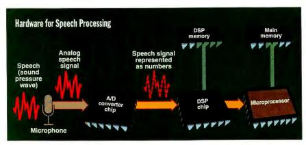
The speech-recognition hardware must convert the analog speech into digital form. Once in digital form, the speech is data that a DSP, a microprocessor, or both can process.
