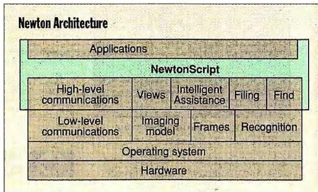
Newton Intelligence is object-oriented from the ground up. Most programmers will access MessagePad resources and write applications using NewtonScript.
