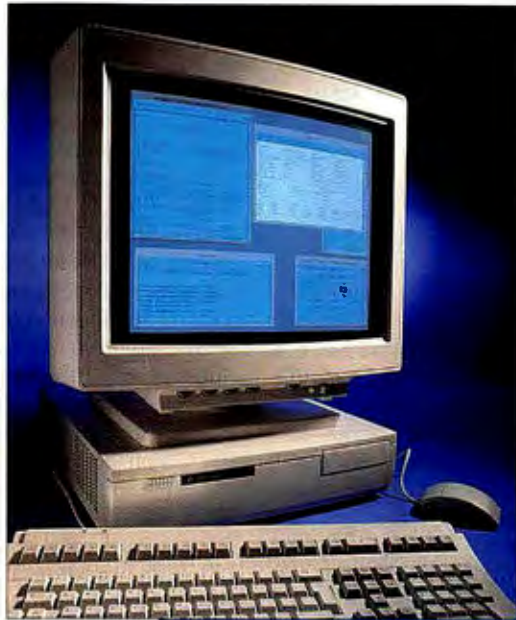
The first Alpha PCs from DEC: the DEC 3000 Model 300 (left), a powerful Unix box, and the DECpc AXP 150, an EISA server that runs NT.
