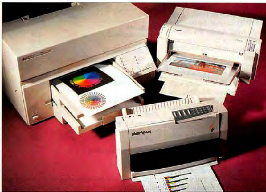
Clockwise from foreground: Inexpensive color printers from Star Micronics, Hewlett-Packard, and Fargo. Star Micronics' SJ-144 and Fargo's Primera break the $1000 price barrier for thermal-transfer color printing by leaving the image processing to the host system. With its photo-realistic upgrade, the Primera is the least expensive dye-sublimation printer by far.
