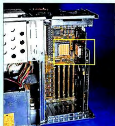
The motherboard holds a 486DX2; an optional card holds a second matching CPU (two chips outlined).
