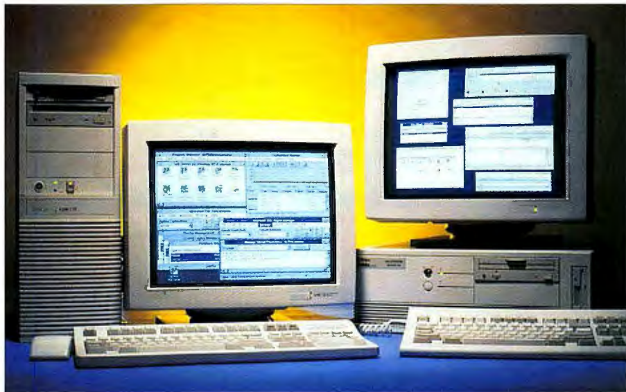
One of NT's strengths is its ability to run on RISC-based hardware such as the Alpha-based DEC AXP 150 and the R4400-based SGI/Mips Magnum.
