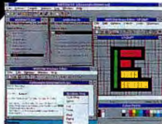
Watcom C/C++ 10.0 includes a programmer's editor with syntax highlighting, a suite of resource editors and application testing and monitoring tools for Windows 3.x and Windows NT development.
