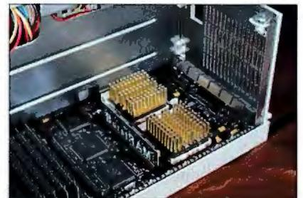
With the power supply up, memory and CPUs (two here) are easily accessible.
