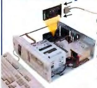
**PEL 1640** 16 BIT SCSI adapter, internal 50-pin & floppy ribbon cable, adds a BIOS and support for up to two 3.5 and/or 5.25 floppy drives. \$132.00
