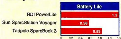
Results are in hours. The PowerLite is the best choice for running without AC power, as its 1.2-hour battery life (measured by BYTE's Thumper) attests. But compared to more common Intel-based notebook PCs, which average 2.5 hours of battery life on this test, all these systems are far behind. Battery life is limited enough, even for the PowerLite, that I wouldn't consider using any of these systems without access to AC power.
