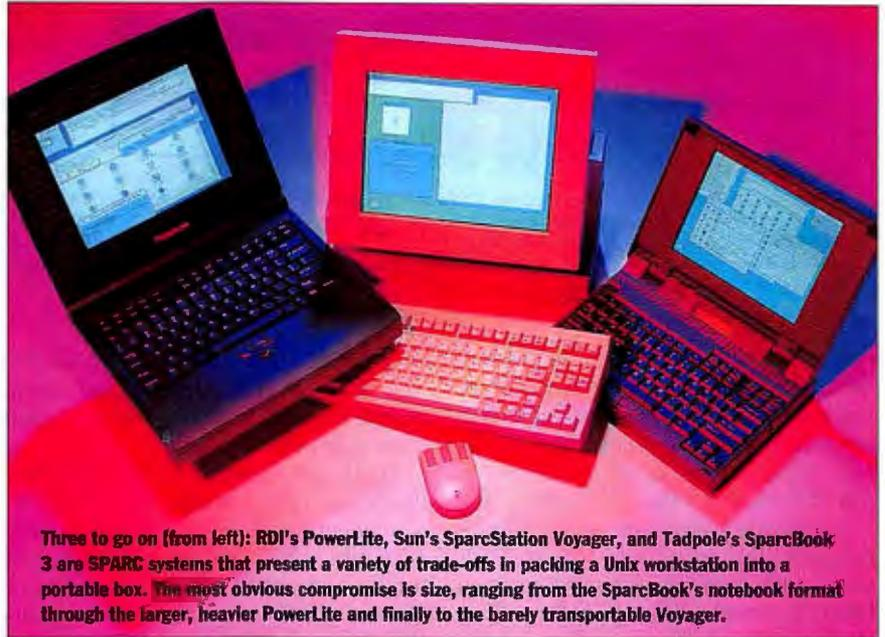
Three to go on (from left): RDI's PowerLite, Sun's SparcStation Voyager, and Tadpole's SparcBook 3 are SPARC systems that present a variety of trade-offs in packing a Unix workstation into a portable box. The most obvious compromise is size, ranging from the SparcBook's notebook format through the larger, heavier PowerLite and finally to the barely transportable Voyager.
