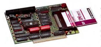
Quatech's I/O cards are available in RS-232. RS-422 and RS-485. Each are PCMCIA PC Card 2.1 compliant and support "hot-swapping" (insertion and removal of card while system is on). Quatech also offers a single port IBM PC compatible Enhanced Parallel Port PCMCIA card and a 24 digital input/output Type II PCMCIA card.
