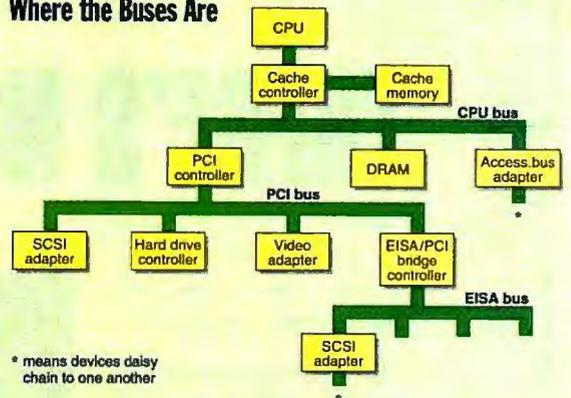
Not only do buses attach to computer systems, they can attach to one another, creating a hierarchical series of slots where different peripherals can be attached. This figure shows one possible configuration.
