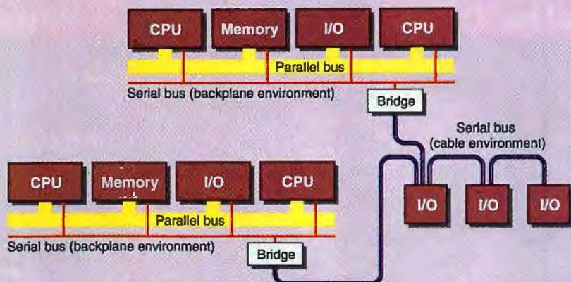
More than one computer can be connected to the P1394 (or FireWire) bus. Each device on the bus has a port with terminators, transceivers, and logic. The cable and ports act as bus repeaters between the nodes to simulate a single logical bus.
