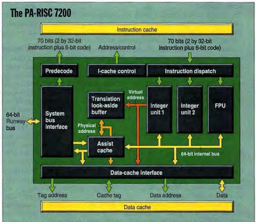
Unique in a number of ways, the PA-RISC architecture is best exemplified by its use of off-chip primary instruction and data caches. It integrates 1.3 million transistors onto a 210-mm<sup>2</sup> die.
