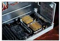
With the power supply up, memory and CPUs (two here) are easily accessible.
