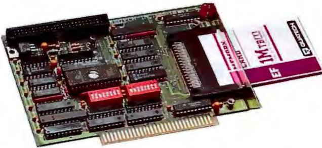
The PCMCIA standard allows the information gathered via laptop, PDA, palmtop, or pen-based systems to be compatible with desktop PC's. Quatech manufactures a full line of products that conform to the PCMCIA standards including Type I card readers for memory cards, Type II and III interface adapters, and I/O cards for communications and data acquisition applications.
