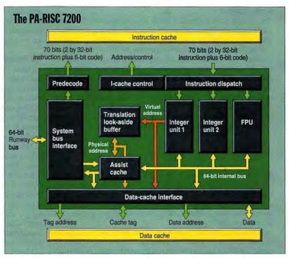
A splendid sentiment, and one that can't Unique in a number of ways, the PA-RISC architecture is best exemplified by its use of off-chip primary instruction and data caches. It integrates 1.3 million transistors onto a 210-mm<sup>2</sup> die.
