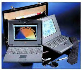
The 500 series PowerBooks (left) provide a much-needed overhaut for the alin-one design. Improvements include storage and RAM capacity, built-in Ethernet support, an innovative trackpad, stereo sound, a PCMCIA Expansion Module, and a 68040 processor upgradable to PowerPC. The Duo 280 systems (right) bring the might of the 68040 processor to the PowerBook Duo line.
