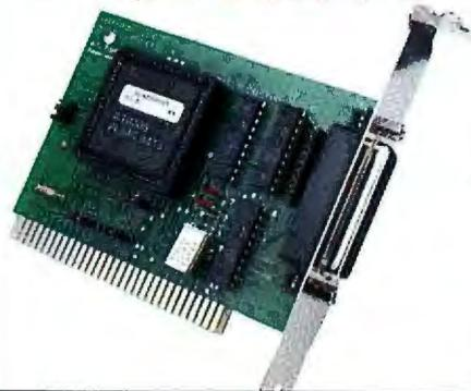
Plug the BuffPort™ into your PC and print to any parallel printer or device. Transfer data from your PC as fast as the printer can accept it, up to 150,000 cps. (A standard PC parallel port is typically limited to about 10,000 cps.) Use the BuffPort with the HWP for a 150,000 cps printer sharing system!
