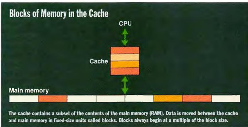
The cache contains a subset of the contents of the main memory (RAM). Data is moved between the cache and main memory in fixed-size units called blocks. Blocks always begin at a multiple of the block size.
