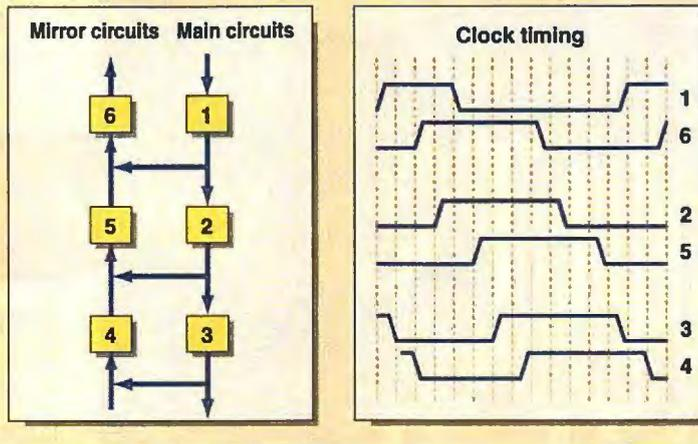
With split-level charge recovery, circuits are paired with their inverse circuits (1 with 6; 2 with 5; 3 with 4). The results of the main circuit chain are passed to the mirror-image chain, thus preserving the results and the energy used to generate them. The timing diagram shows how the clocks that drive the circuits must cascade so that the system uses as little power to switch as possible.
