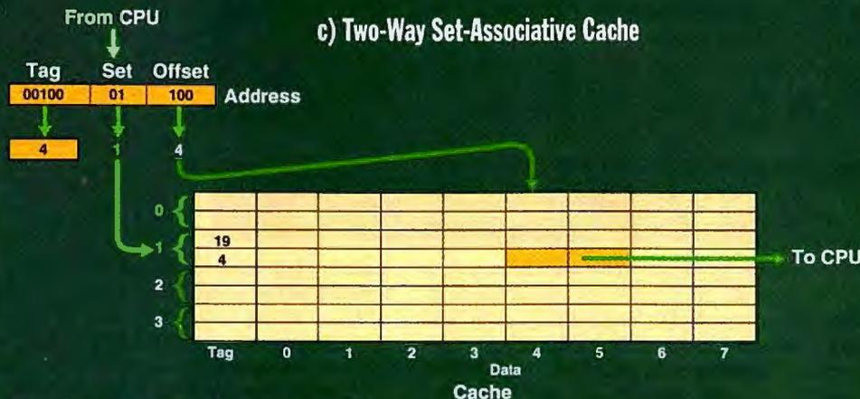
For purposes of illustration, this figure uses a 10-bit address, an eight-line cache, and an 8-byte line size.
