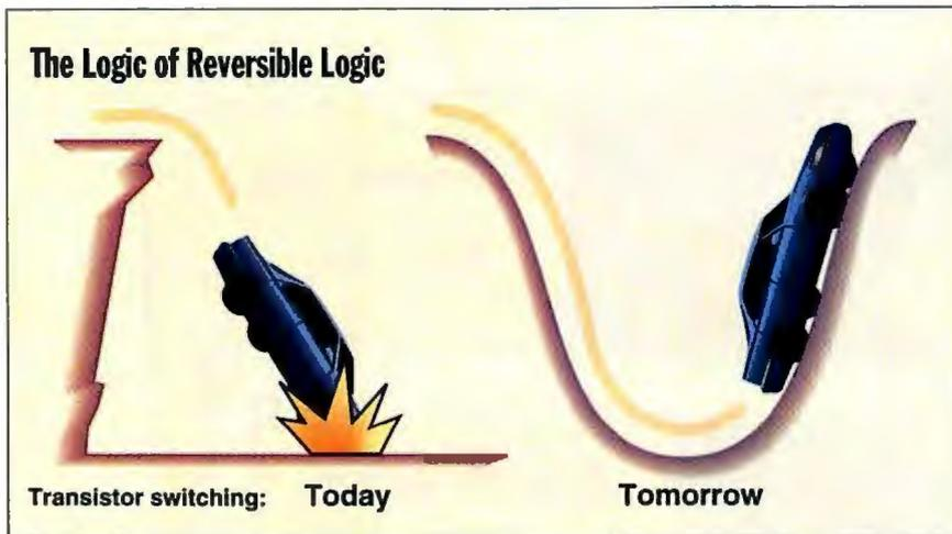
Chips today consume so much power because of the way in which transistors switch on and off. When a transistor switches from a high-logic state to a low-logic state, all the energy required to get to the high state is dissipated, just like a car going over a cliff dissipates its potential energy at impact. Reversible logic aims to conserve the energy so that it can be used to switch again.
