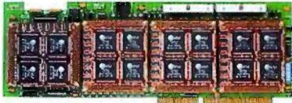
MB of DRAM. The board implements 16 concurrent V.32bis modems and supports up to 512 concurrent phone conversations. Bundled software includes the VCOS real-time multitasking operating system and a set of multimedia and telephony modules.
