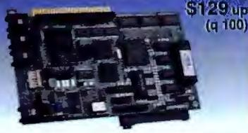
**Use 'C' code** KS-2: XT equivalent card with NEC V40, 256k RAM \$149(q1) Options; PCMCIA, 1M Ram/Rom/Sram, 3sr1., par, modem, A/D.
