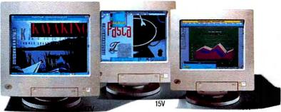
actual viewable screen size of 15.8, 13.7, and 13 inches, respectively, when measured diagonally.
