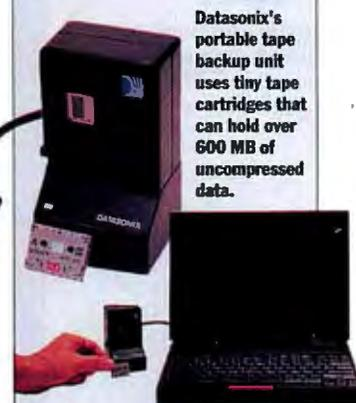
Data-sonix's portable tape backup unit uses tiny tape cartridges that can hold over 600 MB of uncompressed data.
