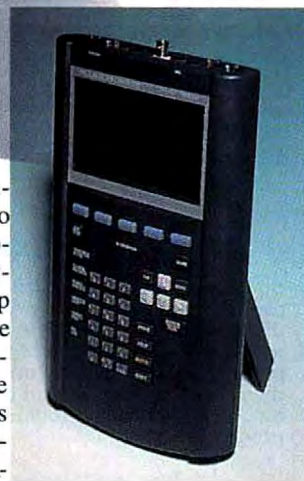
Fluke crams a useful mix of LAN-testing functions into the LANMeter's rugged 4½-pound, 11½-by 6½-by 2½-inch package. Batteries last up to 3 hours if you don't use the screen backlighting. Five keys located below the LCD display take on the functions displayed on the screen above (inset).
