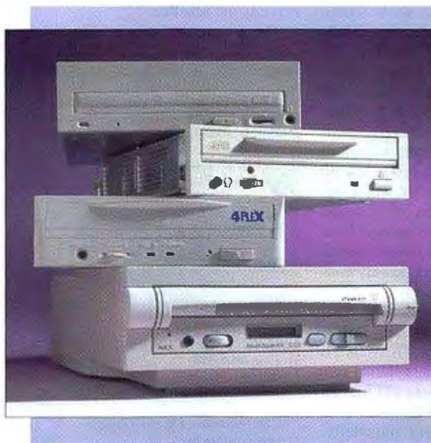
A stack of four quad-speed CD-ROM drives (from top to bottom): TEAC America's SuperQuad, Toshiba's XM-3501B, Plextor's 4Plex, and NEC Technologies' MultiSpin 4Xe. List prices with host adapter range between $549 and $645. The TEAC drive uses a proprietary AT interface compatible with some Sound Blaster cards; the other three are SCSI drives. The NEC is an external unit (internal also available); the others are internal. The Plextor and Toshiba drives provided the best performance.
