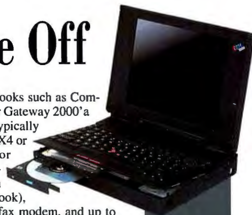
The IBM ThinkPad 755CD's lift-up keyboard lets you remove the CD-ROM drive and install a removable disk drive or a PCMCIA cartridge to add an additional card slot.
