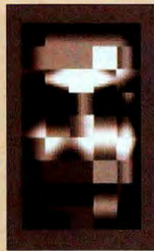
In addition to accuracy, Photobook's eigenface model is also an efficient way to store images. The eigenface image on the left requires only 85 bytes of storage space; the murkier image on the right is a JPEG-compressed version of the original that requires 540 bytes of storage.
