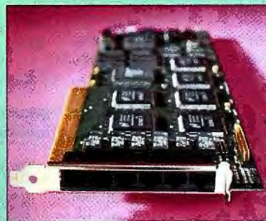
The server-based XNET Series 1800 ParallelSwitch is a store-and-forward switch with a RISC processor, six full-bandwidth Ethernet ports, and an address capacity of 8000.
