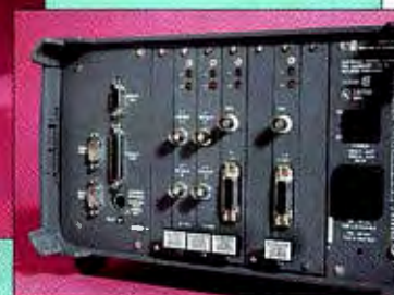
The DA-30 protocol analyzer captures and generates network traffic.
