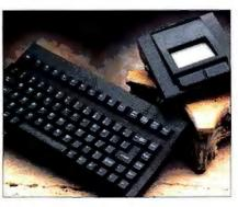
83-key keyboard, a mouse touchpad pointing device, and an RF transmitter/receiver. The touchpad allows fast and accurate movement of the screen cursor as you simply glide your finger over its 2- by 3-inch surface. Contact: Wireless Computing, Irving, TX, (214) 719-2515. Circle 999 on Inquiry Card.
