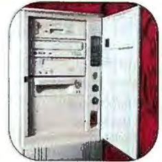
The Gateway P5-120XL comes with a quad-speed CD changer that lets you load up to three CDs into the unit and switch among them without handling them. The CD changer supports multisession Kodak Photo CDs as well as XA (Extended Architecture) format and includes a headphone jack, volume control, play/pause controls, and a skip function. CD-ROMs are becoming a necessity on file servers for loading system software and utilities.
