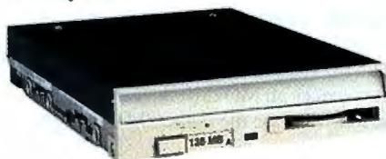
The Zip comes in two interface versions, as either a SCSI or parallel unit. The SCSI version includes both PC and Mac software. (If your PC does not have a SCSI adapter, Iomega sells one for \$149.95.) Easy-to-use switches on the back of the SCSI drive set SCSI ID and termination settings. For PC users, the parallel unit is a good portable choice for moving among different machines, with the help of unique software (see below). A pass-through parallel port lets you attach a printer.
