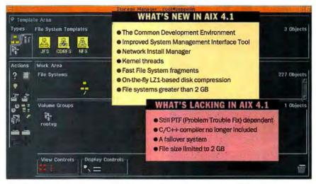
The VSM (Visual System Manager) is an extension of the CDE environment. VSM is a set of tools that lets you view installed products, hardware, and user accounts using an "object oriented" visual metaphor. The storage manager tool shown enables easy control of logical volumes, volume groups, and file systems.
