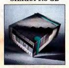
The Sierra 1.3 GB is the industry's fastest optical drive. It can be used as both a hard disk replacement and an on-line archiving system. Each 5.25" cartridge holds 1.3 Gigabytes of data, and boasts a 30-year shelf life. It is ideal for data-intensive applications such as graphics, CAD/CAM, multimedia or data archiving. \$2,495
