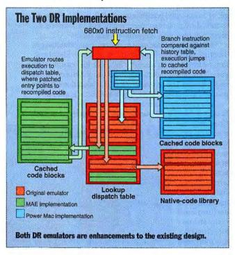
tected, recompiled, and the corresponding locations in the dispatch table and the application are revised, the interpretive emulator starts jumping to the recompiled code blocks (see the figure above, "The Two DR Implementations").
