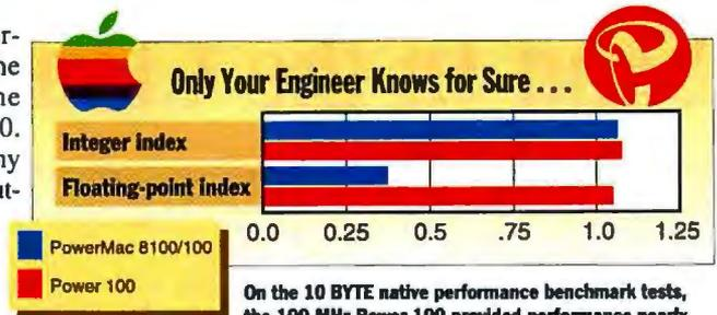
On the 10 BYTE native performance benchmark tests, the 100-MHz Power 100 provided performance nearly identical to that of a 100-MHz Power Mac 8100/100. On two tests, the Power 100 showed faster floating-point performance—due to the improved math library in System 7.5.1, not to system differences. Here we show just the integer and floating-point indexes derived from the 10 tests. Results are indexed; higher numbers indicate better performance, and a Dell 90-MHz Pentium = 1.
