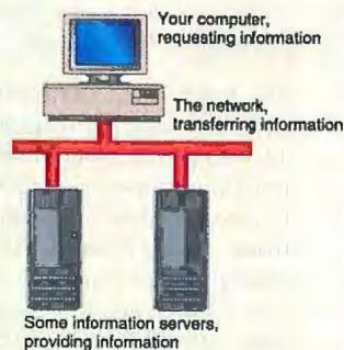
A fully functional WWW site requires a computer (with software), a set of network links, and servers.
