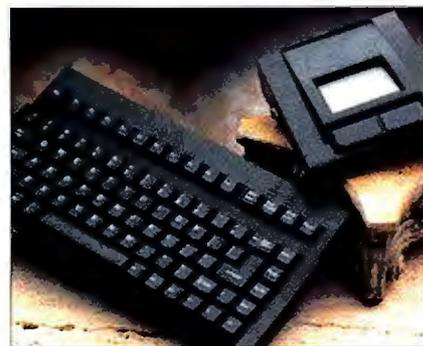
83-key keyboard, a mouse touchpad pointing device, and an RF transmitter/receiver. The touchpad allows fast and accurate movement of the screen cursor as you simply glide your finger over its 2- by 3-inch surface.
