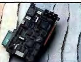
**KS-1** XT CPU card. NEC V40, 1 MB Dram, Sram, Flash, Pcmcia, 3 srl, 2 par, modem, A/D. **\$129 up**
