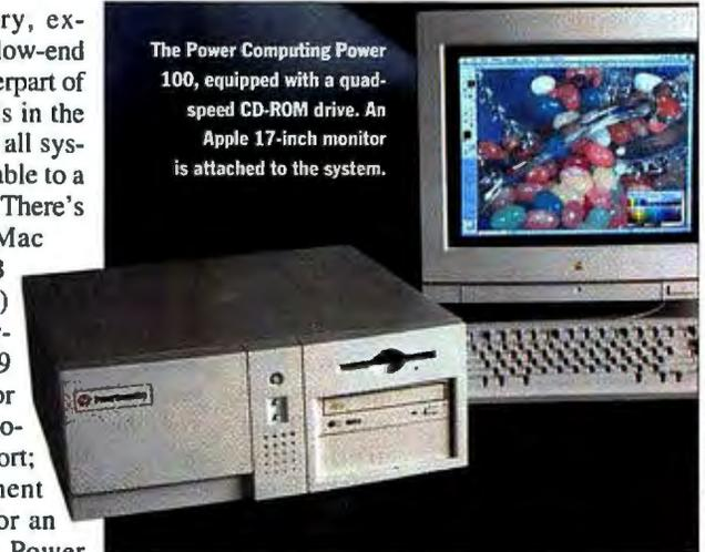
The Power Computing Power 100, equipped with a quad-speed CD-ROM drive. An Apple 17-inch monitor is attached to the system.
