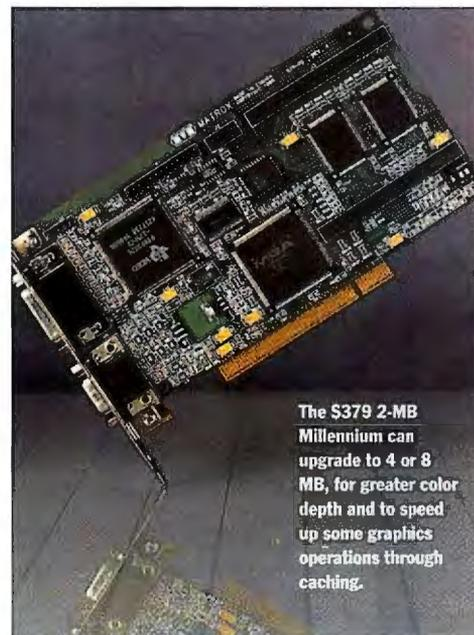
The \$379 2-MB Millennium can upgrade to 4 or 8 MB, for greater color depth and to speed up some graphics operations through caching.
