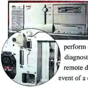
The SFT Alpha has a swinging door on the front of the chassis that prevents you from inadvertently turning off or resetting the system. It also includes a removable SCSI hard drive that's protected with a keylock. The large tower chassis is mounted on four rollers, enhancing the file server's mobility.
