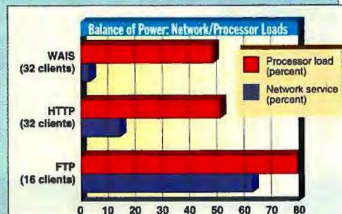
Under heavy FTP activity, the server's work is balanced between network-servicing and processing chores. But as the server tends to HTTP and WAIS activity, the processor becomes the chief performance constraint.
