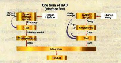
With RAD (rapid application development), you design and prototype the interface separately from designing and programming the rest of the system. This enables you to have two groups of engineers working in parallel and mostly independently, if you change the interface (which in traditional programming would necessitate reprogramming—possibly severely), you can simply relink it with the back-end code. It may not even require any reworking of the systems design.
