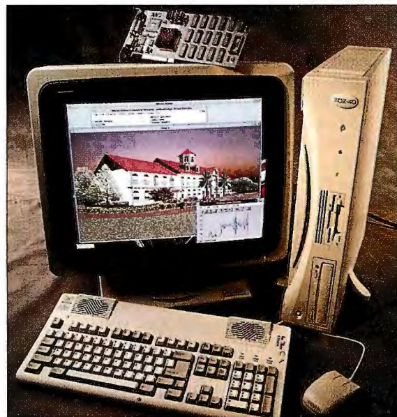
Intergraph's Pentium-powered TDZ-40 system combines workstation-level 3-D performance with Intel x86 software compatibility. The Omnicomp 3Demon SX48 board (perched atop the monitor) provides good 3-D performance for tighter budgets.
