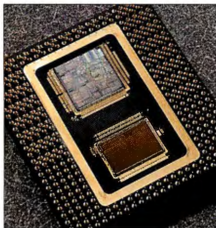
THIS IS INTEL'S P6: ALL 5.5 MILLION TRANSISTORS, 133 MHz, AND 300 MIPS OF IT. IT'S ROUGHLY 6000 TIMES AS FAST AS THE 4004. YOU'VE COME A LONG WAY, x86.
