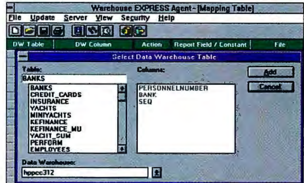
Software AG's SourcePoint Administrator lets a user select a table from the warehouse and map columns to fields from the extract process.
