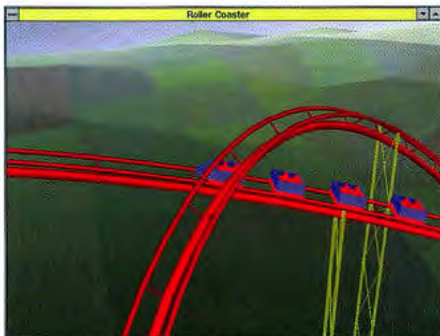
The GLINT displaying a 3-D object with fogging, which enhances the illusion of depth.
