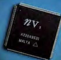
doesn't need on-board memory to hold wave sounds—it can store them in main memory. The one potential problem with the NV1's DSP is that its algorithms are hard-wired into its silicon, so upgrades could be difficult. It's a gamble that reduces the cost and size of the NV1 overall.
