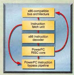
Based on information obtained from sources close to IBM, this speculative design for a Pentium-pin-out PowerPC chip shows how a PowerPC core could be united with an x86-compatible bus. The dual-mode CPU would support both instruction sets, routing x86 instructions through a special decoder that converted the CISC instructions into native-RISC instructions.
