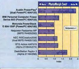
The BYTE cross-platform BYTEmark CPU test shows the PowerPC 604 favorably compared to other CPUs. The Austin PowerPlay<sup>2</sup> 604/133 trailed the 133-MHz IBM Power Series 850 just slightly, due to the overhead of managing two CPUs. Two processors gave the PowerPlay<sup>2</sup> a strong advantage in the PhotoMorph Swiri test, but not in the MicroStation CAD test (results not shown), where graphics controllers are a big factor.
