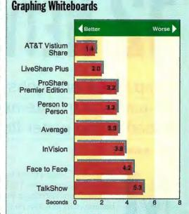
AT&T Vistium Share was the fastest program at updating a graph displayed on the whiteboard. This test used uncompressed files to measure network performance only (factoring out file loading, format conversion, establishing the network link, and so forth).
