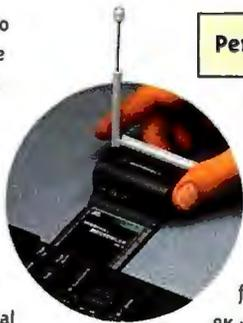
Wireless Modem Card slips into most laptops, palmtops or PDAs with a Type II or III PCMCIA slot. This all-in-one peripheral features a built-in battery for stand alone operation, 8K message memory and fold-away antenna.
