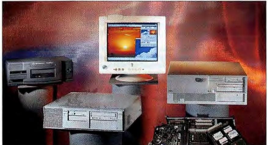
Two PowerPC 604 workstations and a server (from left to right): Motorola's PowerStack Series E 604-100P server, Austin Direct's PowerPlay<sup>2</sup> 604/133, and IBM's Power Series 850.
