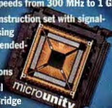
tains five files of 64-bit registers, with 64 registers per file. It also has 64 KB of on-board cache memory, equally divided between instructions and data. A dedicated I/O bus that's only 8 bits wide but can transfer 1 GB of data per second connects the Mediaprocessor to the MediaCodec and MediaBridge.
