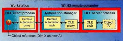
Remote Automation works by replacing the original proxy and stub with modules that use the remote procedure call (RPC) protocol to communicate over the network.
